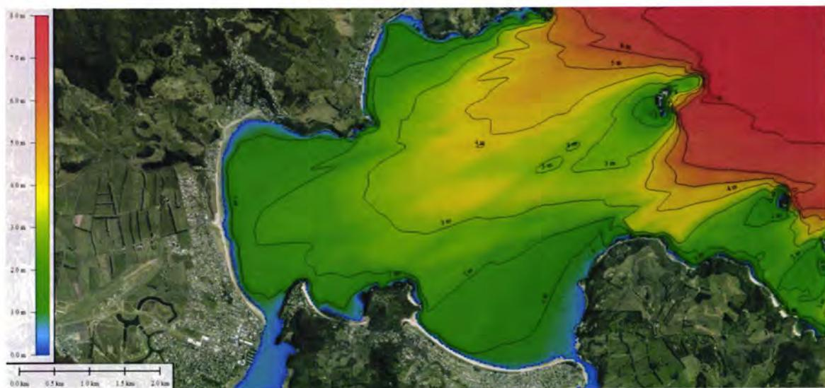
The SWAN model predicts a nearshore wave height of 2.15 m at the 5 m depth contour offshore of Buffalo Beach for a 1% AEP easterly event. Wave set up has been assessed based on the methods described within the Coastal Engineering Manual (CEM, 2006), with the resulting estimated wave set-up being 0.6m.
