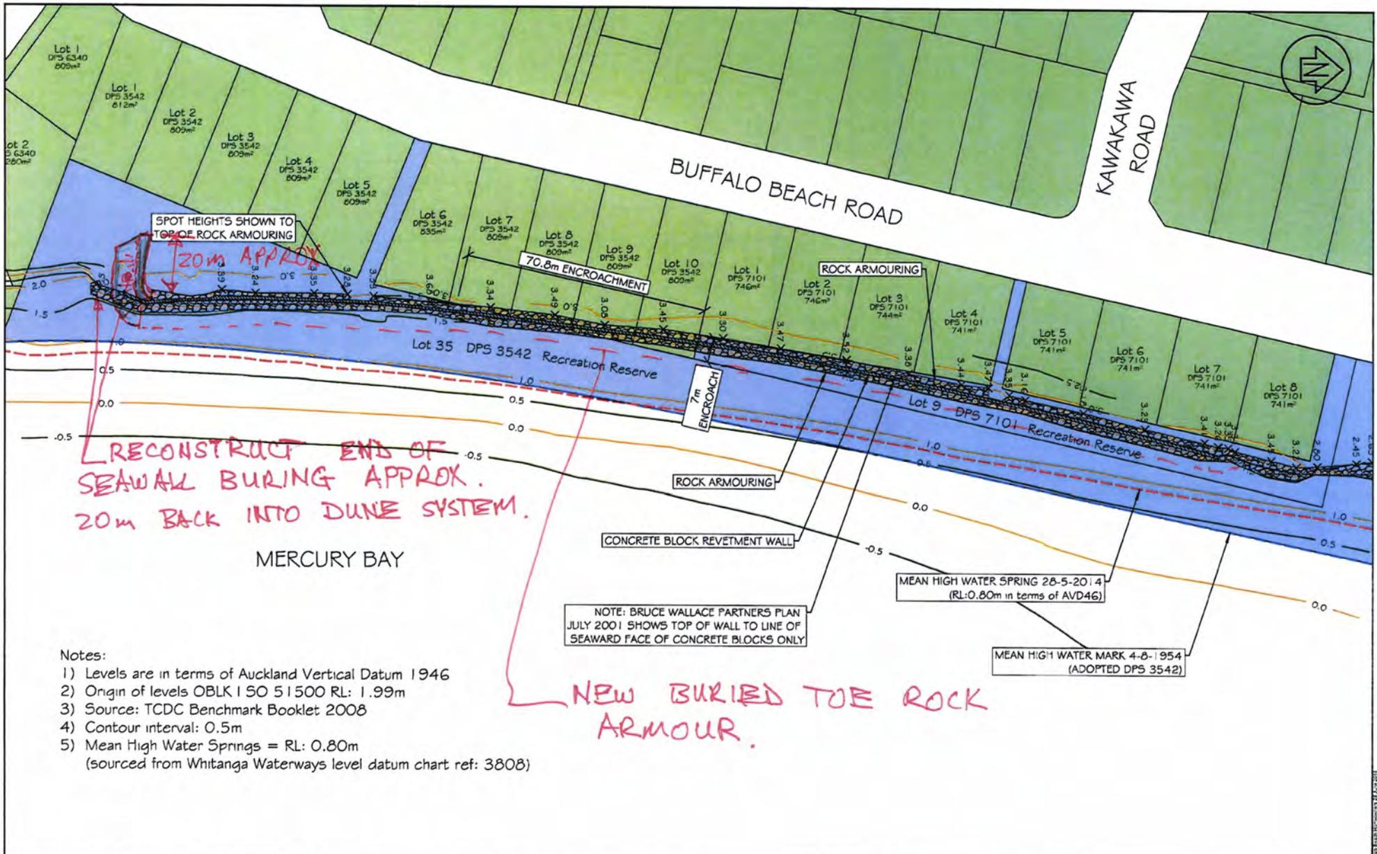
RECONSTRUCT END OF SEAWALL BURING APPROX. 20m BACK INTO DUNE SYSTEM.
