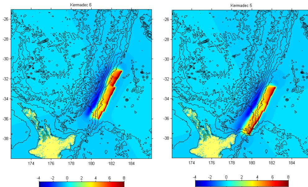
**Figure 2.2 Cases 5 and 6: 600 x 100 km fault, 20.9 m average slip,  $M = 9.1$**
