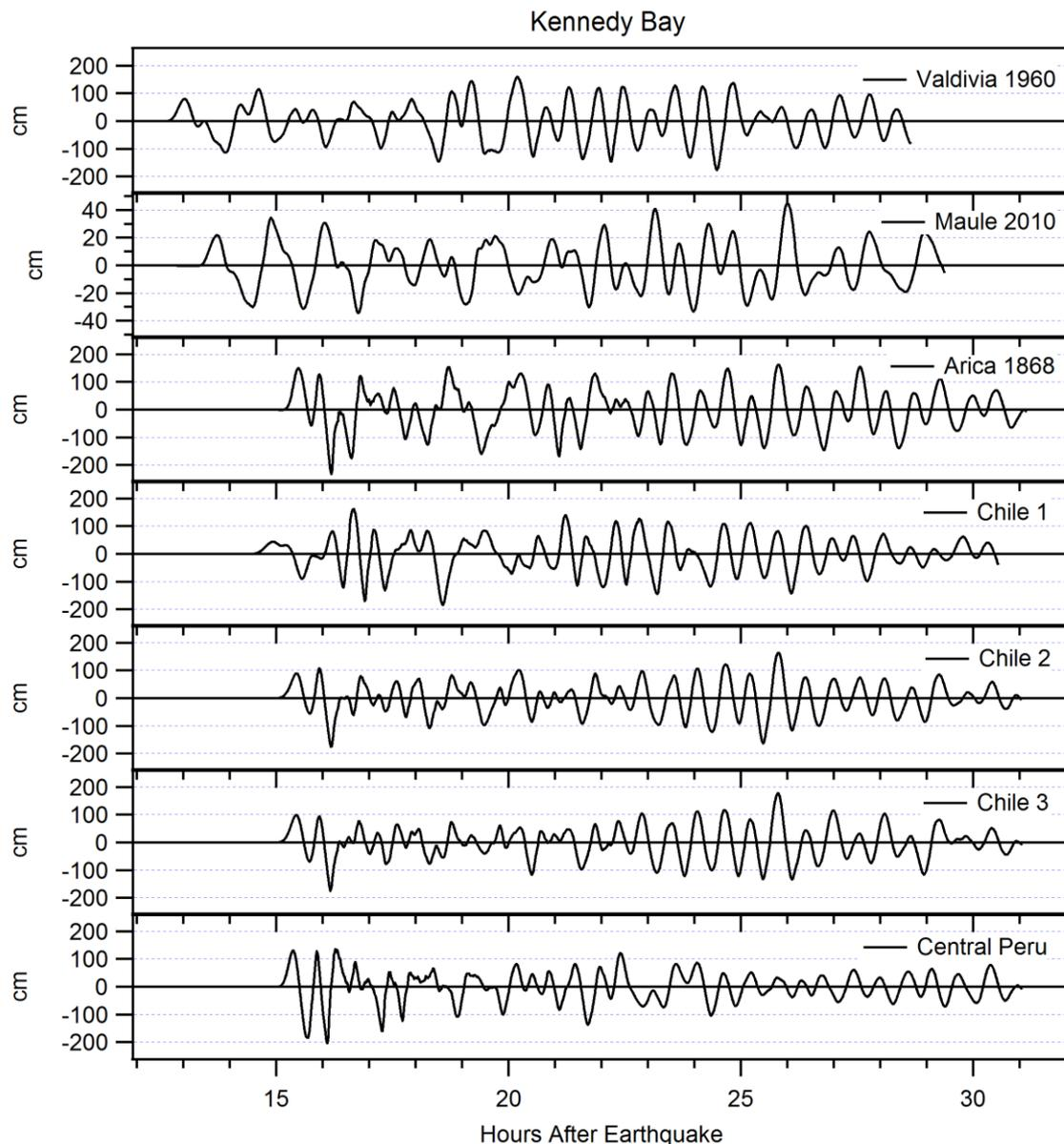
**Figure 4.3 Modelled time series of water levels in Kennedy Bay for each of the distant source scenarios. Note the different scale for the Chile 2010 case.**
