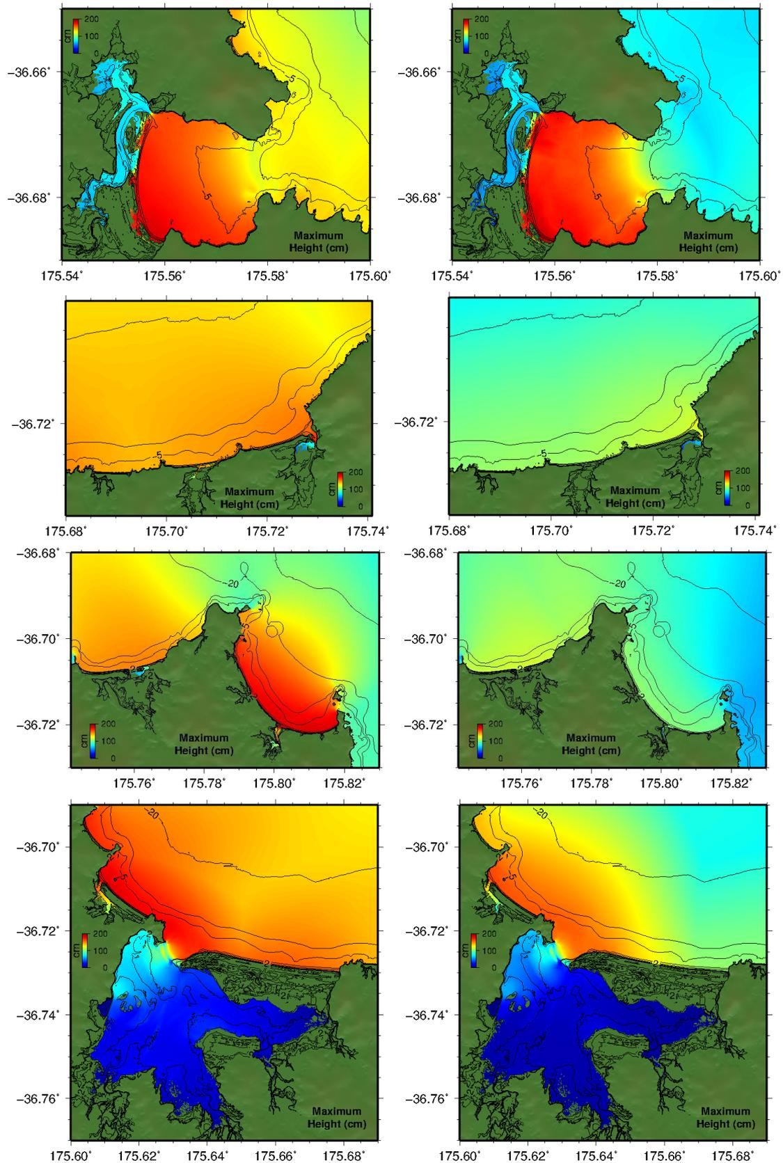
**Figure 4.8 Modelled tsunami heights from the 1868 Arica scenario (left) and the Chile North 1 scenario (right) for Kennedy Bay, Whangapoua, Kuaotunu and Opito Bay (top to bottom); each case run at HT.**
