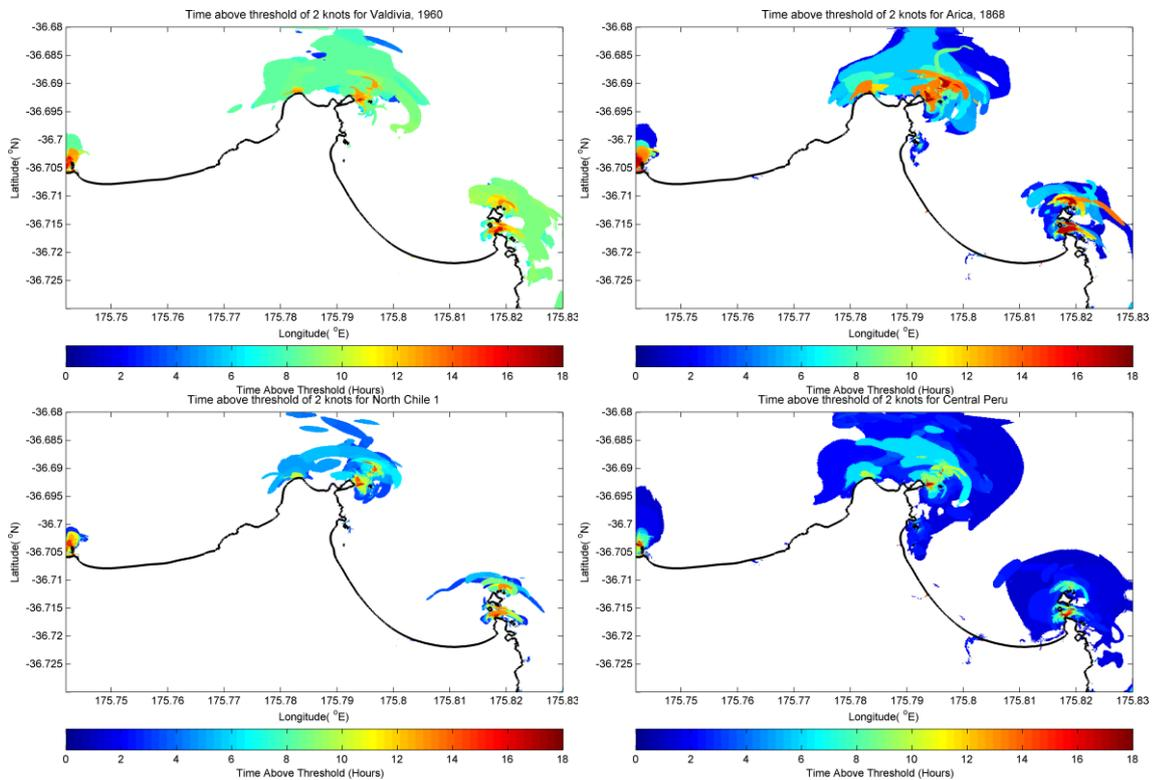
**Figure 4.13 Time Current threshold maps for current speeds of 2 knots for the Chile 1960 (top left) Arica 1868 (top right), Chile North 1 (bottom left) and Central Peru (bottom right) at High tide in Opito Bay.**
