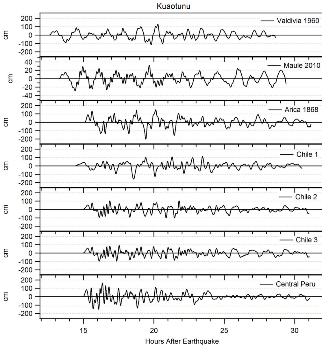
**Figure 4.4 Modelled time series of water level at Kuaotunu for each of the distant source scenarios. Note the different scale for the Chile 2010 case.**
