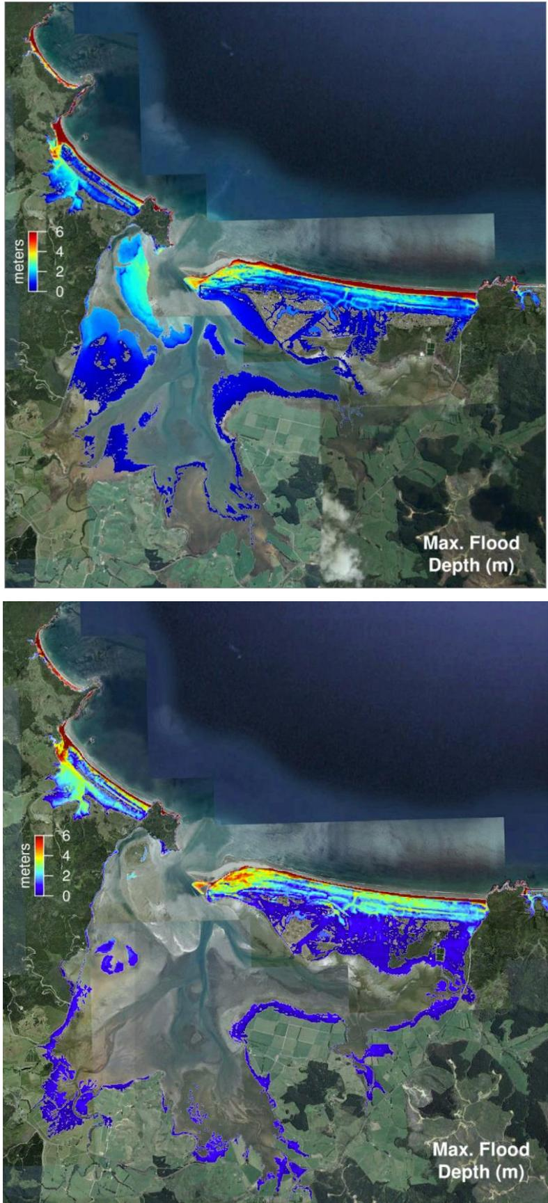
Figure 3.11 Maximum computed tsunami flood depths above ground level at Whangapoua for scenario TK 8 MSL (top) and TK 8 HT (bottom).
