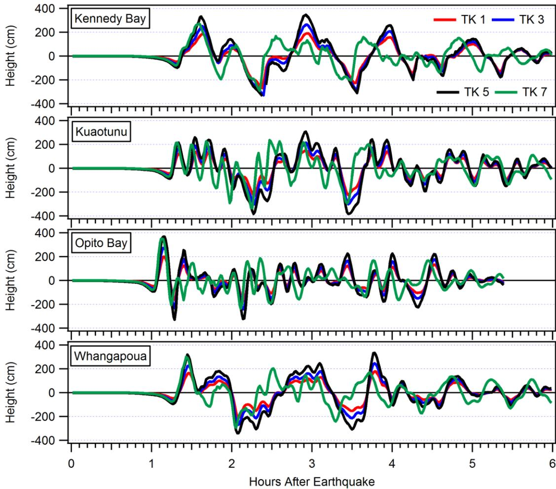
**Figure 3.1 Water level time series plots for sources 1, 3, 5 and 7 at the four sites. Time series locations are indicated with the red dot in Figure 1.4.**
