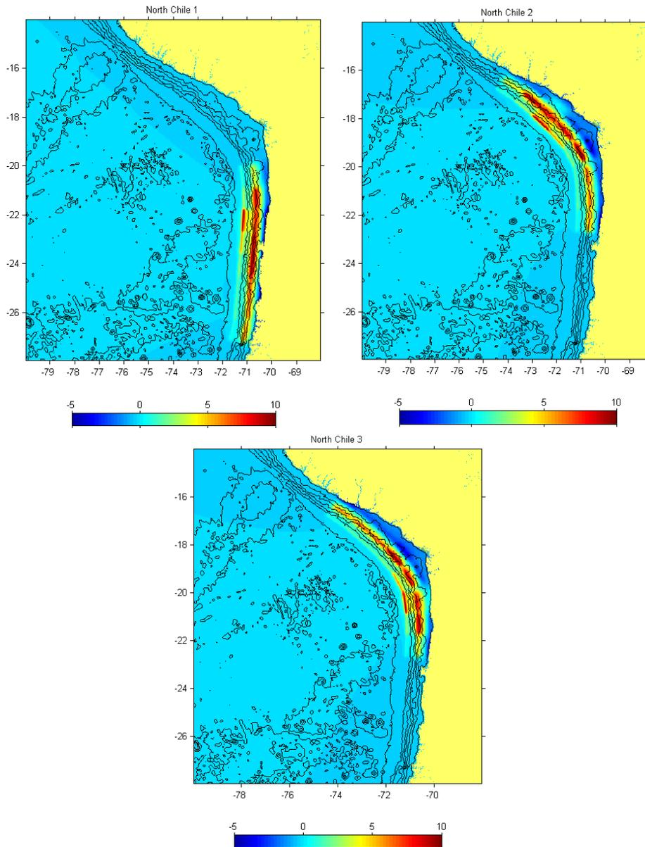
**Figure 2.8 Three additional South American sources. Variants of the Fujii and Satake (2012) source for the 1960 Chile earthquake are positioned along the coast of Northern Chile and Southern Peru.**
