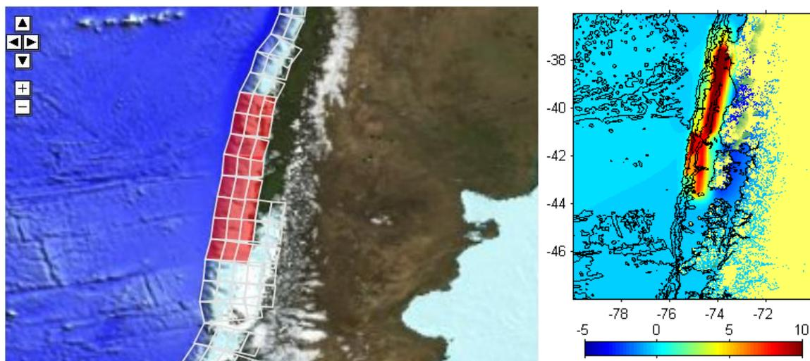
**Figure 2.4 (left) Unit source segments used to define the 1960 Chilean Earthquake suite of events. (right) initial sea floor deformation at the source region.**
