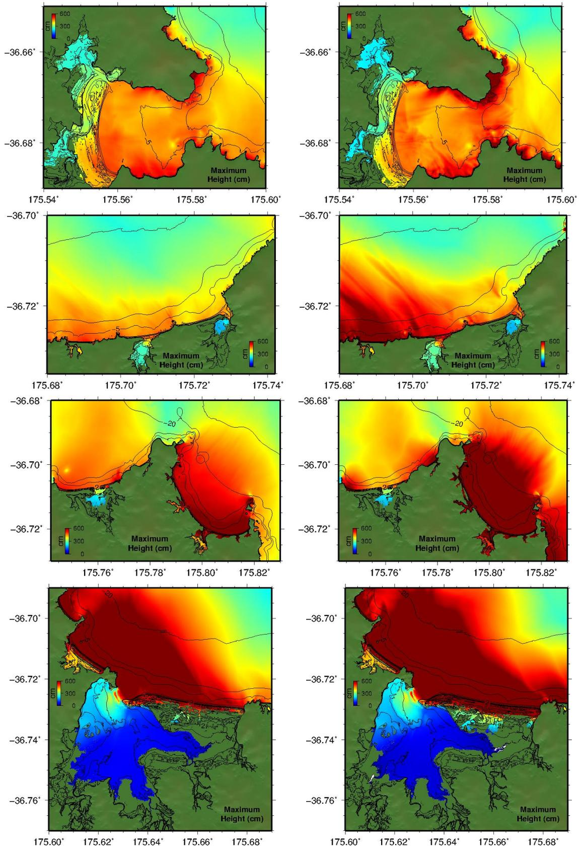
**Figure 3.6 Maximum computed tsunami heights above model reference water level for scenarios TK 6 (left) and TK 8 (right) at Kennedy Bay, Whangapoua, Kuaotunu and Opito Bay (top to bottom respectively); each case run at MSL.**
