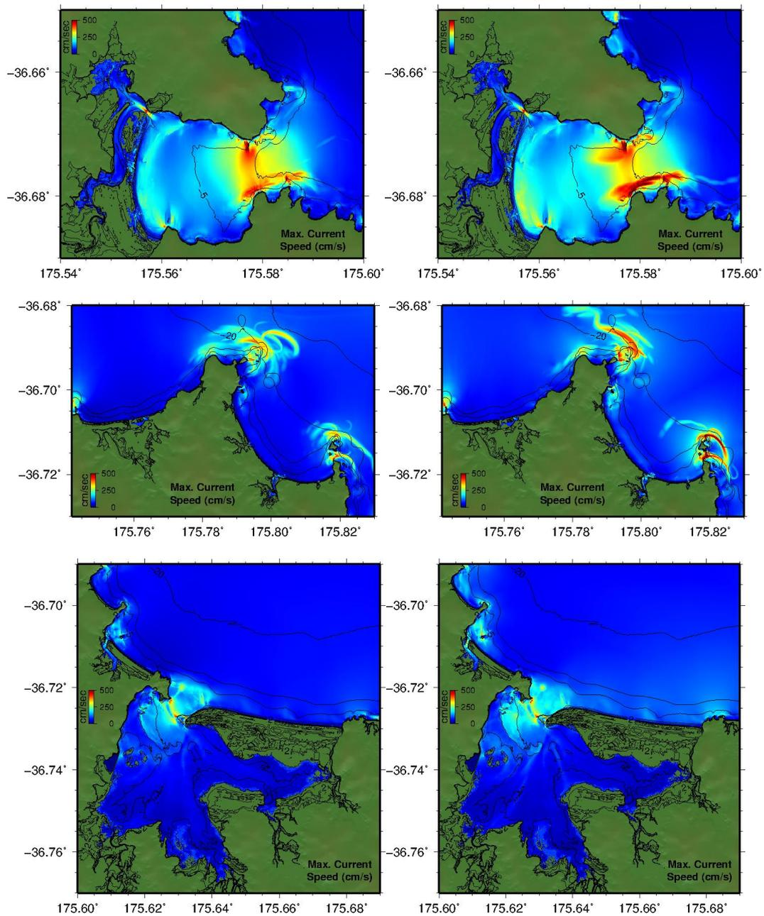
**Figure 4.10** Maximum modelled current speeds from the Arica 1868 (left) and Central Peru (right) scenarios for Kennedy Bay, Whangapoua and Opito Bay (top to bottom respectively); each case run at HT.
