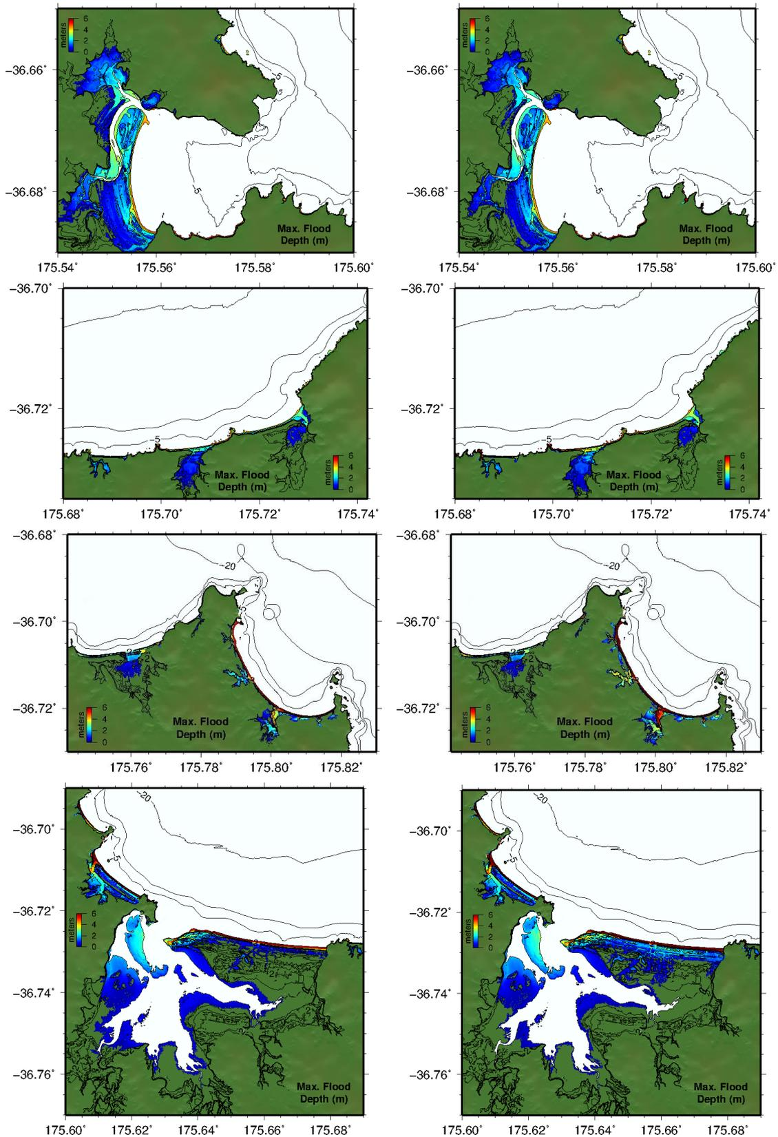
**Figure 3.7 Maximum computed tsunami flood depths above ground level for scenarios TK 6 (left) and TK 8 (right) at Kennedy Bay, Whangapoua, Kuaotunu and Opito Bay (top to bottom respectively); each case run at MSL.**
