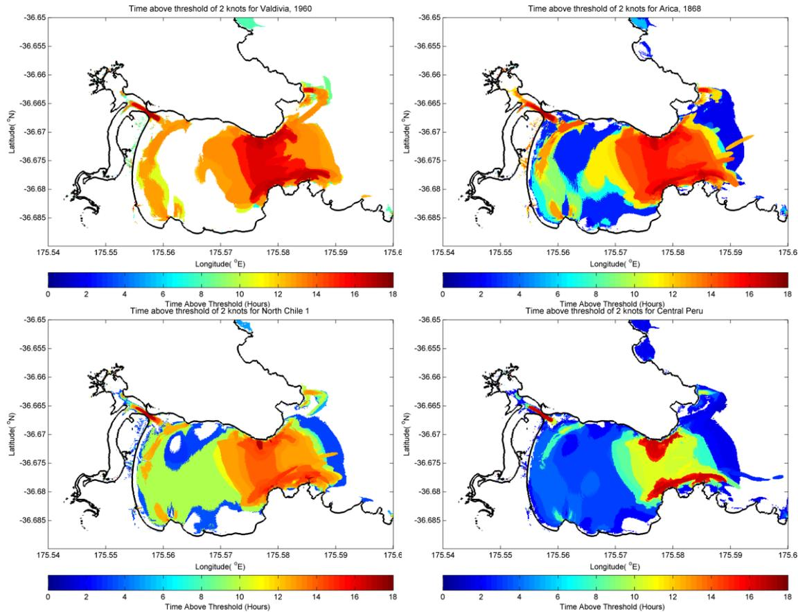
**Figure 4.11 Time Current threshold maps for current speeds of 2 knots for the Chile 1960 (top left) Arica 1868 (top right), Chile North 1 (bottom left) and Central Peru (bottom right) at High tide in Kennedy Bay.**
