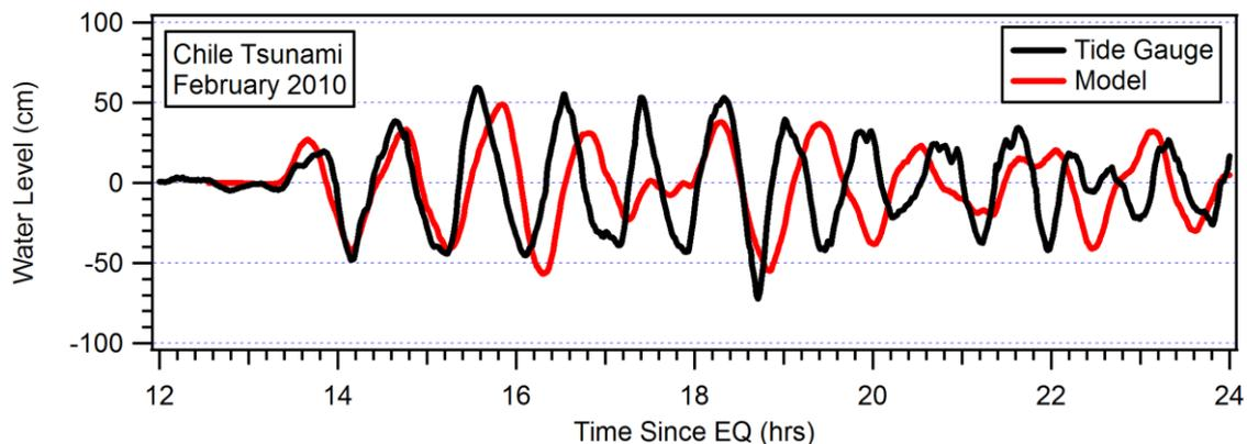
**Figure 2.6 Comparison between measured and modelled water levels at the Whitianga tide gauge for the February 2010 Chile earthquake and tsunami.**
