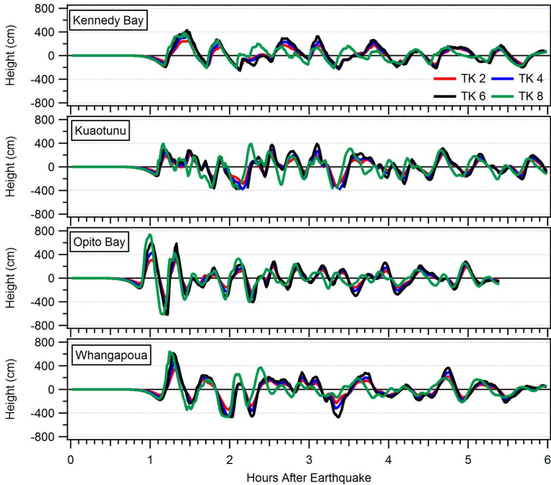
**Figure 3.2 Water level time series plots for sources 2, 4, 6, and 8 at the four sites. Time series locations are indicated with the red dot in Figure 1.4.**
