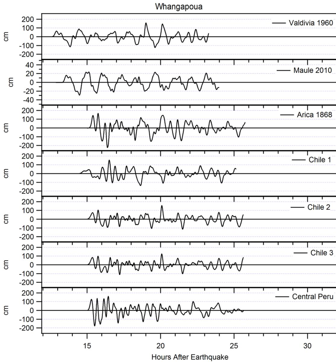
**Figure 4.6 Modelled time series of water levels at Whangapoua for each of the distant source scenarios. Note the different scale for the Chile 2010 case.**
