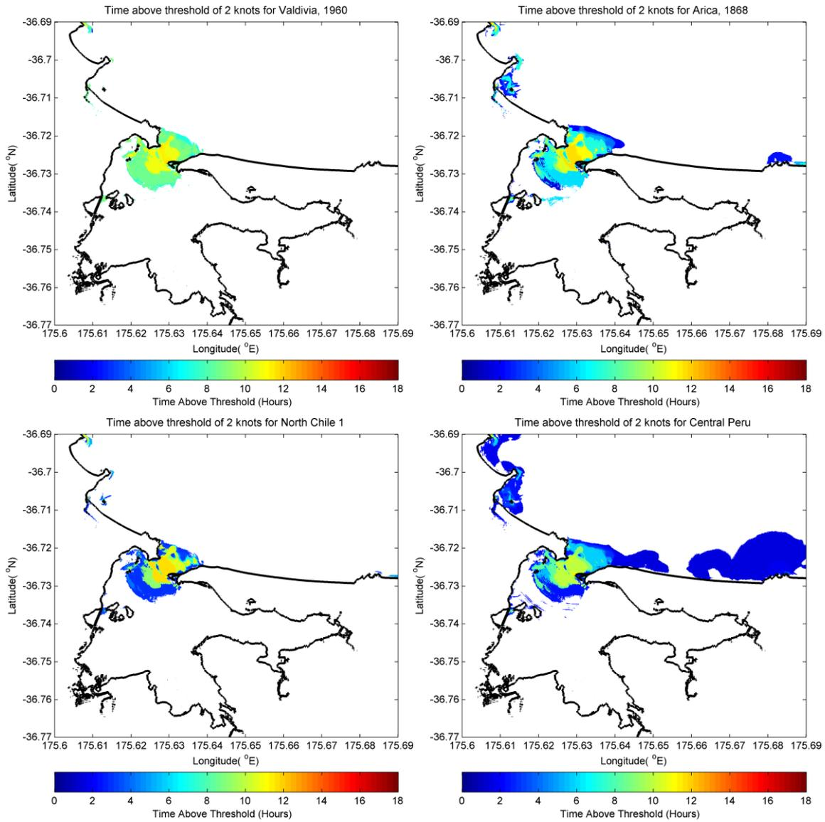
**Figure 4.14 Time Current threshold maps for current speeds of 2 for the Chile 1960 (top left) Arica 1868 (top right), Chile North 1 (bottom left) and Central Peru (bottom right) at High tide in Whangapoua.**
