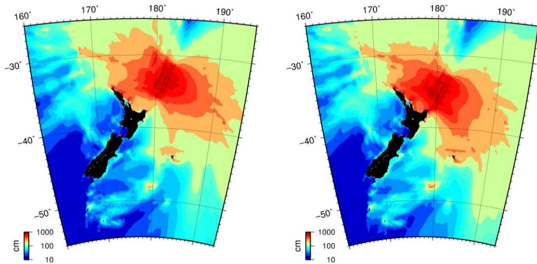
**Figure 3.4** Maximum computed tsunami heights over the regional grid for source TK 1 (left) and TK 2 (right). Tsunami heights along the Coromandel Peninsula and in the Bay of Plenty are noticeably higher from source TK 2 due to its more southerly position along the subduction zone.
