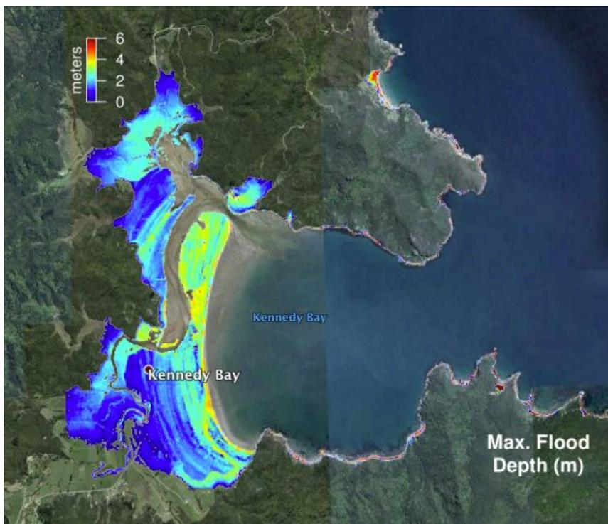
Figure 3.8 Maximum computed tsunami flood depths above ground level at Kennedy Bay for scenario TK 8 MSL (top) and TK 8 HT (bottom).
