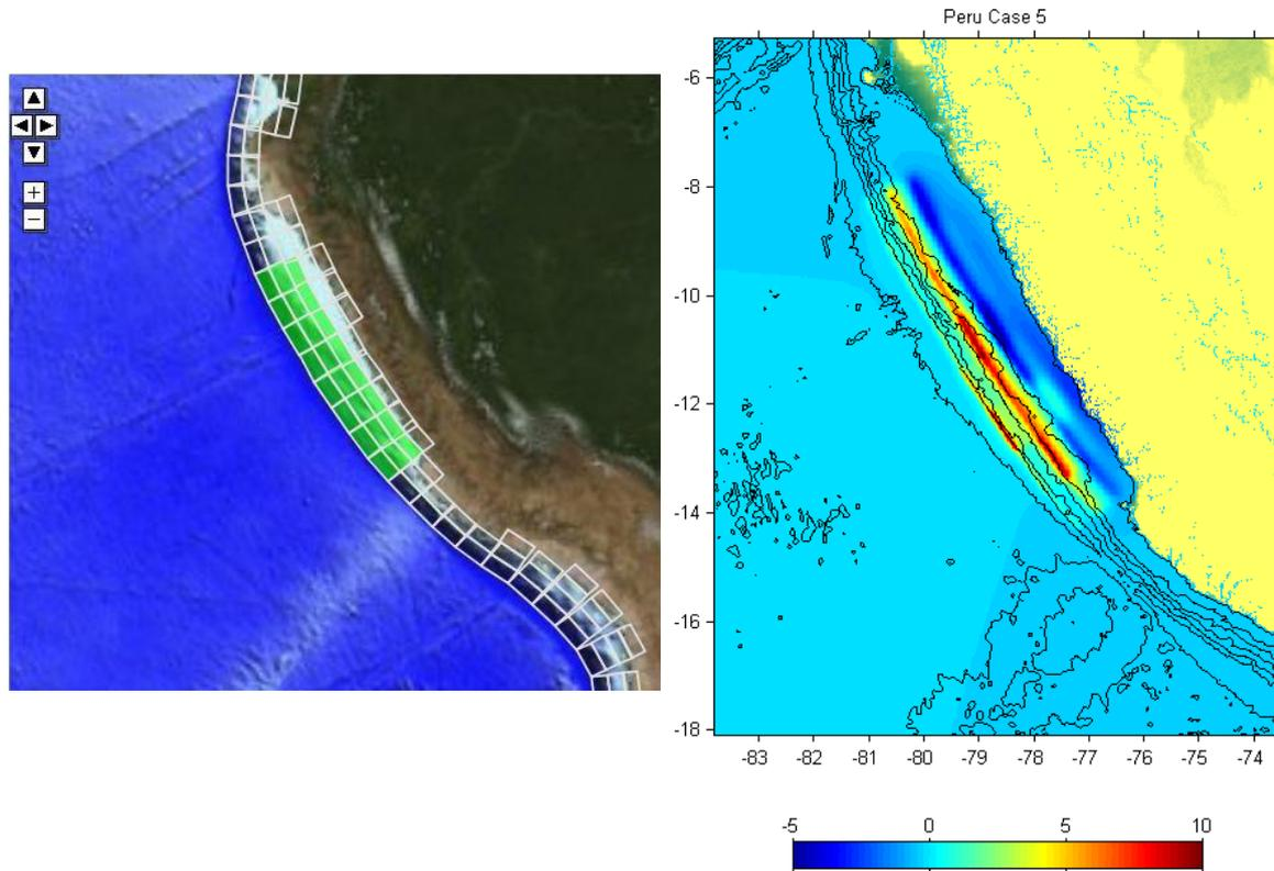
**Figure 2.9** Fault segments used to construct the Peru tsunami source (left) and the initial deformation field used to initialise the tsunami model (right).
