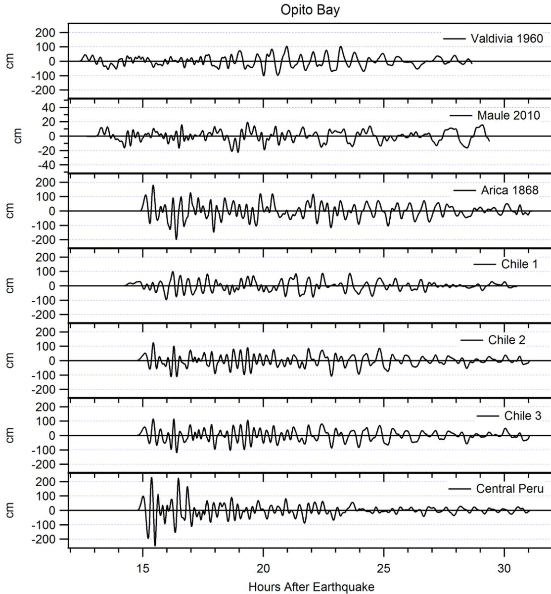
**Figure 4.5 Modelled time series of water levels in Opito Bay for each of the distant source scenarios. Note the different scale for the Chile 2010 case.**
