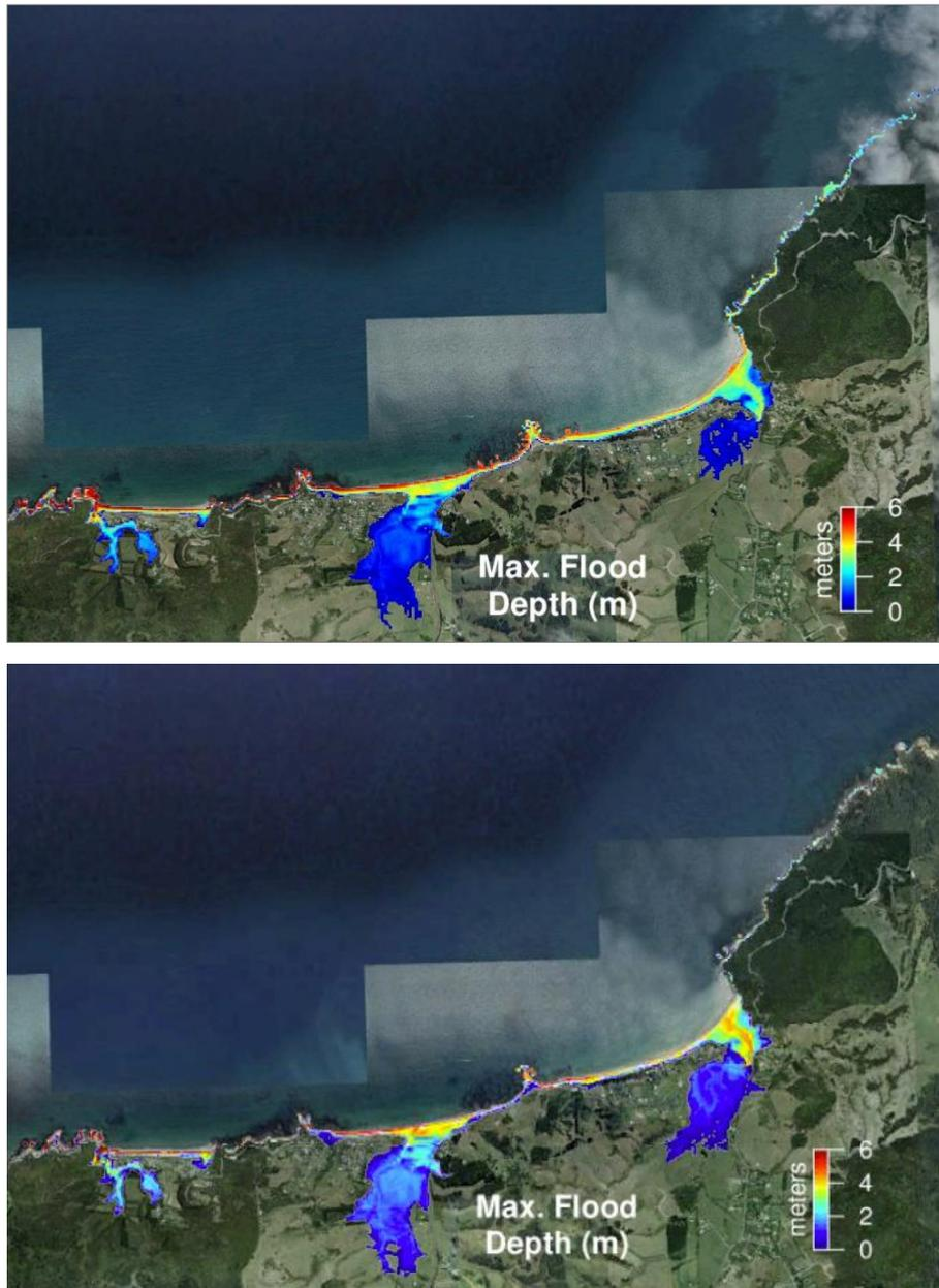
**Figure 3.9 Maximum computed tsunami flood depths above ground level at Kuaotunu for scenario TK 8 MSL (top) and TK 8 HT (bottom).**
