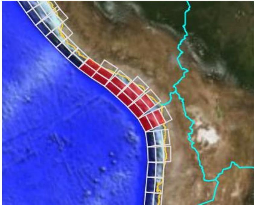
**Figure 2.7 Source segments used to model the 1868 Arica tsunami. A uniform slip amount of 39.6 m was applied to each segment.**
