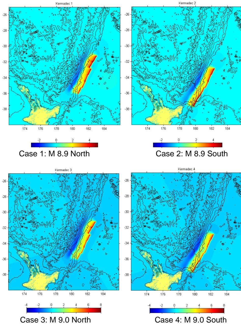
**Figure 2.1 Case 1, 2: 600 x 100 km fault 10.47 m average slip, M = 8.9. Case 3, 4: 600 x 100 km fault, 14.8 m average slip, M = 9. Note the change in the colour scale for cases 3 and 4.**
