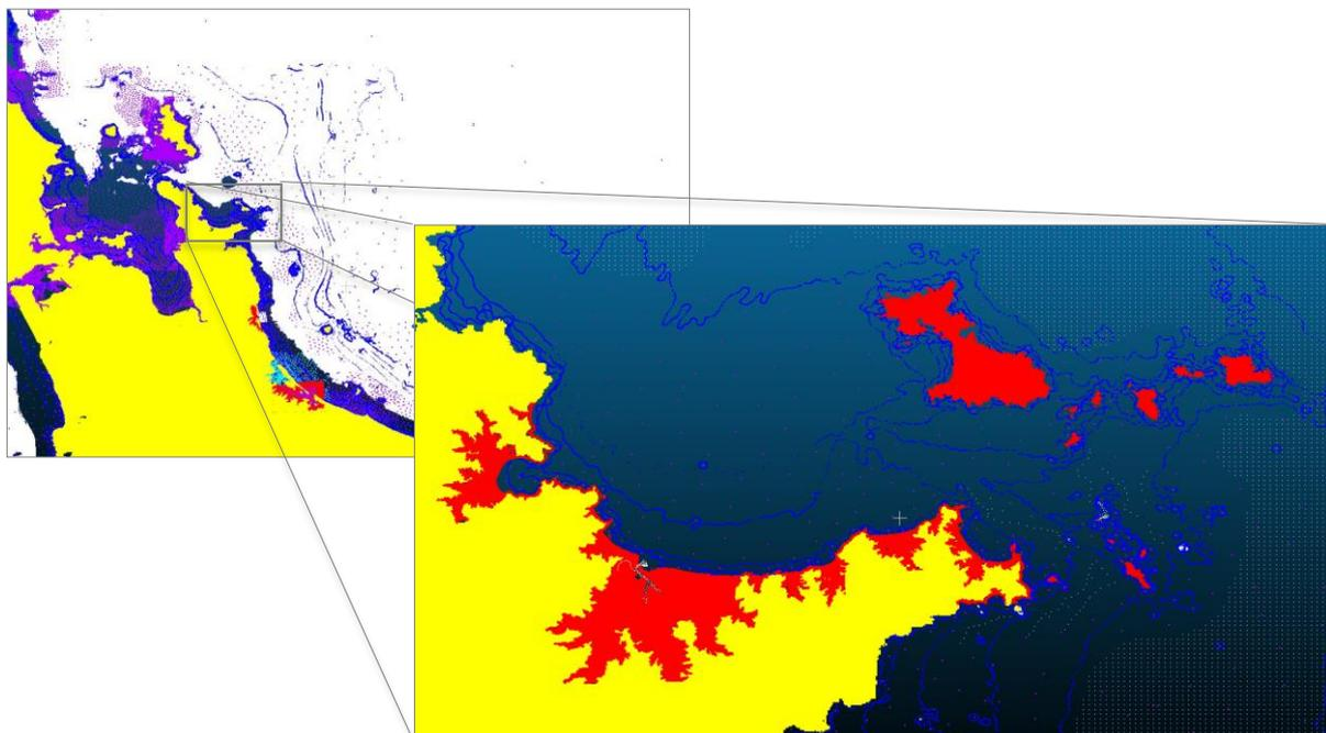
**Figure 1.3 (left) coverage area of the different bathymetry data sets. Yellow: SRTM topography, White: NIWA bathymetry, Blue and Purple: LINZ digitised charts contours and sounding points. (right) Close-up of the Kennedy Bay/Whangapoua/Kuaotunu/Opito Bay region, yellow: SRTM topography, Red: LiDAR topography, Blue: LINZ digitized contours and soundings.**
