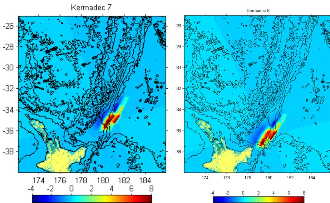
**Figure 2.3 Case 7 (left) the Japan 2011 tsunami source positioned 200 km north of the East Cape ( $M = 8.8$ ). Case 8 (right) the Japan 2011 tsunami source positioned at the southern end of the Tonga-Kermadec Trench ( $M=8.8$ ).**
