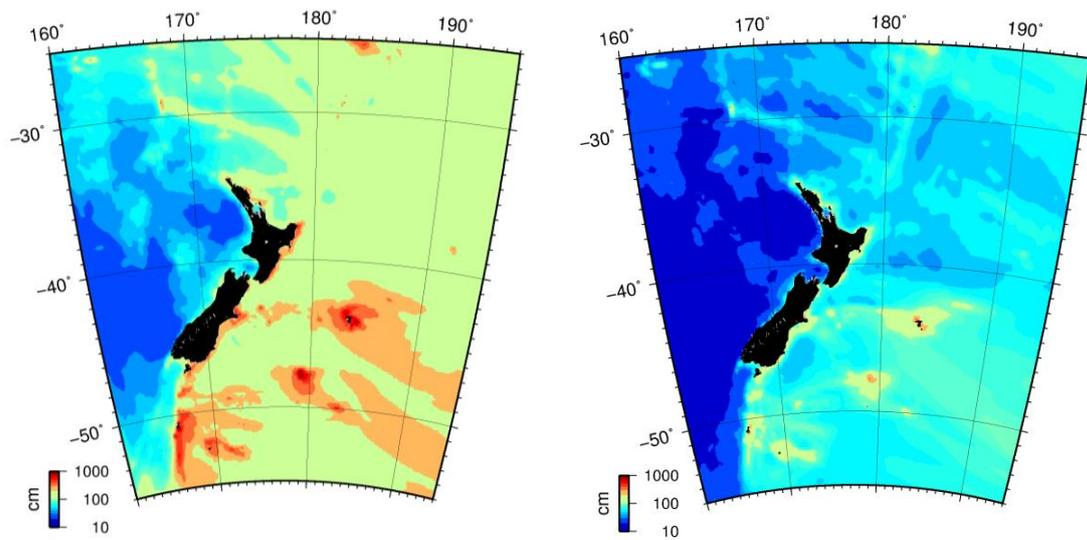
**Figure 4.9 Modelled tsunami heights from the propagation model for the 1868 Arica scenario (left) and the Chile North 1 scenario (right).**
