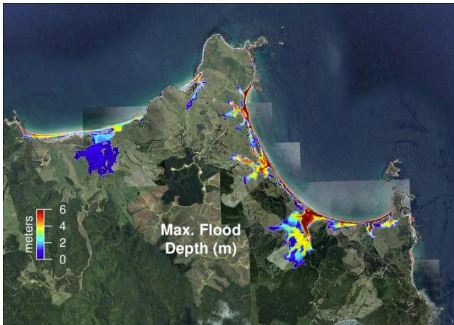
Figure 3.10 Maximum computed tsunami flood depths above ground level at Opito Bay for scenario TK 8 MSL (top) and TK 8 HT (bottom).
