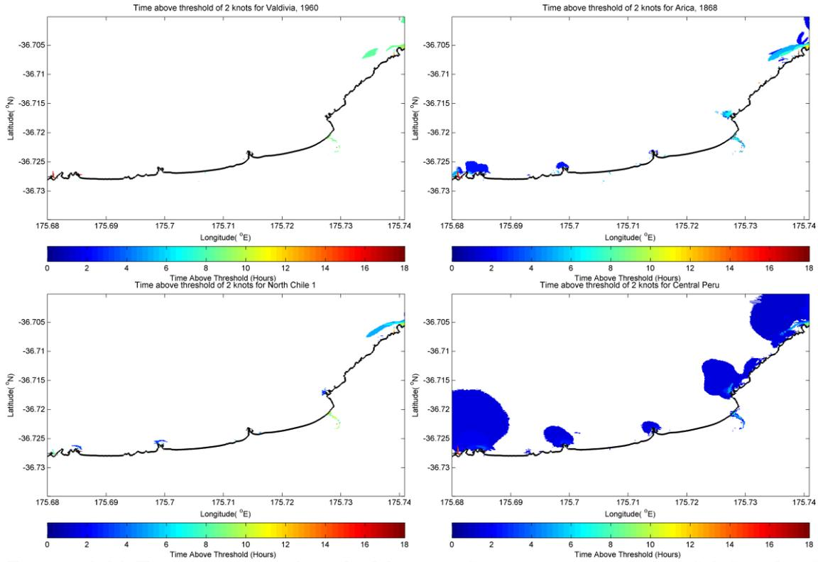
**Figure 4.12 Time Current threshold maps for current speeds of 2 for the Chile 1960 (top left) Arica 1868 (top right), Chile North 1 (bottom left) and Central Peru (bottom right) at High tide in Kuaotunu.**
