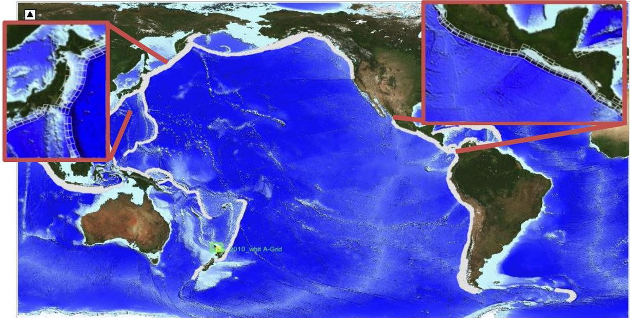
**Figure 1.2** The ComMIT propagation model database for tsunamis in the world's oceans. Insets show the details of the source zone discretization in to rectangular sub-faults.
