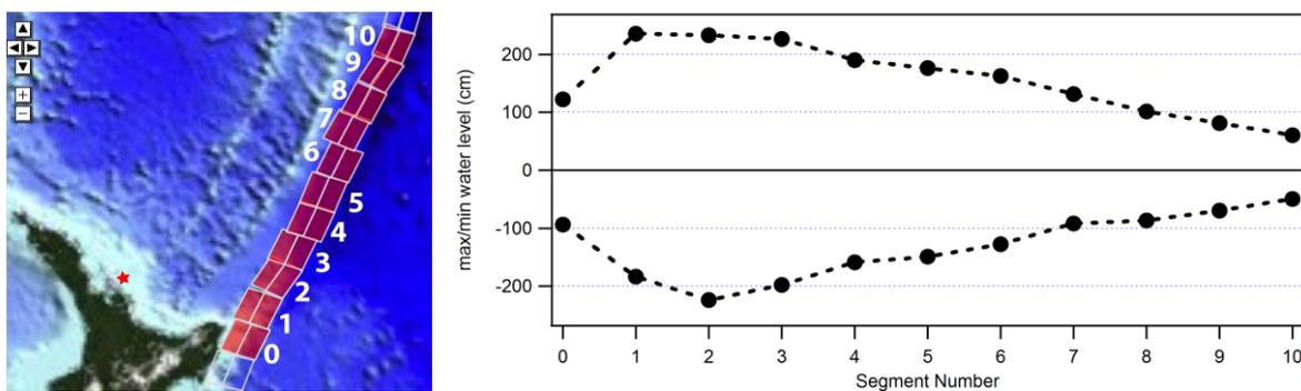
**Figure 3.3 Tsunami wave heights produced offshore of the Coromandel Peninsula (red star) by identical tsunami sources positioned on each of the fault segments indicated in the panel on the left. Note that the strongest effects are the result of ruptures in the first 300 km north of the East Cape (segments 1, 2 and 3).**
