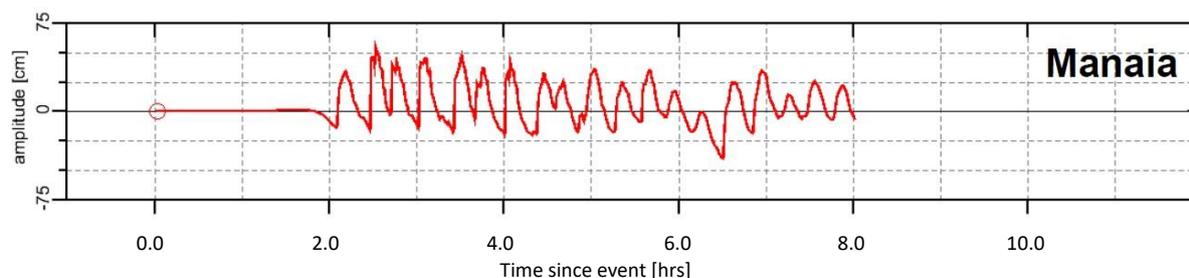
Figure 7: Wave arrival times and inundation levels from the Tonga-Kermadec Trench (at MHWS)
