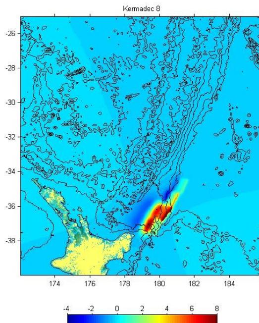
Figure 6: The 'maximum credible event' from the Tonga-Kermadec Trench. This event is a similar magnitude and nature to the 2011 Japan tsunami
