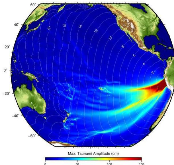
**Figure 11: Map of the 'FF 7' variant of the 1960 Chilean earthquake, placed in Central Peru**
