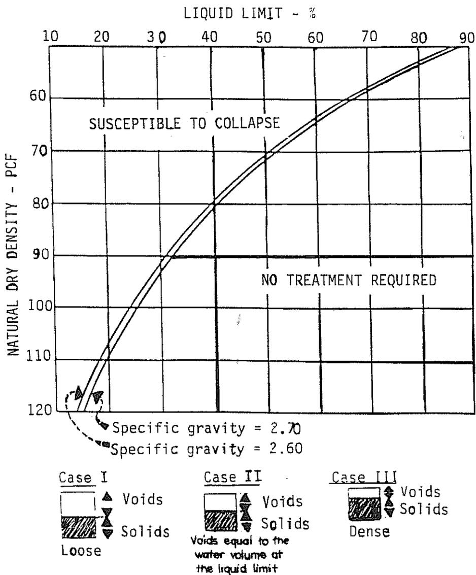
Figure 3:0. Alternate foundation design criteria for relatively dry fine grained soils
