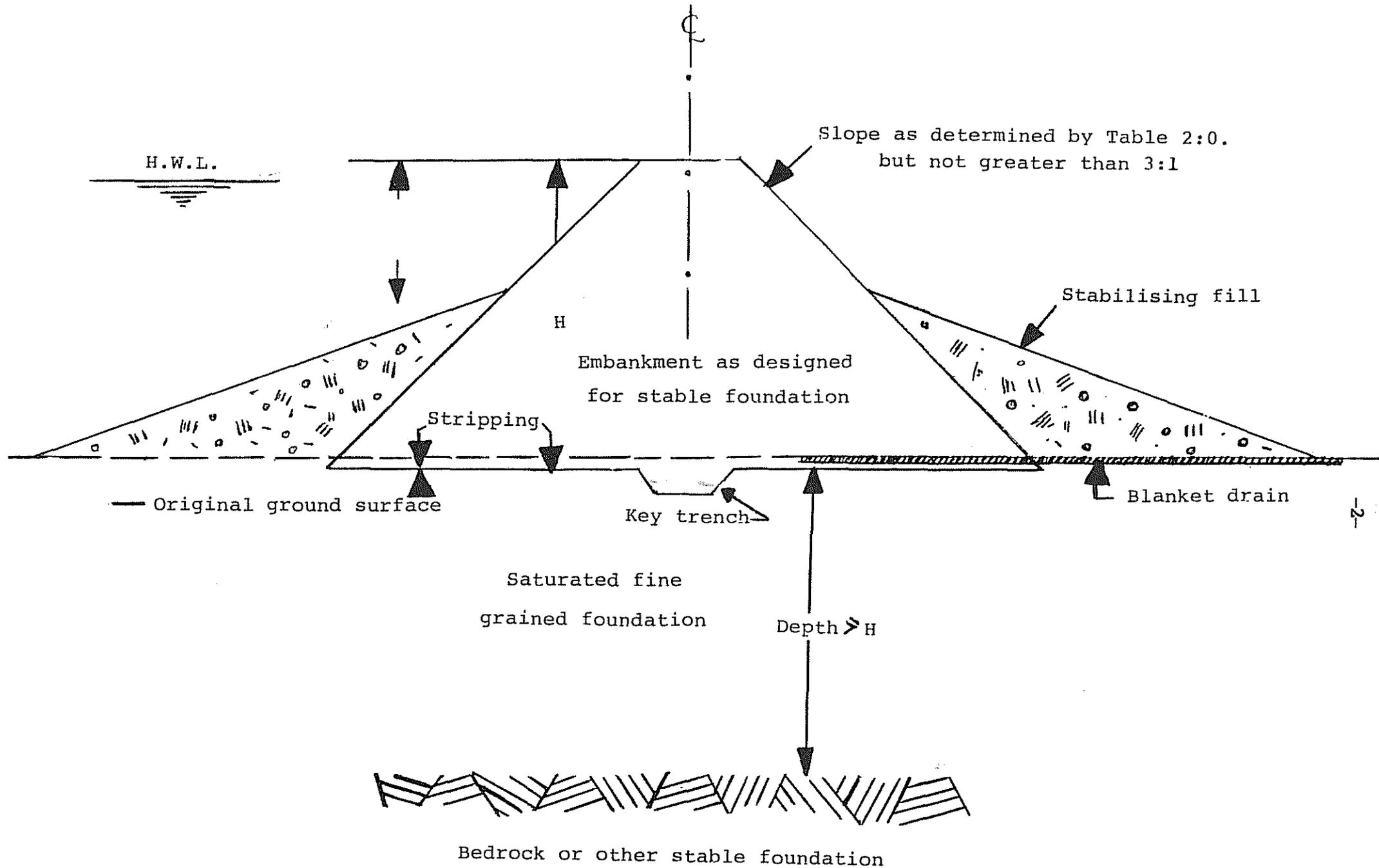
Figure 1:0. Design of dam on saturated fine grained foundation
