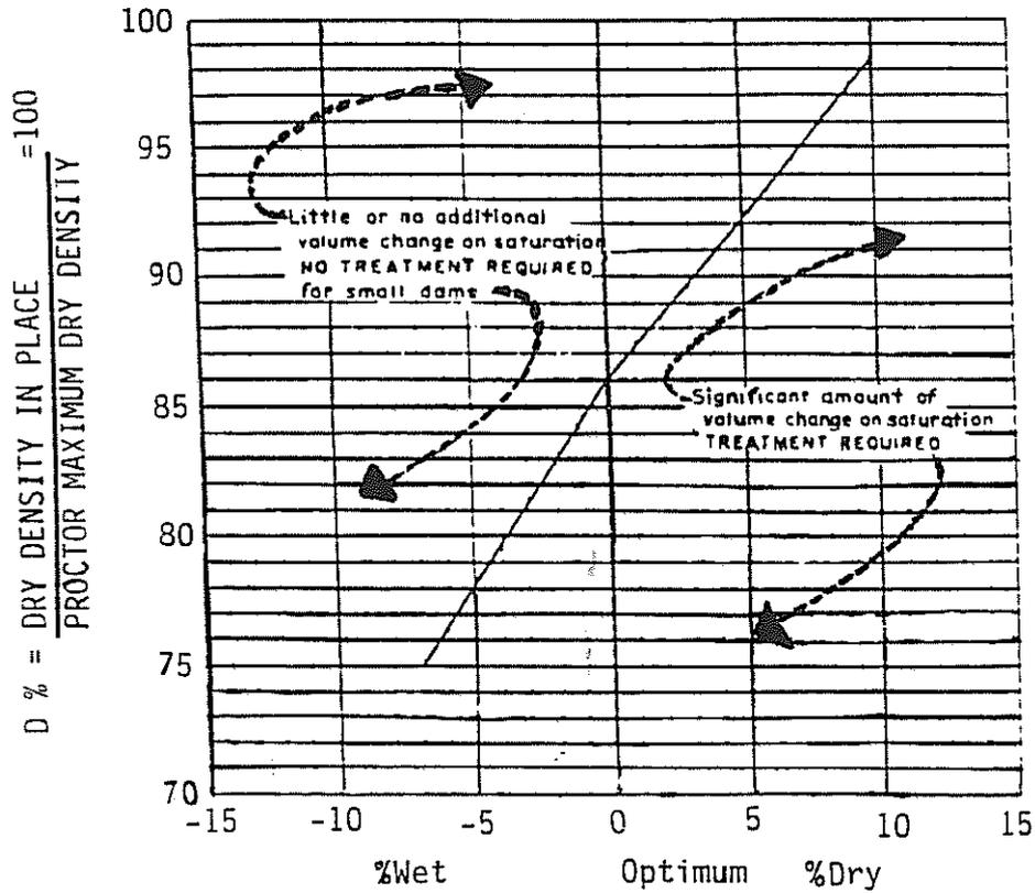
Figure 2:0. Foundation design criteria for relatively dry finegrained soils
