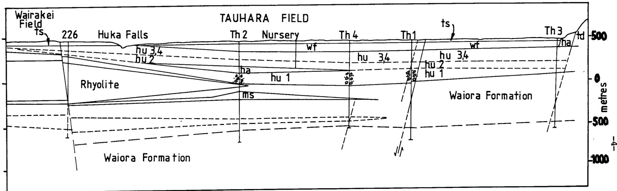
FIGURE 2: NW-SE simplified geological cross section through Tauhara Geothermal Field. Data from Grindley, 1965 and Grindley, et al., 1966. Vertical and horizontal scales are equal.
