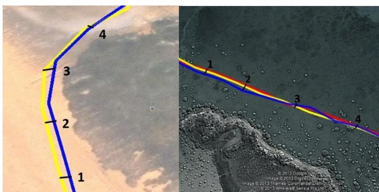
**Figure 3-1: Examples of precision measurements for Manaia (left) and Whangapoua (right) harbours.** In the examples shown measurements are approximately 30 m apart.
