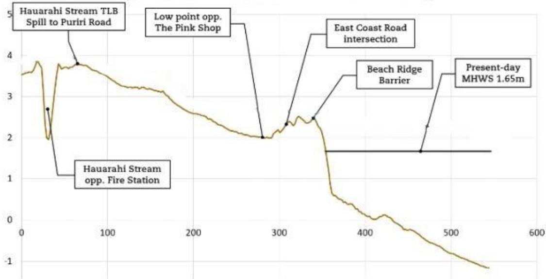
**Figure 15 Northern Kaiaua ground elevation cross-section indicating key locations of flooding from overflows from the Huarahi Stream (Chambers J, 2020, pp.10).**
