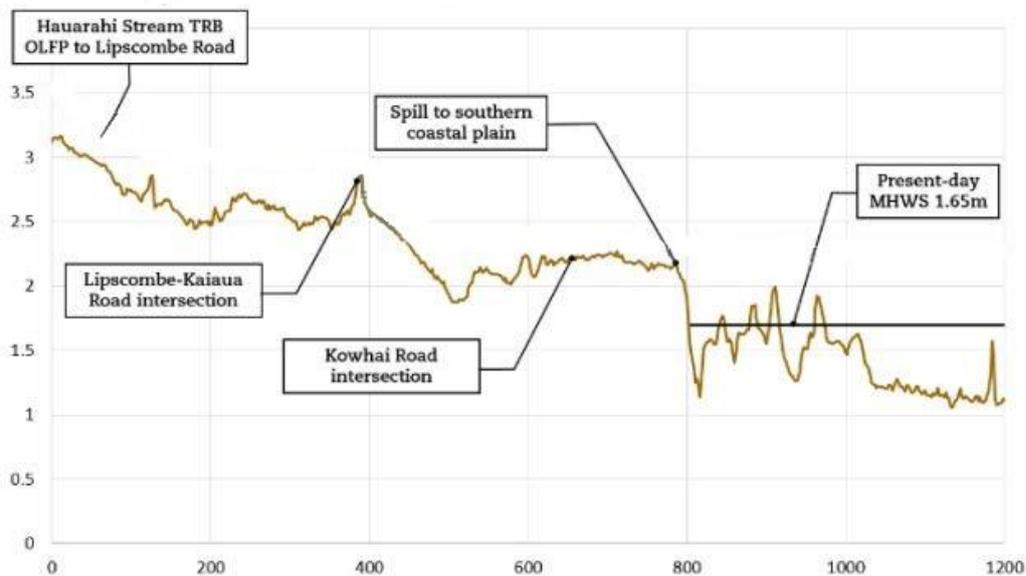
**Figure 16** Southern Kaiaua ground elevation cross-section indicating key locations of flooding from overflows from the Haurahi Stream (Chambers J, 2020, pp.10).
