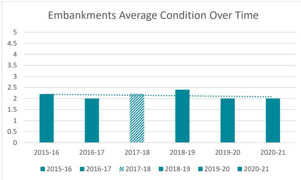
Average condition has been mostly stable with some fluctuations, suggesting the stopbank maintenance is keeping pace with any degradation that is occurring. The patterned bar denotes an interpolated value.
