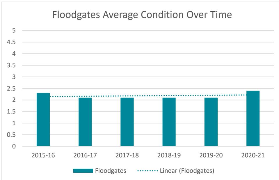
Overall Condition for Floodgates has remained stable over time, with a moderate swing towards deterioration this year.
