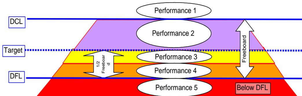
Figure 1 Performance grading for earth structures
