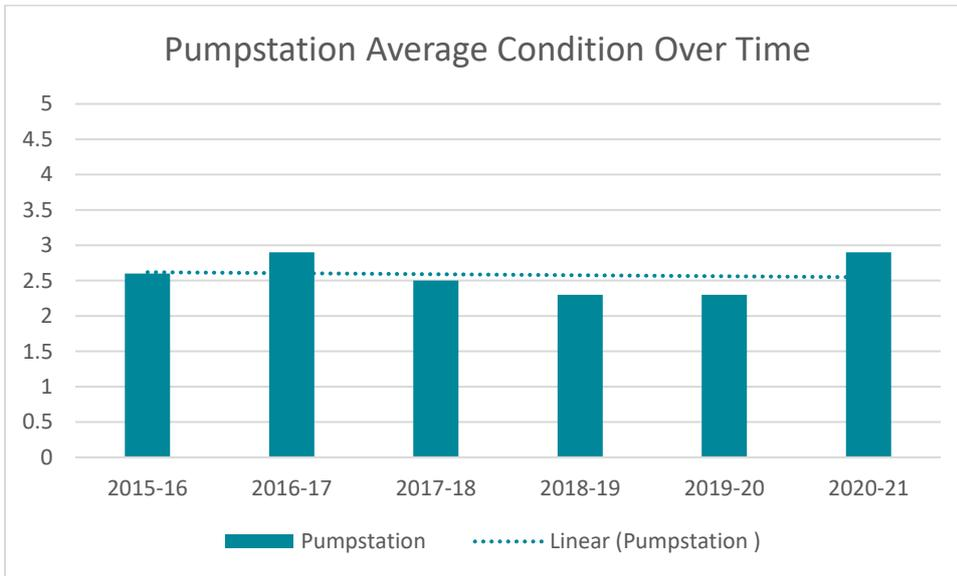
Pumpstation Average Condition has remained relatively stable over the last six years, although the overall average condition is the among the highest in the zone; almost all other asset types in Lower Waikato are in better condition than the Pumpstations and their components. As discussed in section 4.1, Pumpstations are poorly managed region wide and further investigation is required as to where improvements can be made.
