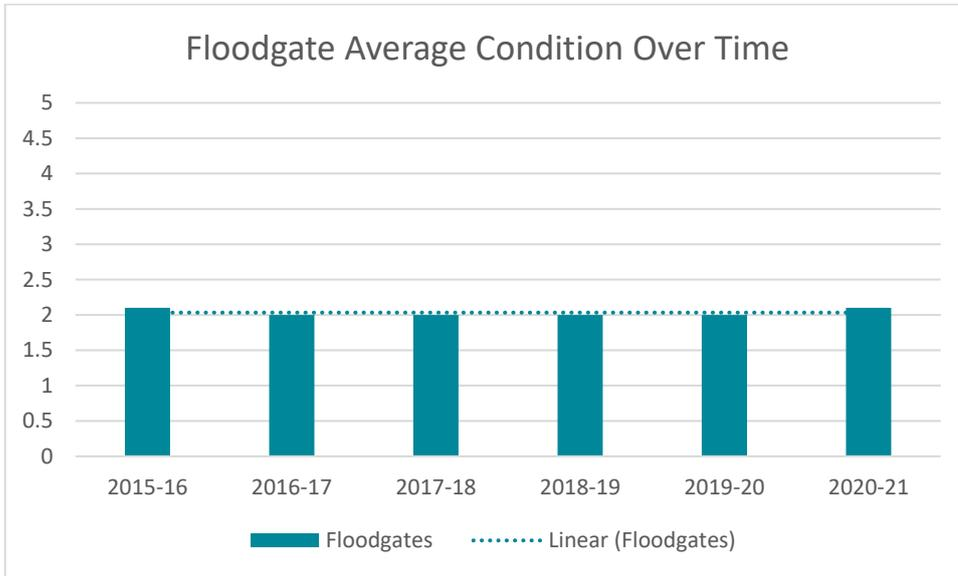
The trend is exceptionally stable over the last 6 years, with almost no fluctuation. This suggests that maintenance is keeping pace with natural deterioration.
