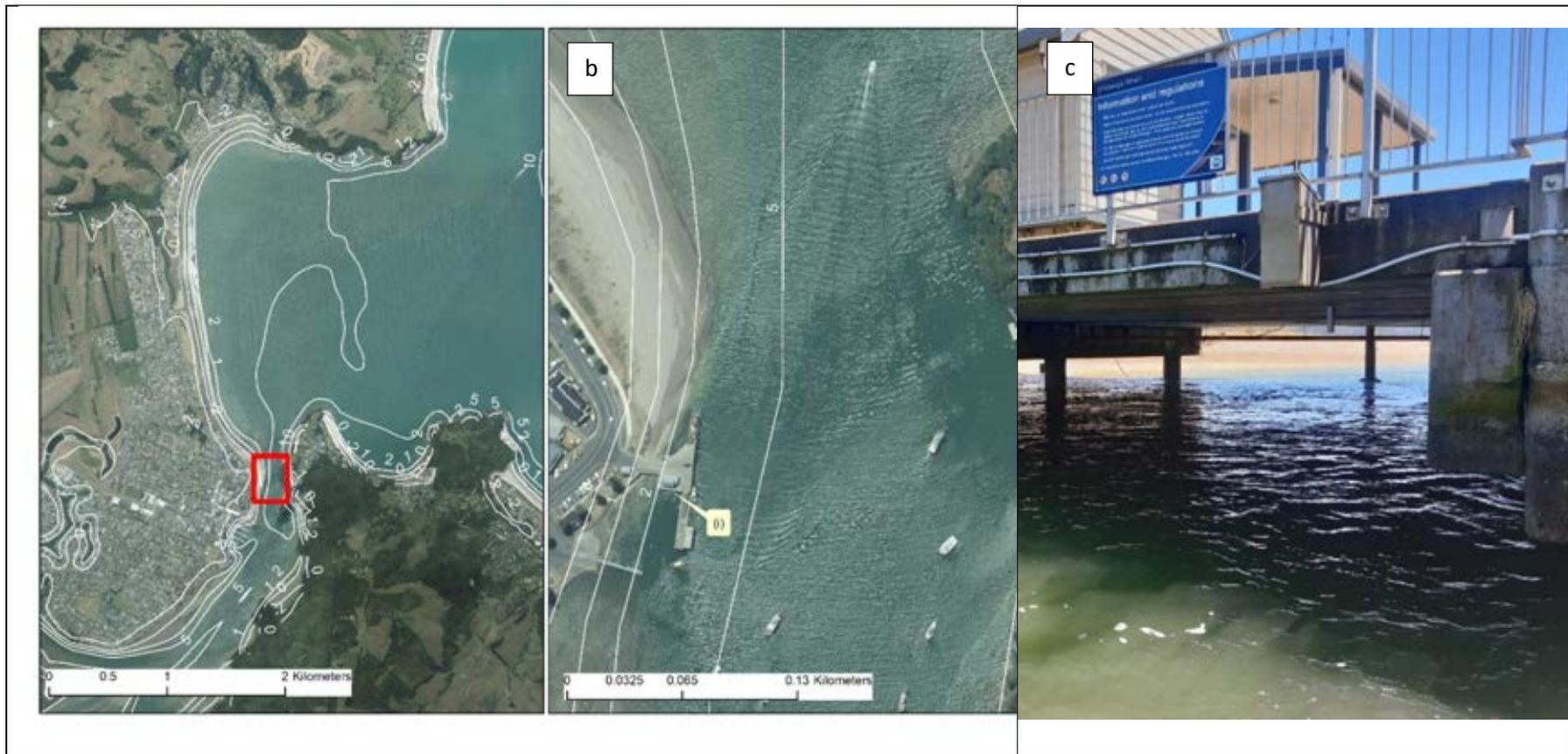
Figure 15. Whitianga Wharf tide gauge location showing the wider area (a) and Whitianga Wharf (b and c) with the tide gauge instrumentation (i). Extent of (b) is shown as a red box (a). Depth contours are in metres below to Auckland Vertical Datum 1946 (AVD-46) from a compilation of all available bathymetry in the Waikato region (Gardiner and Jones, 2020). AVD-46 is 0.0094 m below Whitianga Wharf gauge zero datum (MVD-53).
