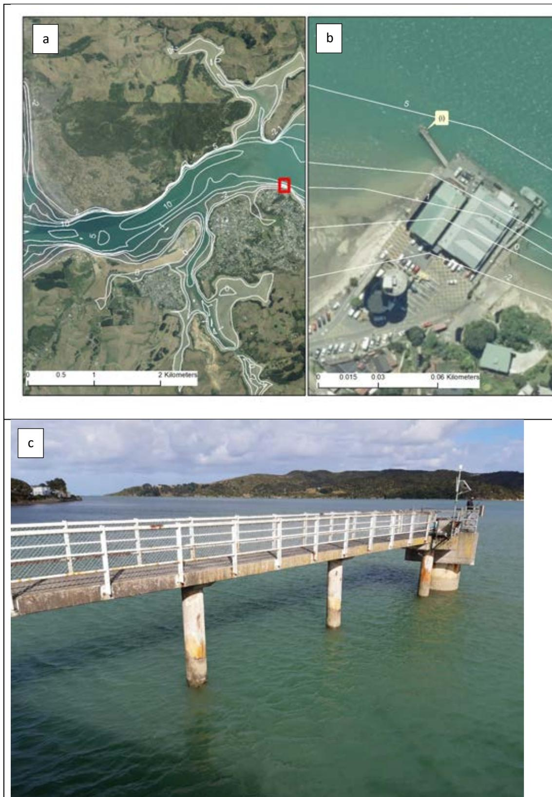
**Figure 11. Raglan Wharf tide gauge location showing the wider area (a) and Raglan Wharf (b and c) with the tide gauge instrumentation (i). Extent of (b) is shown as a red box (a). Depth contours are in metres below MVD-53 from a compilation of all available bathymetry in the Waikato Region (Gardiner and Jones, 2020).**
