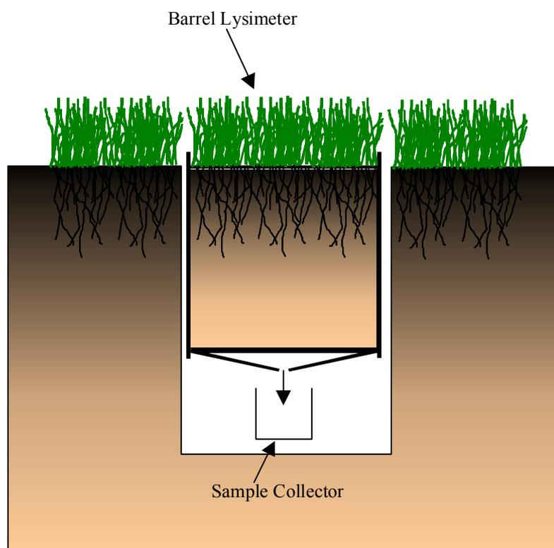
Figure 21. Concept sketch of barrel lysimeters.
