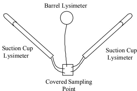
**Figure 25. Schematic diagram: Plan view of instrument set showing all sampling tubes coming to the sampling point.**
