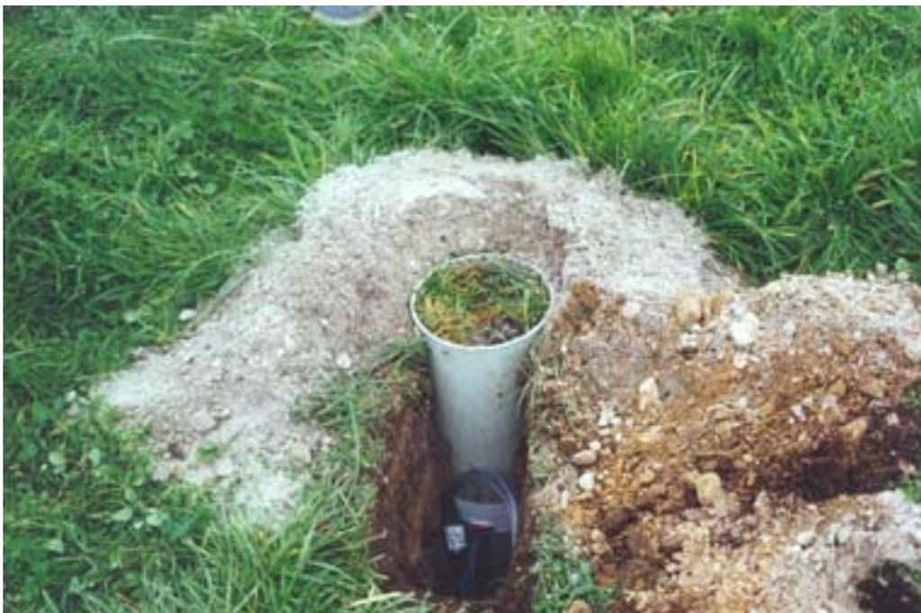
**Figure 23. Barrel lysimeter prior to installation flush with the soil surface.**
