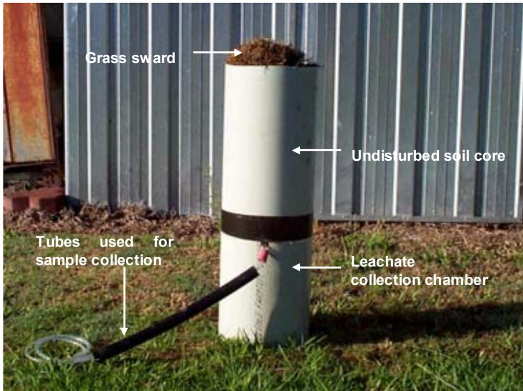
**Figure 22. Barrel lysimeter used in the trial, showing undisturbed soil core, leachate collection chamber and sample collection tubing.**
