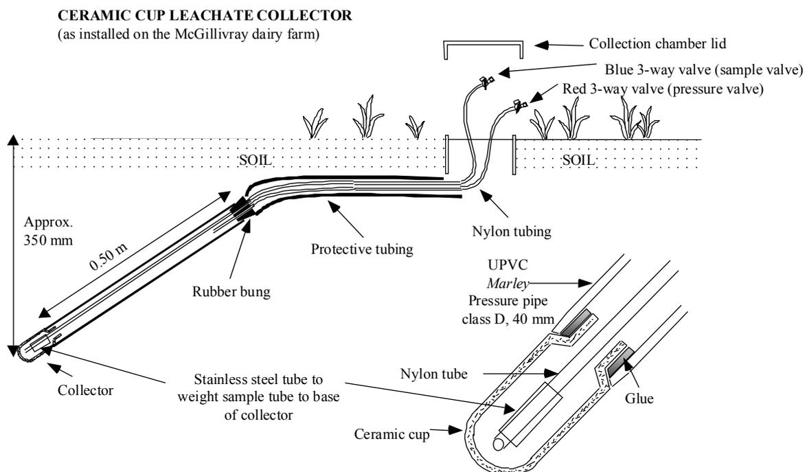
**Figure 24. Ceramic cup soil solution sampler installed in the trial.**
