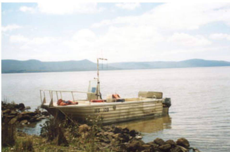
**Figure 20: Tracking set up on IFS boat – directional antenna attached to receiver near steering position**
