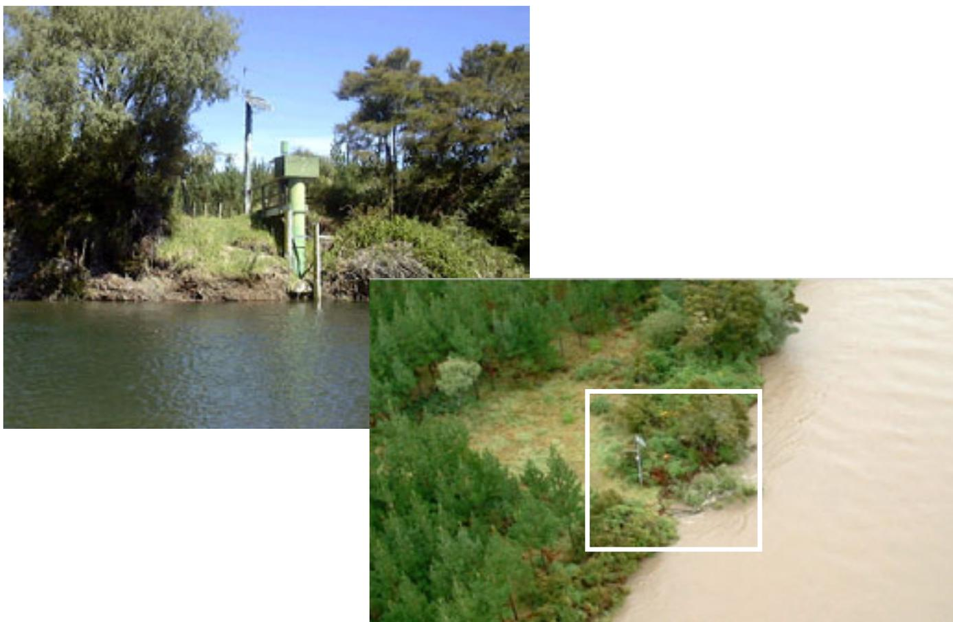
**Figure 3: Before and after photos of the Tuaranga Taupo river level recorder that was destroyed in the event.**
