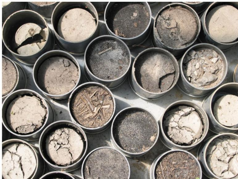
**Figure 9:** Dried sediment cores showing a range of sediment types sampled.
