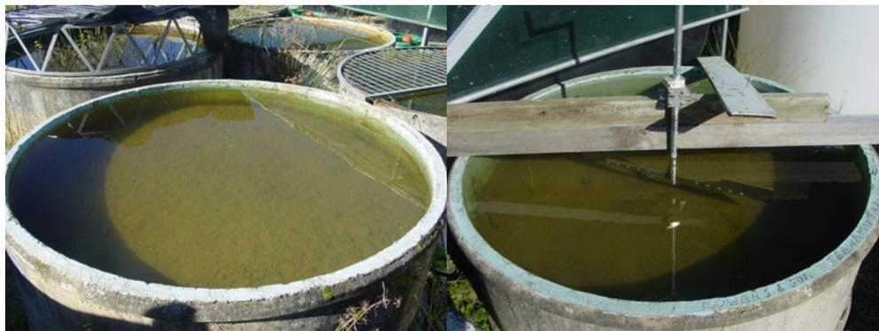
**Figure 11:** Control (left) and 2-months-dry (right), 17 May 2004. The 2-month-dry trough has the stirrer in place, just before beginning the resuspension experiment.
