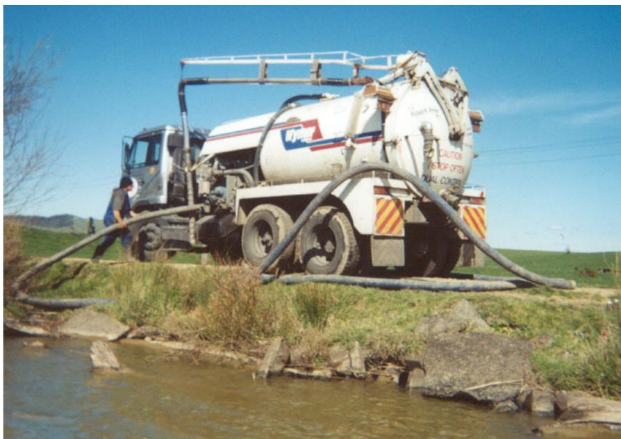
**Figure 3:** Drain suction vehicle used to collect ~6 m<sup>3</sup> of lakebed sediment.
