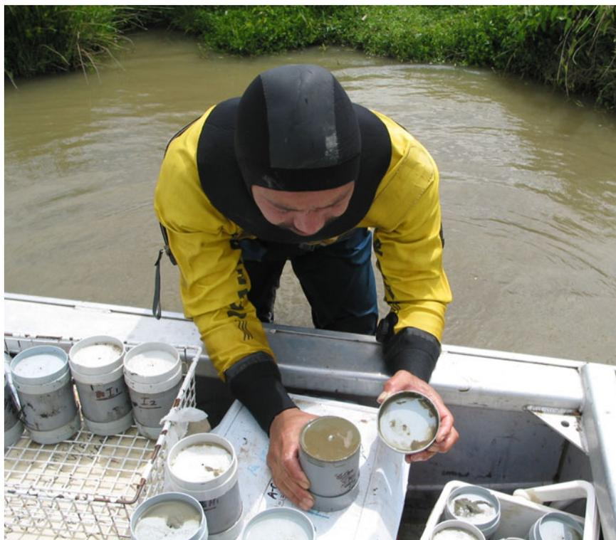
**Figure 8:** An intact core from 1.3 m depth is being checked before storage.
