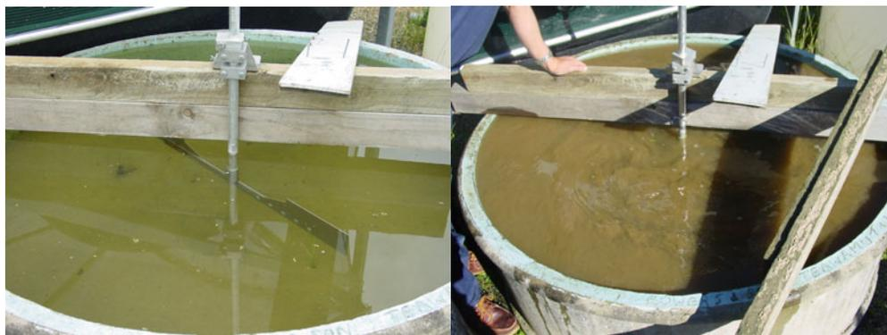
**Figure 6:** 2-months-dry trough with stirrer paddle in place, before (left) and during (right) stirring, 23 Feb 2004 (Table 1).
