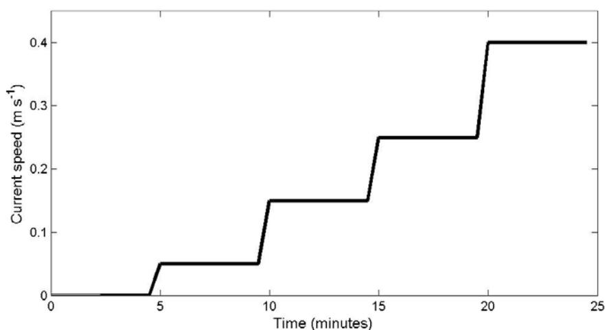
**Figure 7:** Example of current speed regime applied during sediment resuspension experiments.
