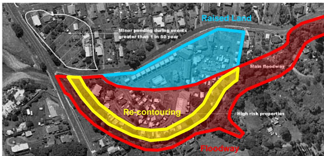
**Figure 10 Proposed floodway works**
