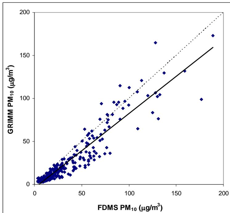
**Figure 2-2** Scatterplot of hourly average PM<sub>10</sub> data obtained from an FDMS permanently installed at Woolston, Christchurch, and a GRIMM instrument, collocated between 6 August and 20 August 2008 (from Olivares et al. 2008b). Linear regression line (solid line) has equation  $y=0.9x-4$  ( $r^2=0.89$ ) and 1-1 line is plotted for comparison (dotted line). FDMS data were provided by Environment Canterbury.
