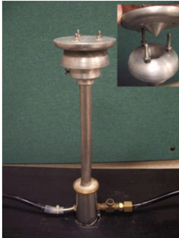
**Figure 2-3: Sample tube intake, showing (inset) convex top-piece designed to direct flow into the tube.**
