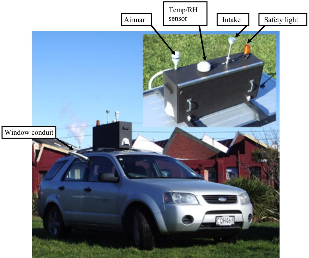
**Figure 2-1: Mobile monitoring vehicle and (inset) rooftop enclosure. Rooftop instrumentation (including Airmar and temperature + relative humidity sensor) and air intake is shown.**
