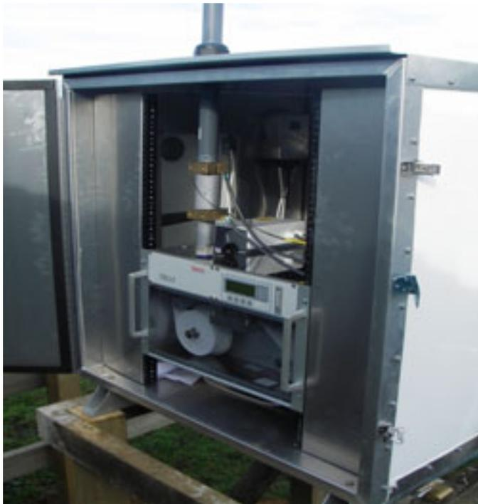
Figure 8.2: Putaruru air quality monitor (Source: Environment Waikato)
