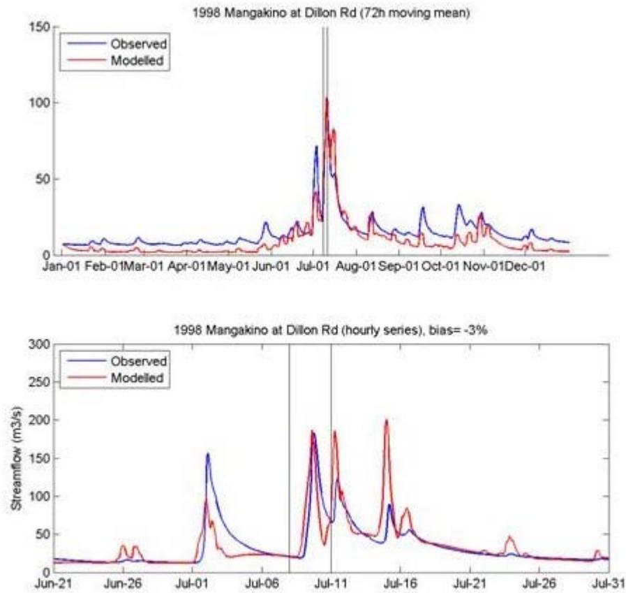
**Figure 19: TopNet validation plot for 1998 flood, Mangakino at Dillon Road. Top panel shows observed and modelled 72-h moving mean flows in  $m^3s^{-1}$ ; Bottom panel shows observed and modelled hourly flows in  $m^3s^{-1}$ .**
