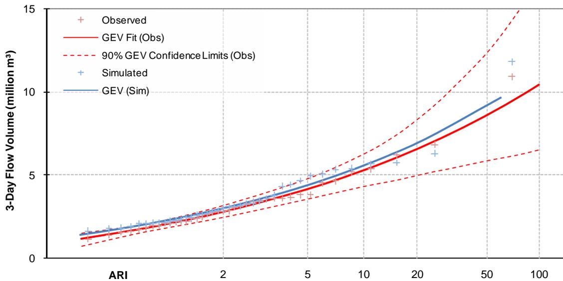
Figure 23: Distribution of observed and simulated 3-day flow volume annual maxima for Waitotapu at Reporoa calibration (using Gringorton plotting positions).
