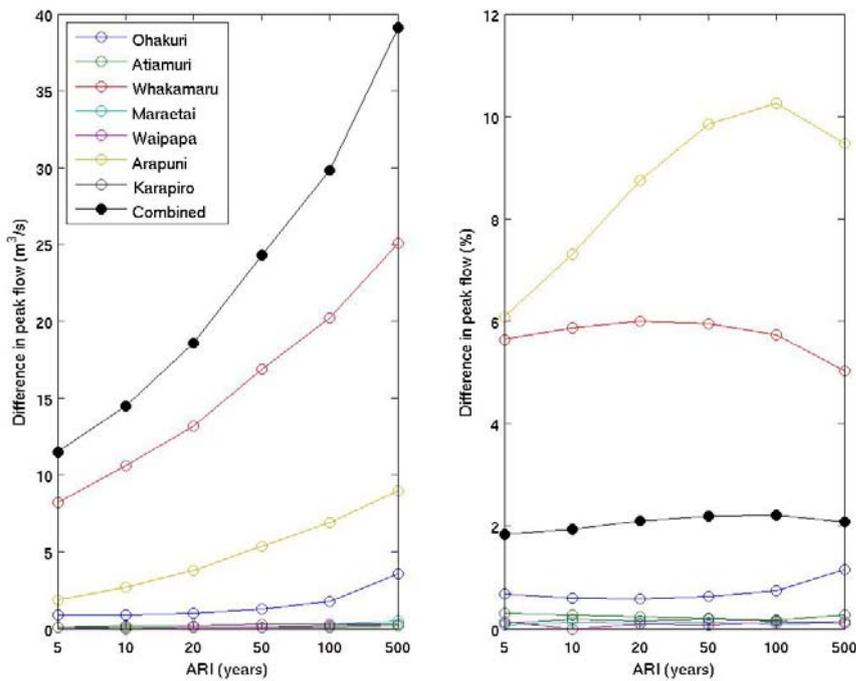
Figure 59: Peak flow differences in m<sup>3</sup>/s (left) and percent (right) for the converted scenarios compared to current land use hydrographs (TopNet simulations, 1998 rainfall pattern). Results are displayed for different return intervals and the dam catchments as well as the outlet. “Combined” refers to the total Taupo-Karapiro inflows.
