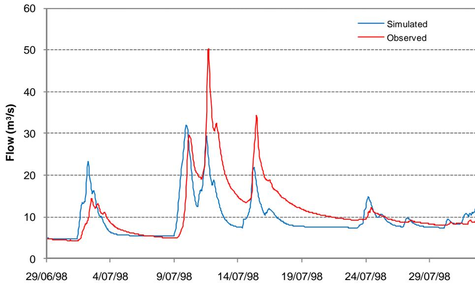
**Figure 37: Observed and simulated flow at Pokaiwhenua at Puketurua calibration for the July 1998 flood.**
