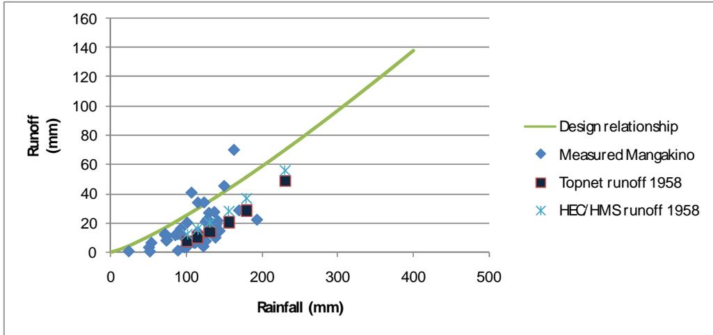
**Figure 47: Measured storm runoff produced by total storm rainfalls and maximum design relationship in the Mangakino Stream compared to storm runoff into Maraetai reservoir predicted by HEC-HMS and TopNet models for rainfalls of 5 to 500 year ARI with 1958 temporal pattern.**
