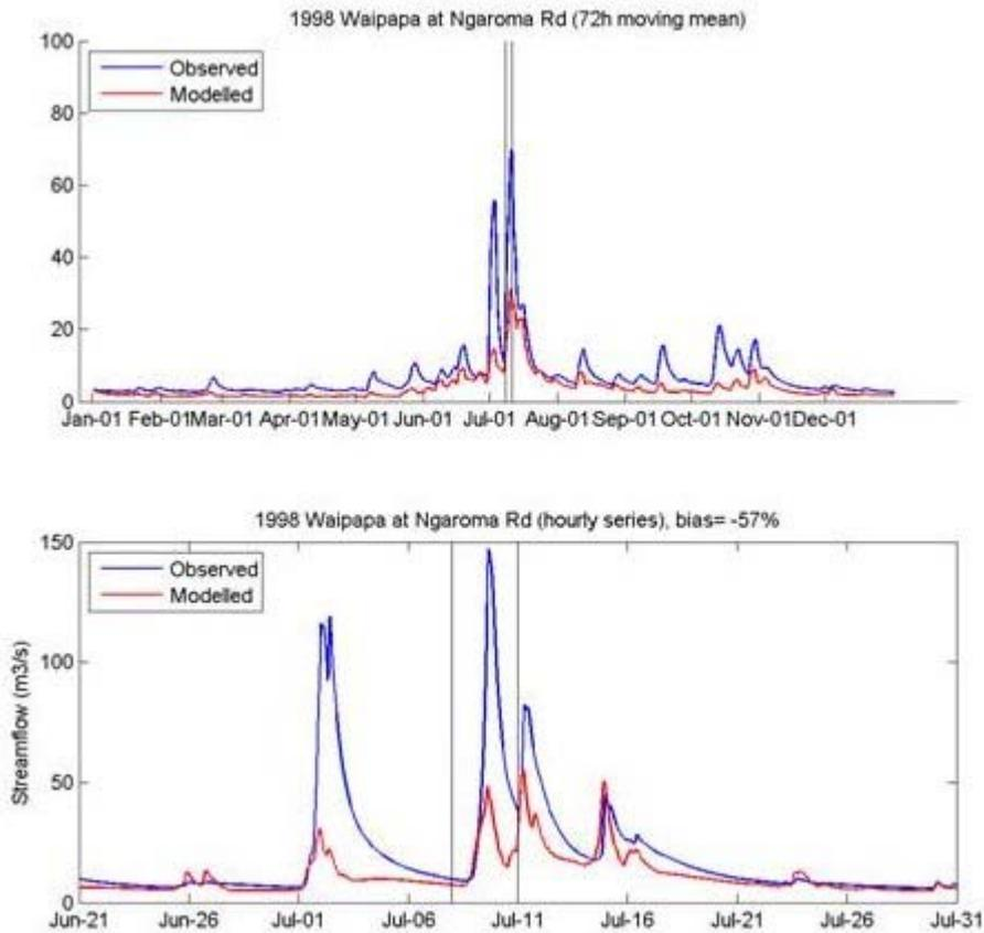
Figure 20: TopNet validation plot for 1998 flood, Waipapa at Ngaroma Road. Top panel shows observed and modelled 72-h moving mean flows in  $m^3s^{-1}$ ; Bottom panel shows observed and modelled hourly flows in  $m^3s^{-1}$ .
