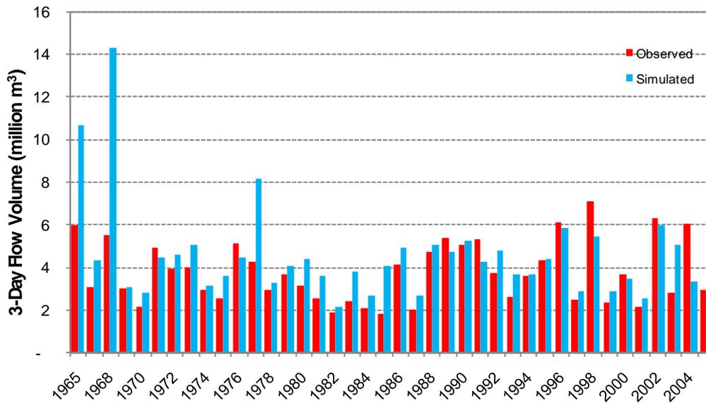
**Figure 36: Observed and simulated 3-day flow volume annual maxima for Pokaiwhenua at Puketurua calibration.**
