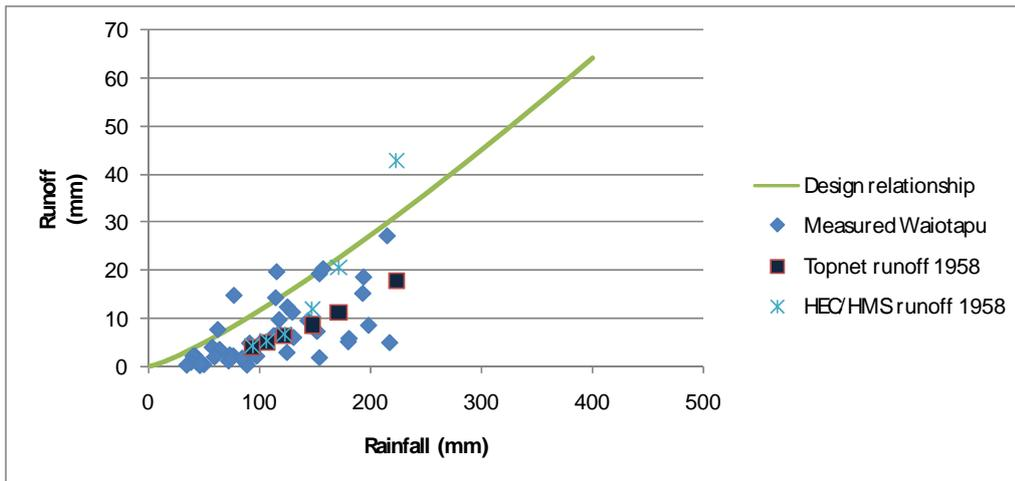
**Figure 45: Measured storm runoff produced by total storm rainfalls and maximum design relationship in the Waiotapu Stream compared to storm runoff into Ohakuri reservoir predicted by HEC-HMS and TopNet models for rainfalls of 5 to 500 year ARI with 1958 temporal pattern.**
