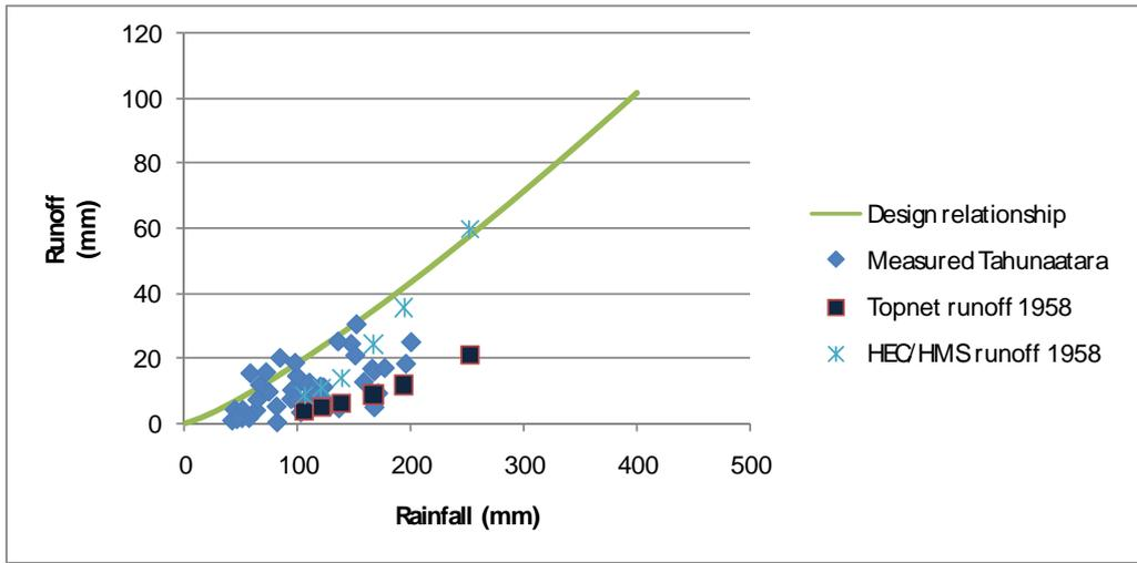
**Figure 46: Measured storm runoff produced by total storm rainfalls and maximum design relationship in the Tahunaatara Stream compared to storm runoff into Atiamuri reservoir predicted by HEC-HMS and TopNet models for rainfalls of 5 to 500 year ARI with 1958 temporal pattern.**
