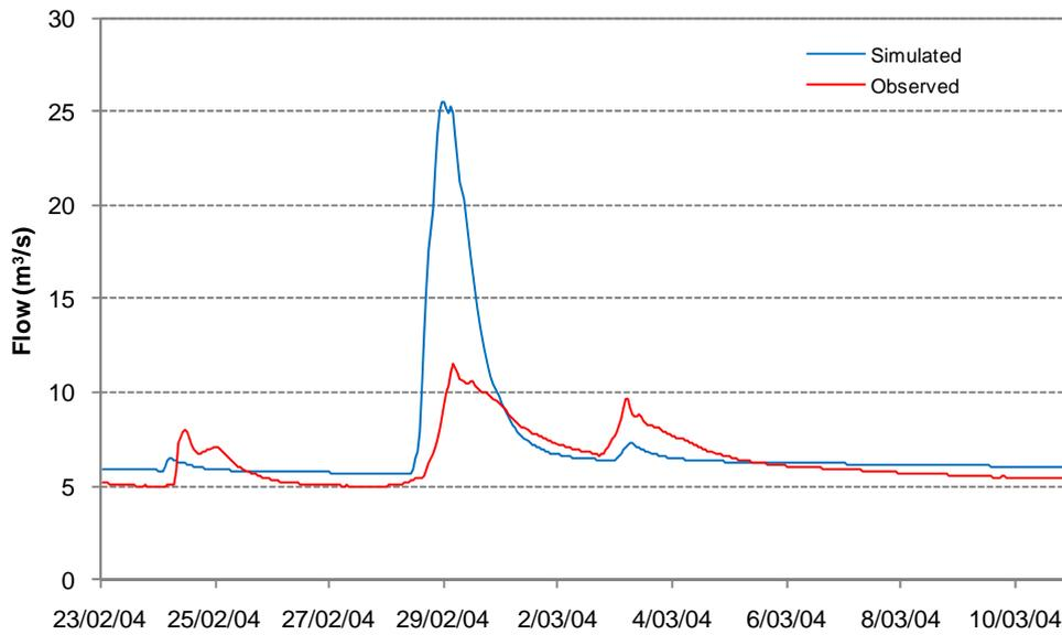
**Figure 38: Observed and simulated flow at Pokaiwhenua at Puketurua calibration for the February 2004 flood.**
