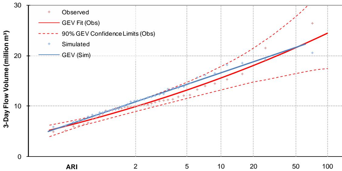
**Figure 31: Distribution of observed and simulated 3-day flow volume annual maxima for Mangakino at Dillon Rd calibration (using Gringorton plotting positions).**
