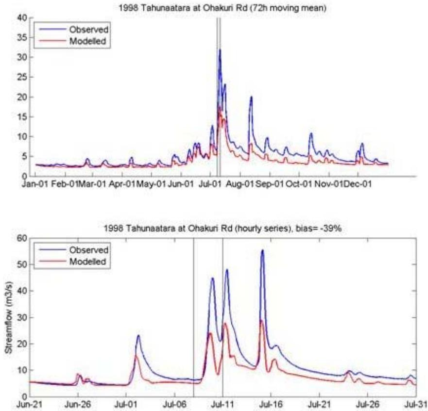
**Figure 18: TopNet validation plot for 1998 flood, Tahunaatara at Ohakuri Road. Top panel shows observed and modelled 72-h moving mean flows in  $m^3s^{-1}$ ; Bottom panel shows observed and modelled hourly flows in  $m^3s^{-1}$ .**
