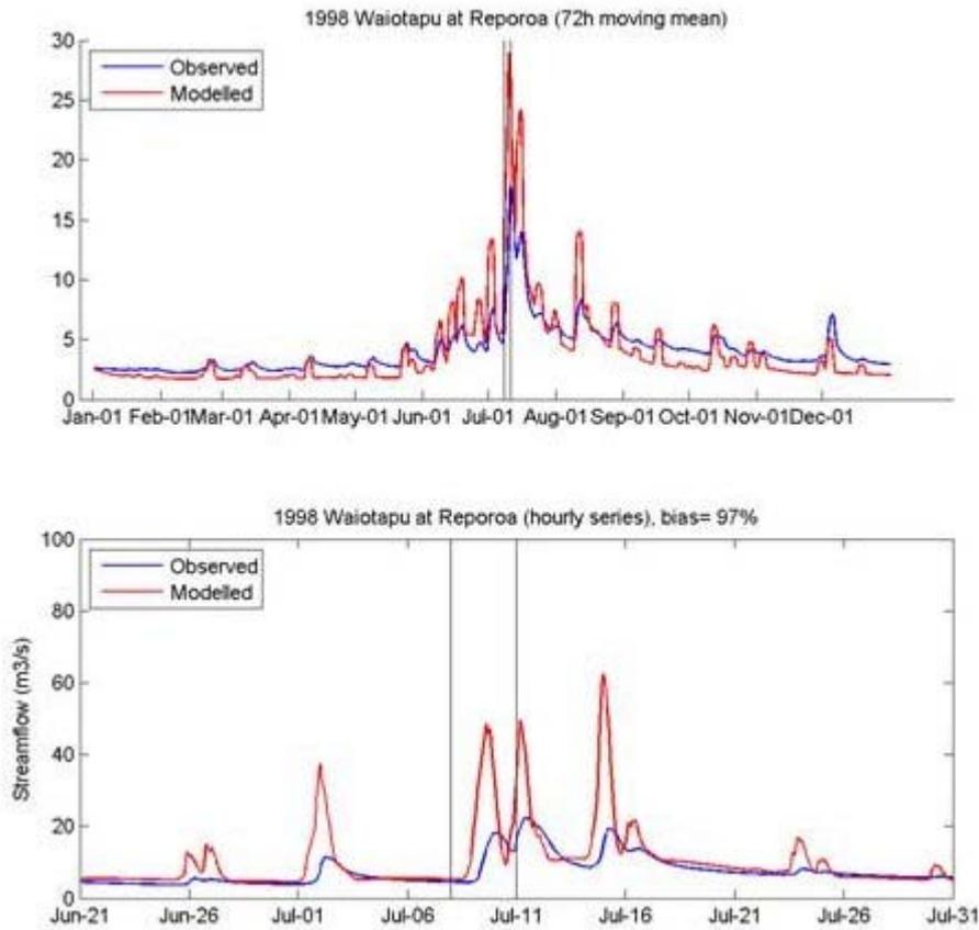
**Figure 17: TopNet validation plot for 1998 flood, Waiotapu at Reporoa. Top panel shows observed and modelled 72-h moving mean flows in  $m^3s^{-1}$ ; Bottom panel shows observed and modelled hourly flows in  $m^3s^{-1}$ .**
