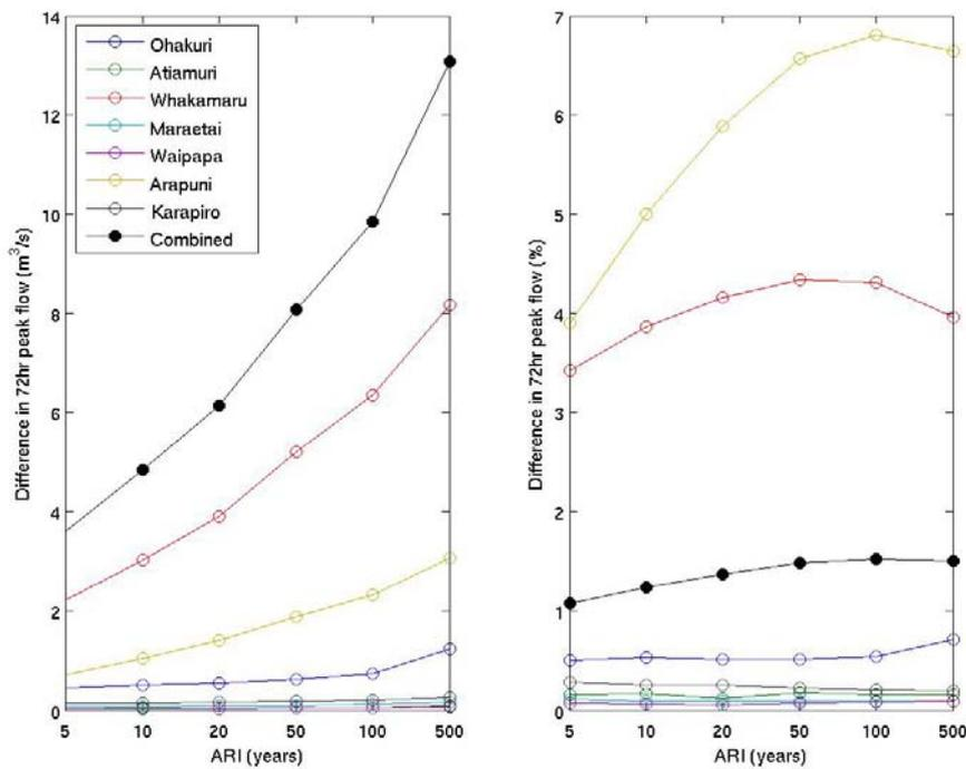
Figure 60: Peak 72-hr flow differences in m<sup>3</sup>/s (left) and percent (right) for the converted scenarios compared to current land use hydrographs (TopNet simulations, 1998 rainfall pattern). Results are displayed for different return intervals and the dam catchments as well as the outlet. “Combined” refers to the total Taupo-Karapiro inflows.
