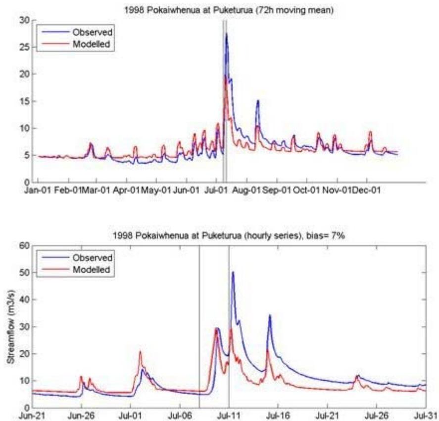
**Figure 21: TopNet validation plot for 1998 flood, Pokaiwhenua at Puketuru. Top panel shows observed and modelled 72-h moving mean flows in  $m^3s^{-1}$ ; Bottom panel shows observed and modelled hourly flows in  $m^3s^{-1}$ .**
