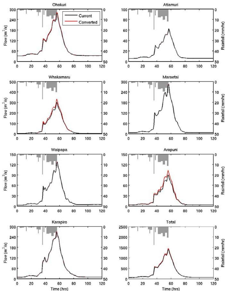
**Figure 58: Simulated hydrographs for each of the dam catchments as simulated by TopNet for the 100-year rainfall event for 1958 under current (black lines) and converted (red lines) land use scenarios.**
