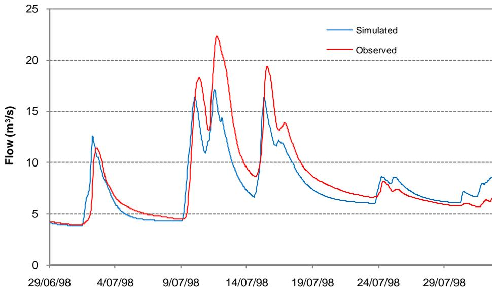
**Figure 25: Observed and simulated flows for Waiotapu at Reporoa calibration (July 1998 flood).**
