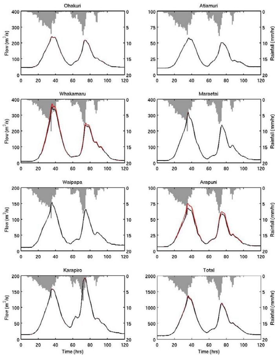
**Figure 57: Simulated hydrographs for each of the dam catchments as simulated by TopNet for the 100-year rainfall event for 1998 under current (black lines) and converted (red lines) land use scenarios.**
