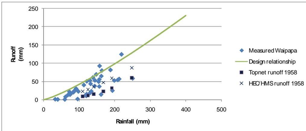
**Figure 48: Measured storm runoff produced by total storm rainfalls and maximum design relationship in the Waipapa River compared to storm runoff into Waipapa reservoir predicted by HEC-HMS and TopNet models for rainfalls of 5 to 500 year ARI with 1958 temporal pattern.**
