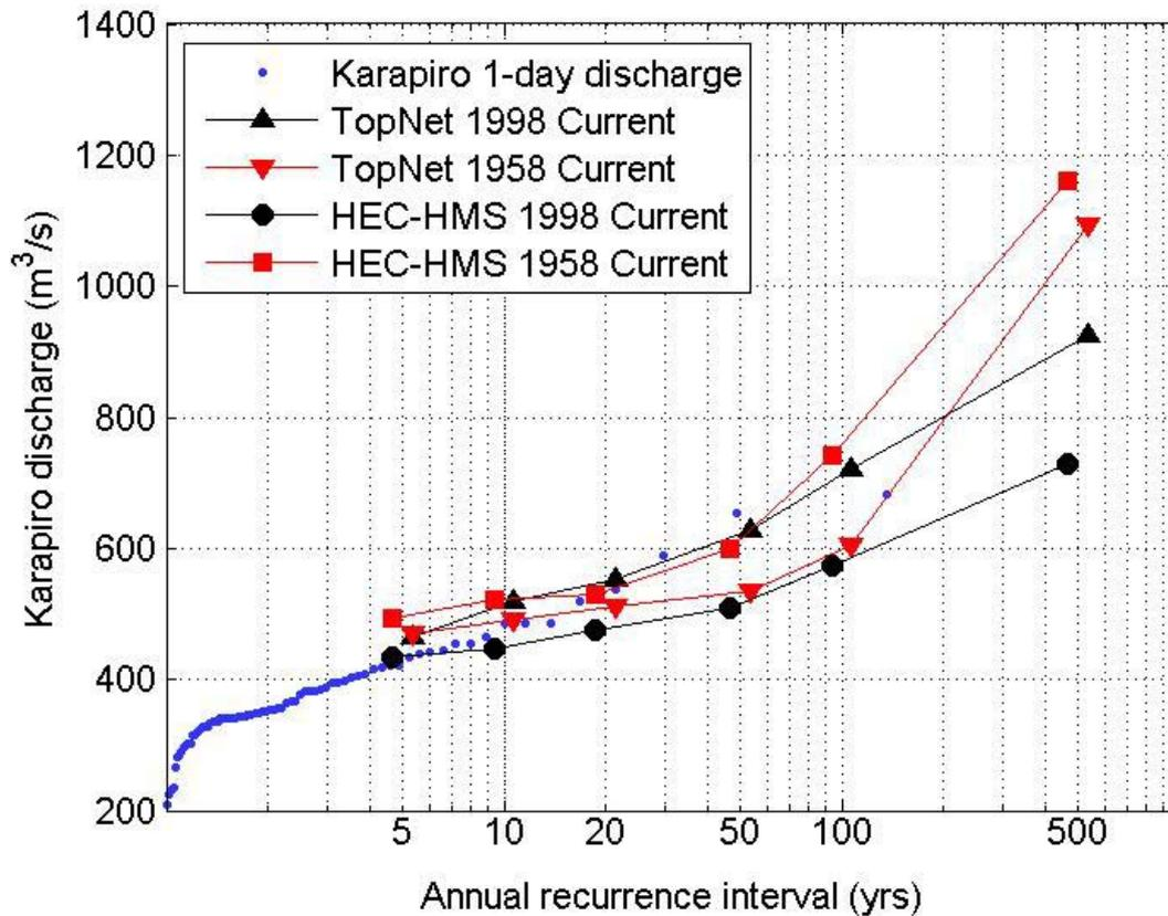
**Figure 68: Recorded annual maximum 1 day discharges and associated annual recurrence intervals from Karapiro compared with simulated discharges resulting from HEC-HMS and TopNet simulated inflows for the current land use, and with temporal patterns matching both the 1998 and 1958 storms. TopNet and HEC-HMS results are horizontally offset from the exact ARI for the sake of clarity.**
