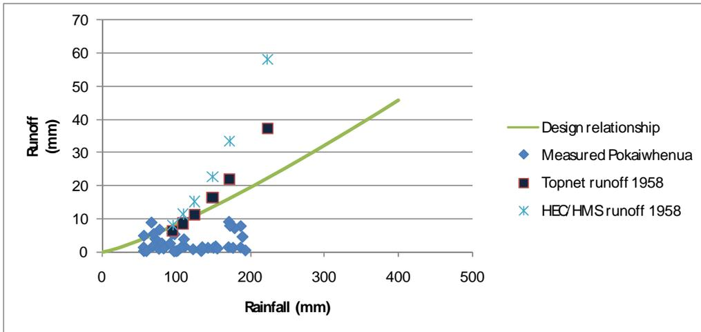
**Figure 49: Measured storm runoff produced by total storm rainfalls and maximum design relationship in the Pokaiwhenua Stream compared to storm runoff into Karapiro reservoir predicted by HEC-HMS and TopNet models for rainfalls of 5 to 500 year ARI with 1958 temporal pattern.**
