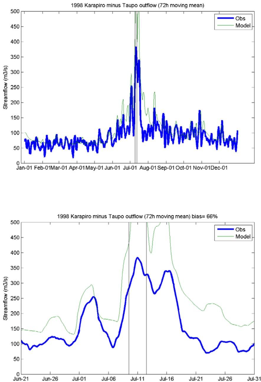
**Figure 16: TopNet validation plot for 1998 flood, for the difference between Karapiro and Taupo outflows. Top panel shows observed and modelled 72-h moving mean flows for entire year; Bottom panel shows detail at time of flood.**
