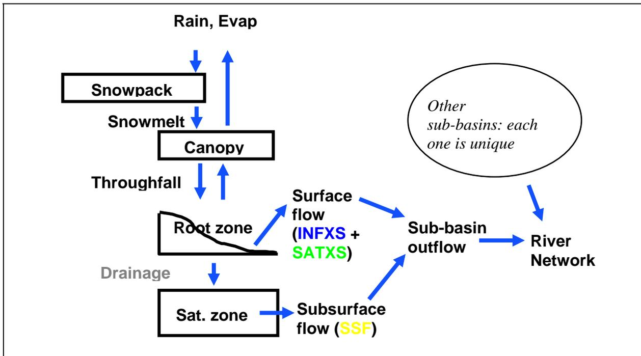
Figure 8: Overview of TopNet model structure, showing the snowpack, canopy, root zone, saturated zone and river network components of the model. Arrows indicate flows of water from one model component to another.
