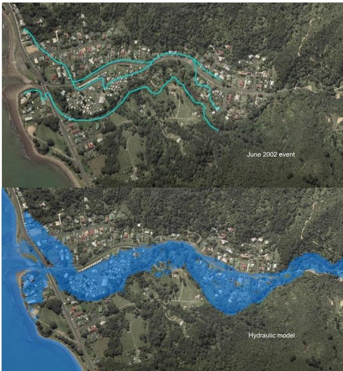
Figure 12 Comparison of modelled and observed flood extents
