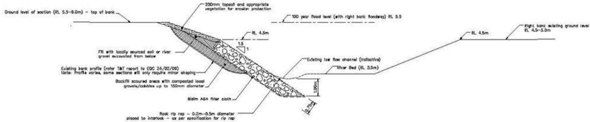
Rock size: Based on peak velocity 3m/s - ref Environment Waikato Mike 21 plots for 100y 45m flood
