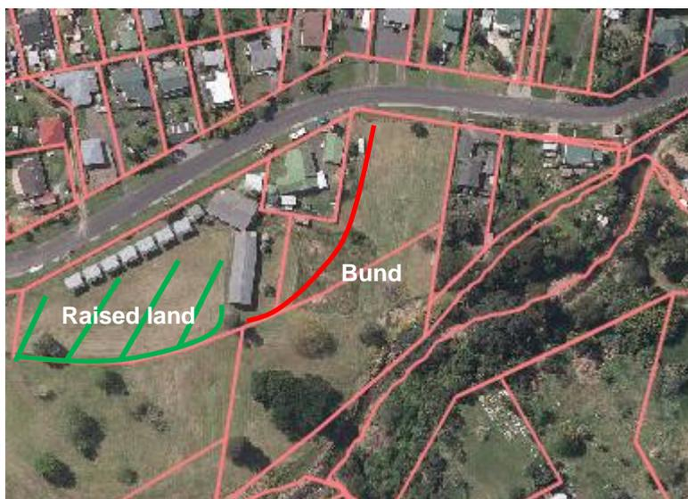
**Figure 24 Indicative alignment for bund/flood wall**
