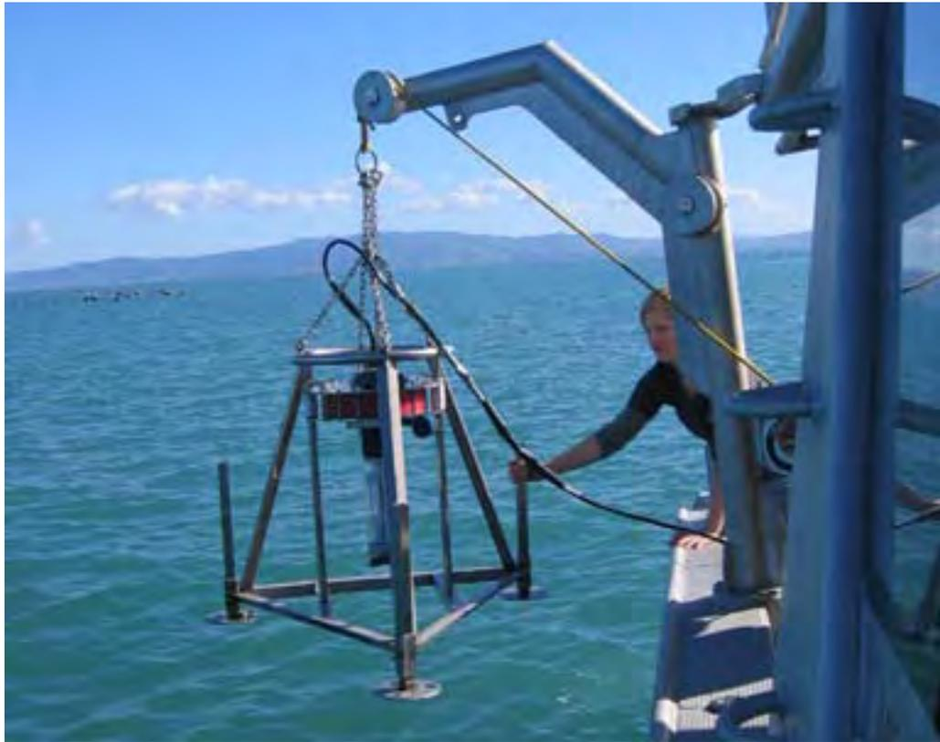
**Figure 2:** Photograph showing the NIWA Sediment Profile Imaging device (NIWA SPI-SCAN) deployed from RV Rangatahi in Wilson Bay, Firth of Thames, in September 2009.
