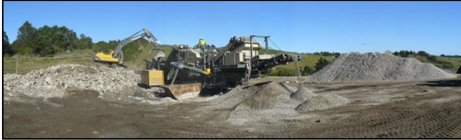
Concrete crushing machine at Recycling Park on Te Tahī St, Whakatane<sup>15</sup>
