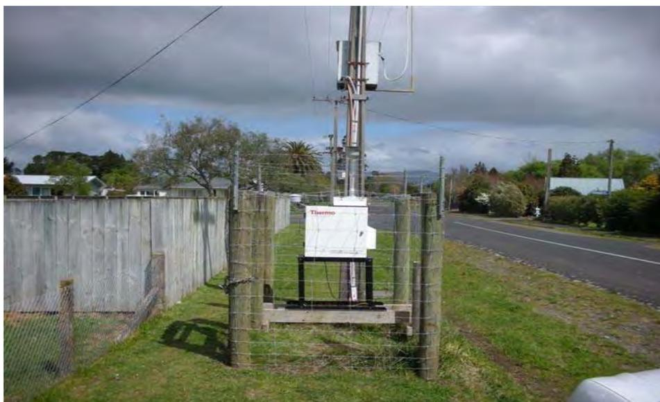
Figure 10.2: Waihi air quality monitor (Source: Environment Waikato, 2009).
