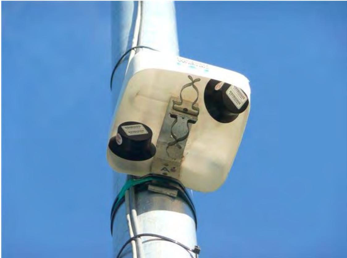
Figure 12.1: Duplicate radon detection badges co-located at an FH62 BAM monitoring site.
