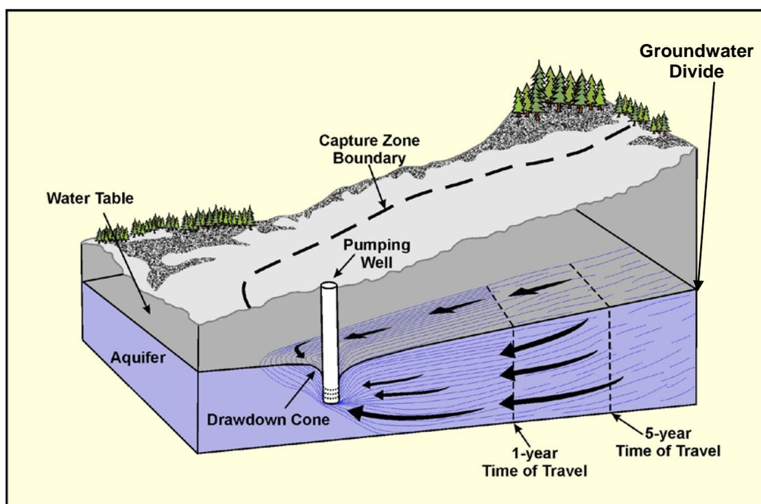
**Figure 1.2** Idealised shape of the capture zone for a well in a homogeneous anisotropic unconfined aquifer. The regional groundwater flow direction is from right to left (Fetter 1994).
