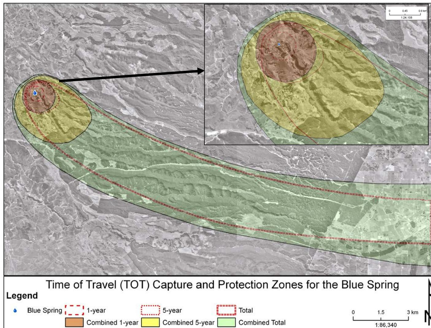
**Figure 4.5** Time of Travel (TOT) Capture Zones (CZs) delineated for the Blue Spring. Dashed lines represent TOT CZs mapped using average values in the calibrated model; solid lines represent “combined” TOT CZs based on sensitivity and uncertainty analysis.
