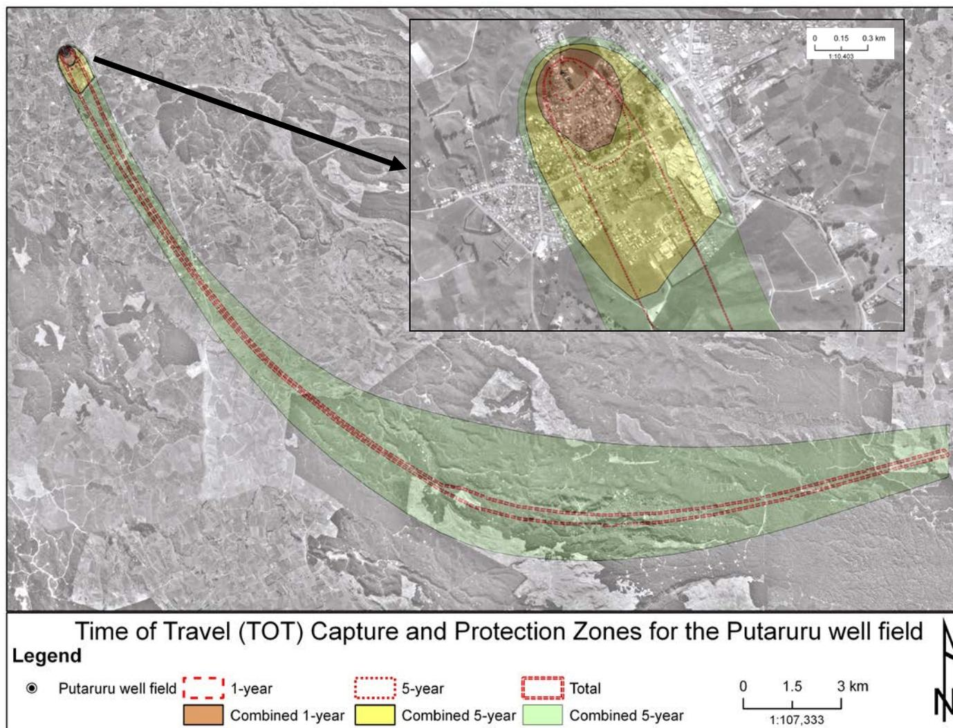
**Figure 4.4** Time of Travel (TOT) Capture Zones (CZs) delineated for the Putaruru well field. Dashed lines represent TOT CZs mapped using average values in the calibrated model; solid lines represent “combined” TOT CZs based on sensitivity and uncertainty analysis.
