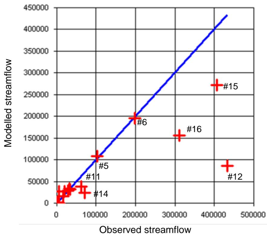
**Figure 4.3** Modelled vs. observed streamflows in m<sup>3</sup>/day from the calibrated GFLOW model.
