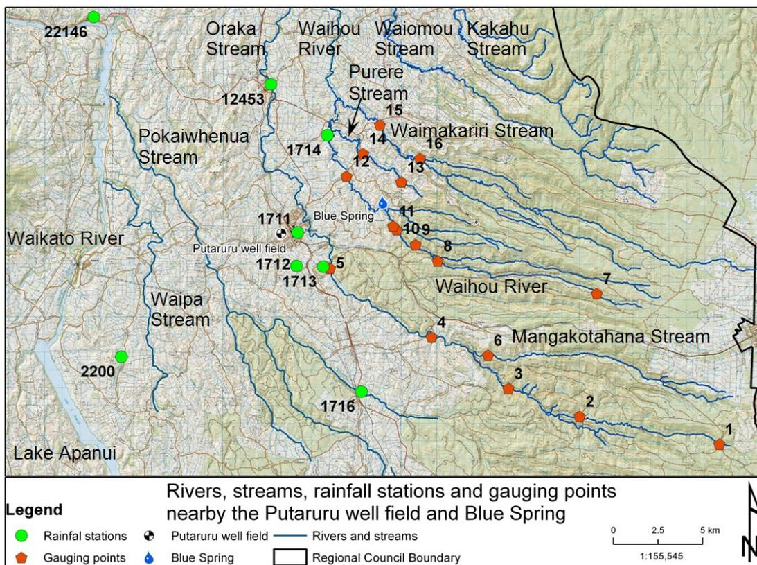
**Figure 2.5** Rivers, streams, rainfall stations and stream gauging stations nearby the Putaruru well field and Blue Spring. The numbers by the gauging points and rainfall stations are site IDs.
