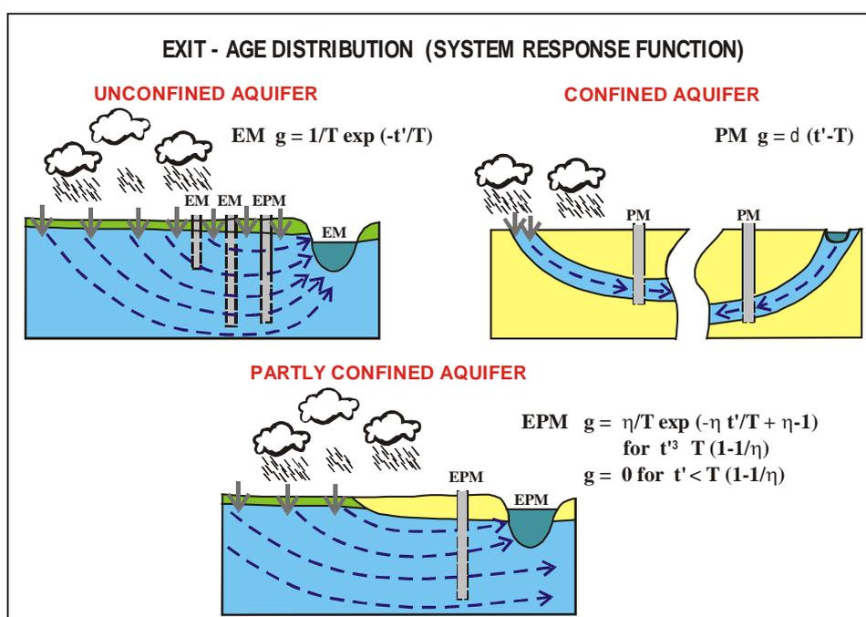
**Figure A2** Schematic groundwater flow situations and corresponding age distribution functions (see Maloszewski & Zuber (1982) for theoretical background).
