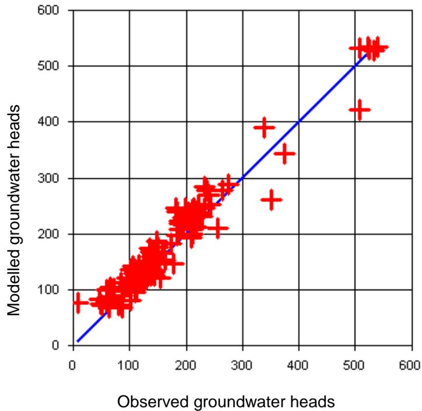
**Figure 4.2** Modelled vs. observed groundwater heads in meters from the calibrated GFLOW model.
