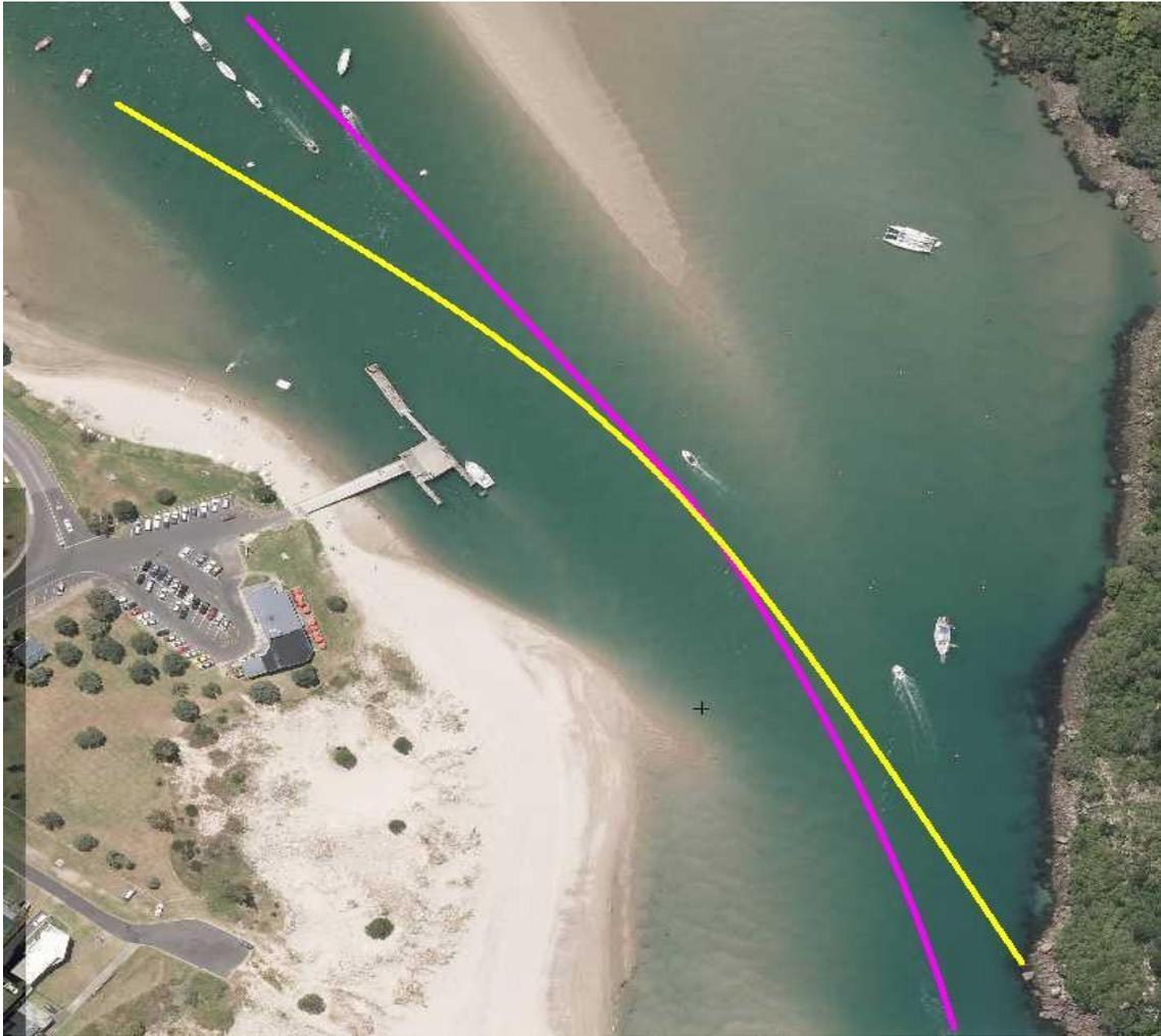
**Figure 3 Main current flow at entrance and proposed boom set**
