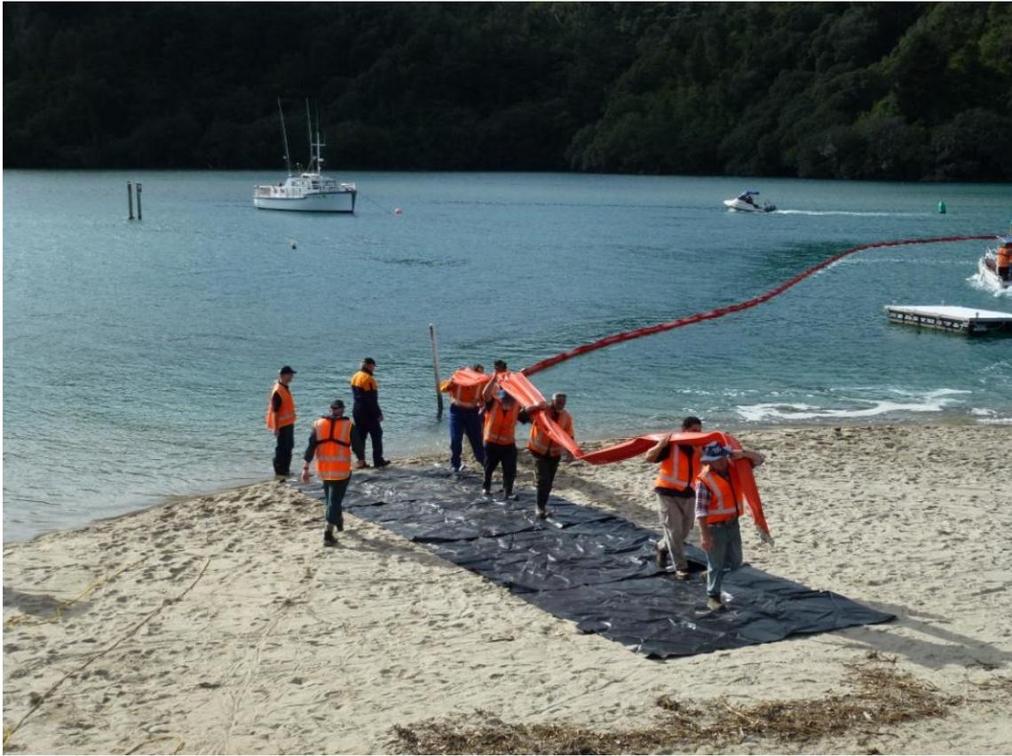
**Figure 15** Manual retrieval of boom when released from boat
