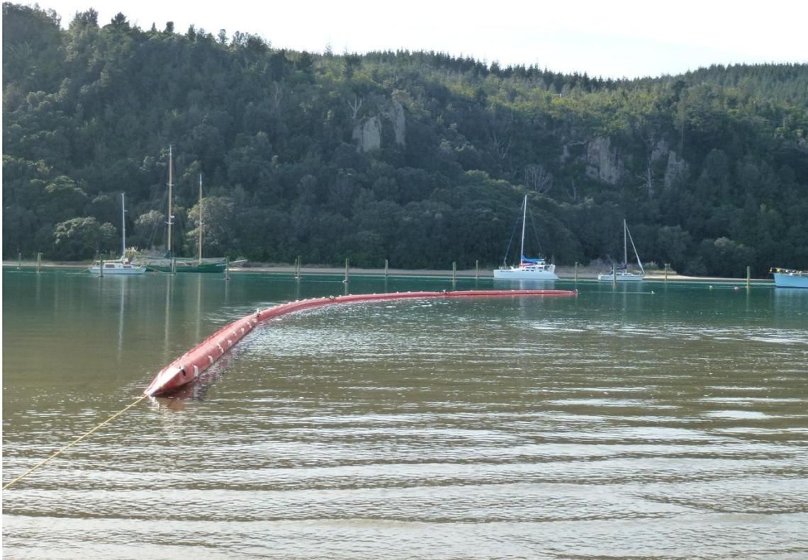
**Figure 9** Angle of boom is still too severe
