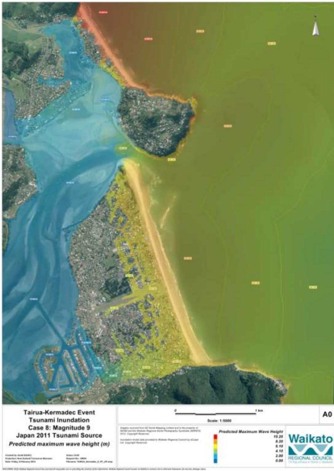
Figure 7.3 Inundation at Tairua/Pauanui from Case 8 source scenario.
