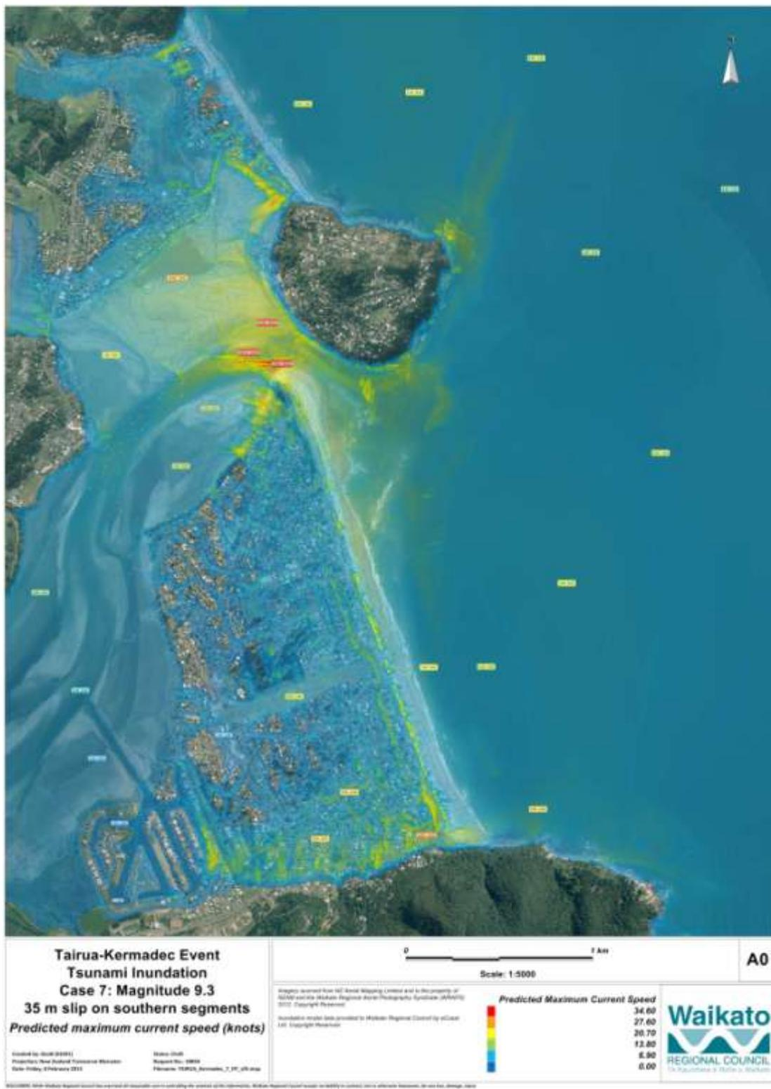
Figure 7.5 Maximum current speed at Tairua/Pauanui from Case 7 source scenario.
