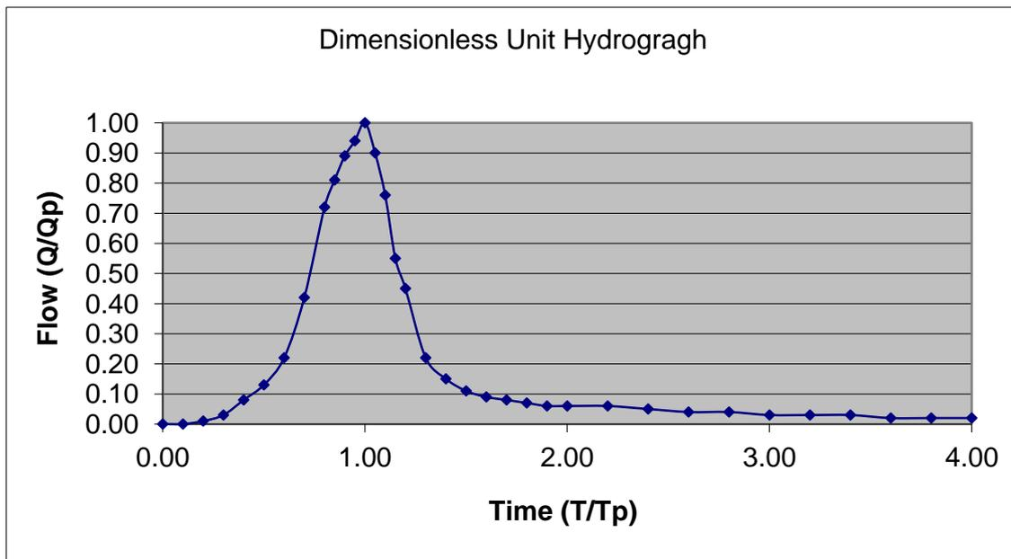
**Figure 10 Dimensionless unit hydrograph**
