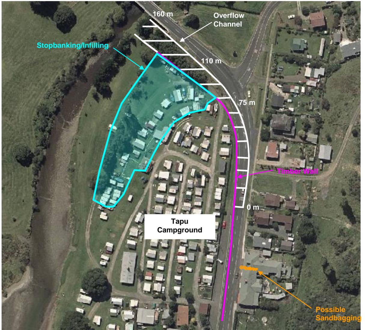
**Figure 15 Completed infill at the Tapu Campground**
