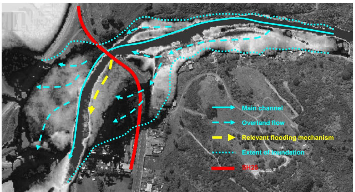
**Figure 16 Flooding mechanism relevant to stopbank and infill design**
