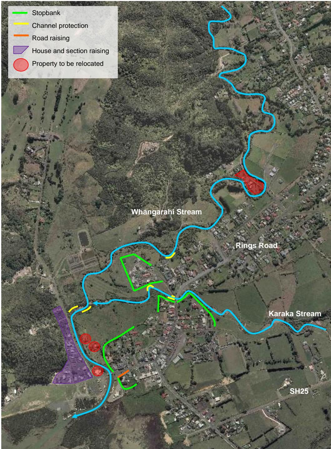
**Figure 12 Proposed flood protection scheme for Coromandel**
