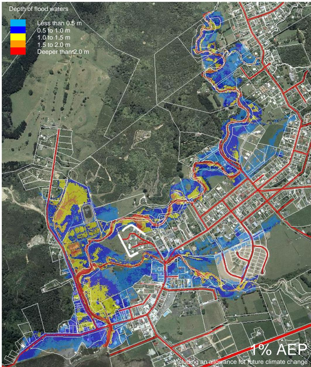
**Figure 7 Predicted flood extents for 1% AEP event (with climate change)**
