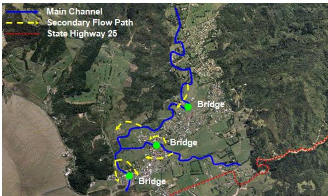
**Figure 6 Indicative flooding mechanisms in Coromandel town**
