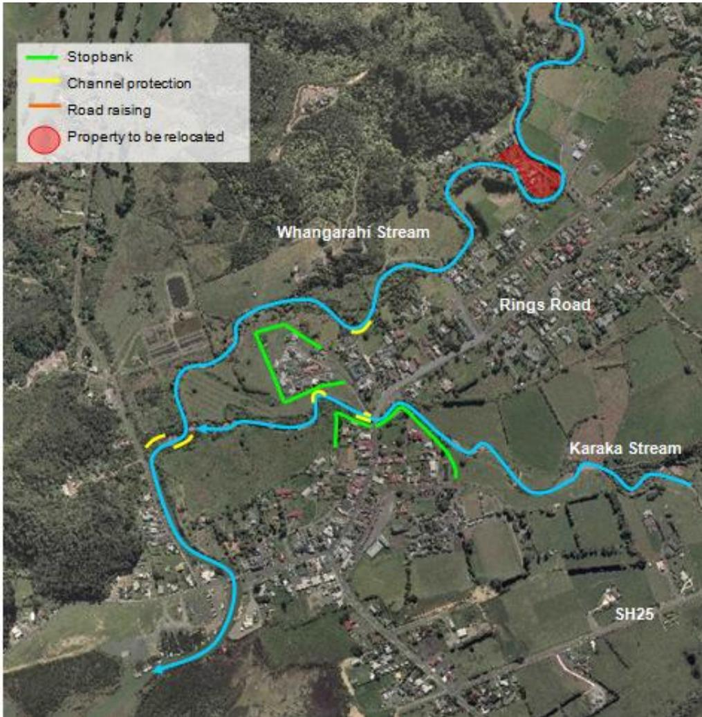
Figure 13 Completed flood mitigation works at Coromandel
