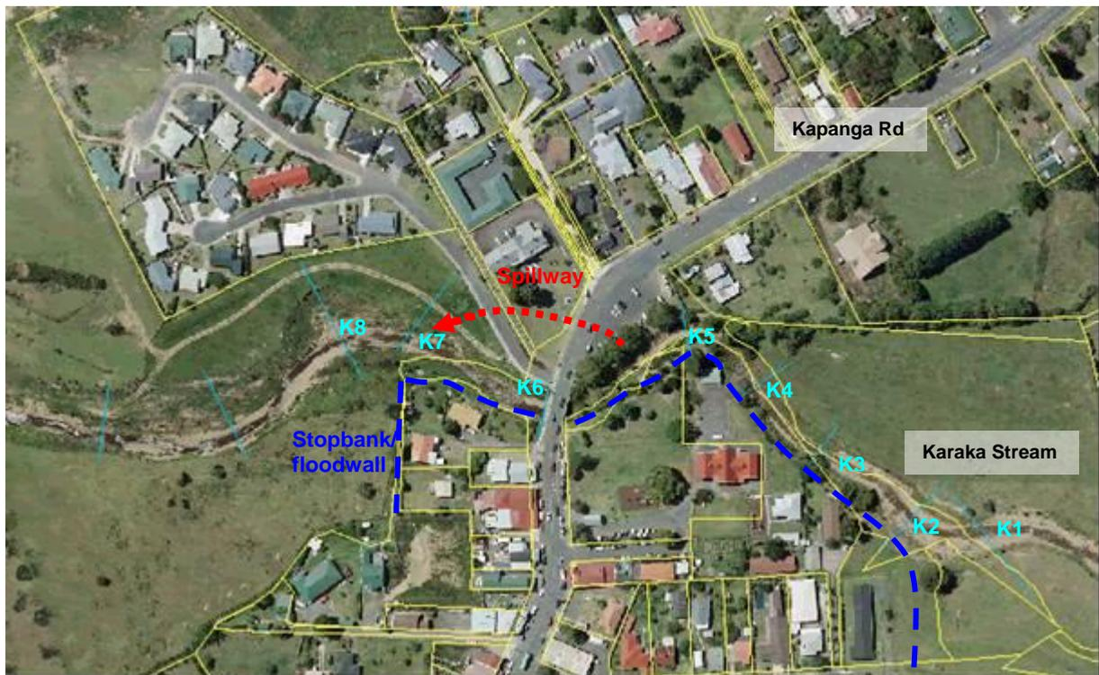
**Figure 1 Karaka Stream flood protection works**
