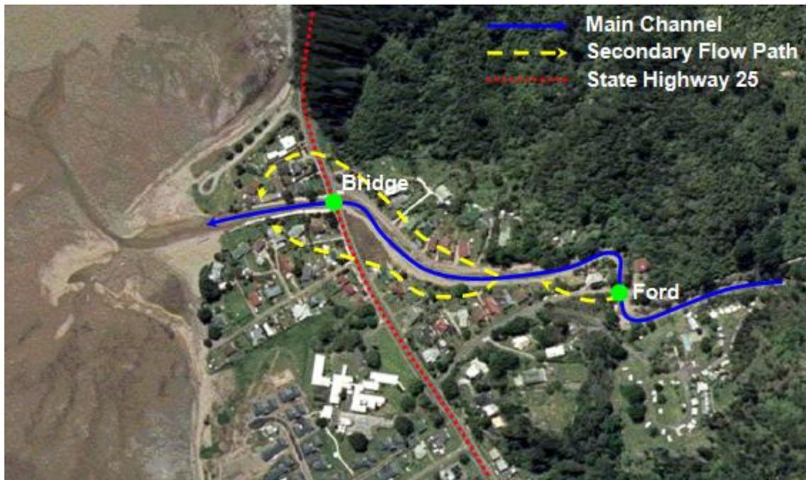
**Figure 6** Predominant flooding mechanism at Tararu
