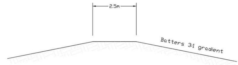
Typical Earth Bank Cross Section (not to Scale)
