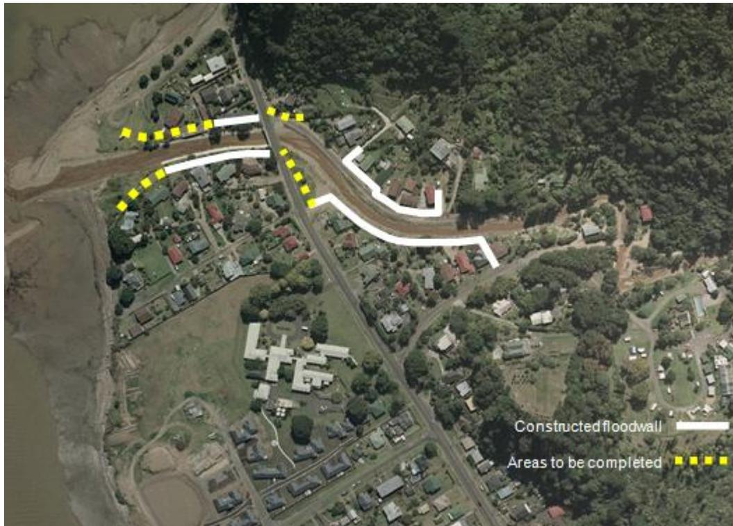
Figure 15 Staged construction of flood walls/stopbanks
