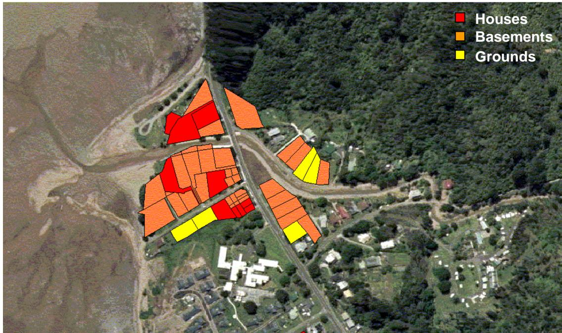
**Figure 8 Property damage within the Tararu community during the 'Weather Bomb'**
