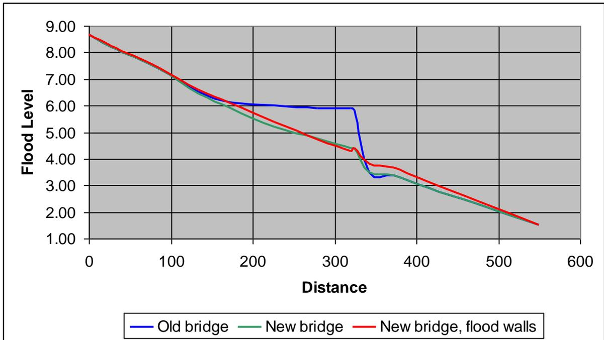
Figure 1 clearly shows the benefit of the new bridge profile. The new bridge allows the flow gradient to be constant whereas the old bridge caused a major restriction. At the bridge itself the flood has been lowered from RL5.81m to RL4.40m (1.41m). The installation of the flood walls have no detrimental impact.
