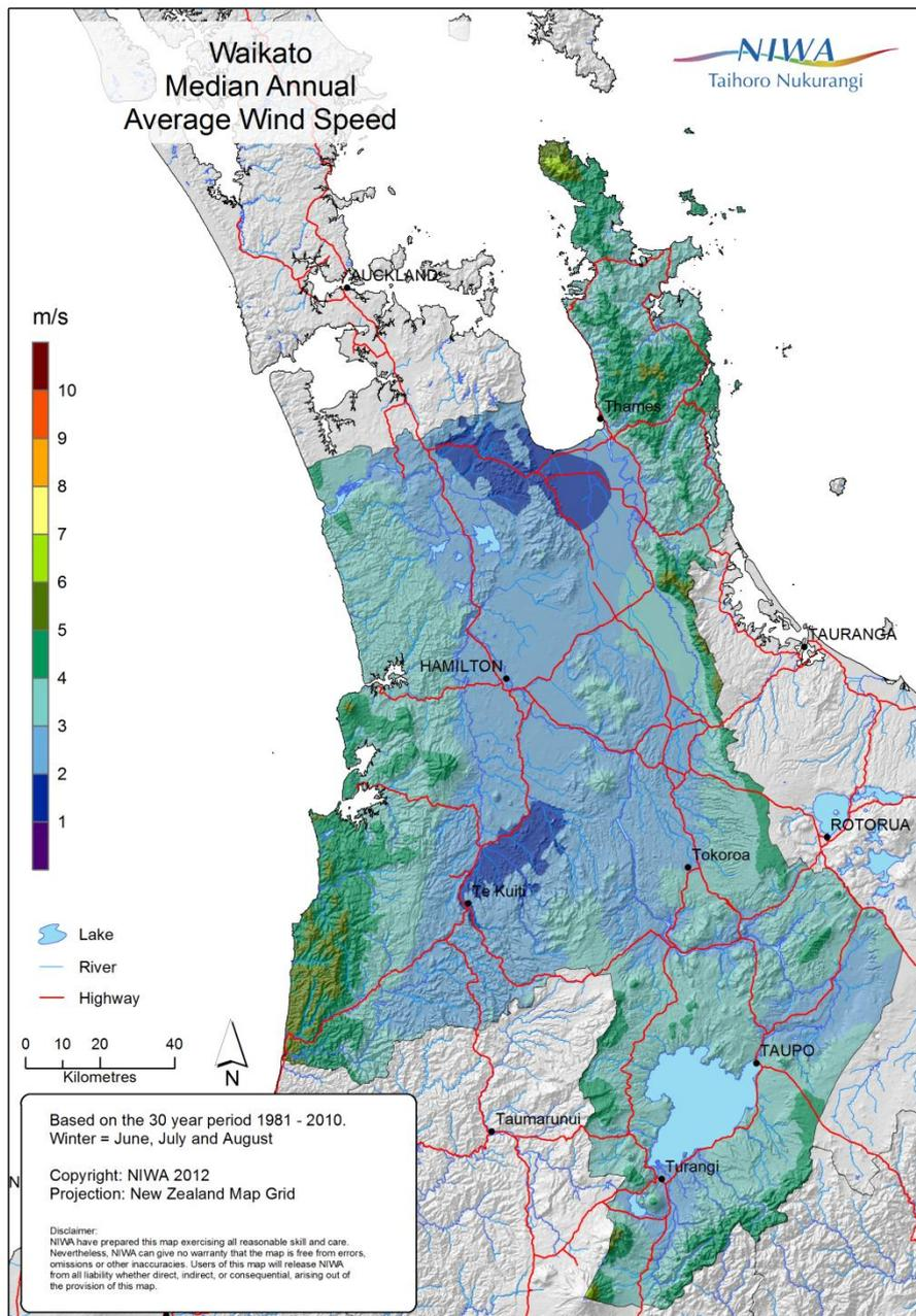
**Figure 5: Waikato Median Annual Wind Speed (based on data from the period 1981-2010)**
