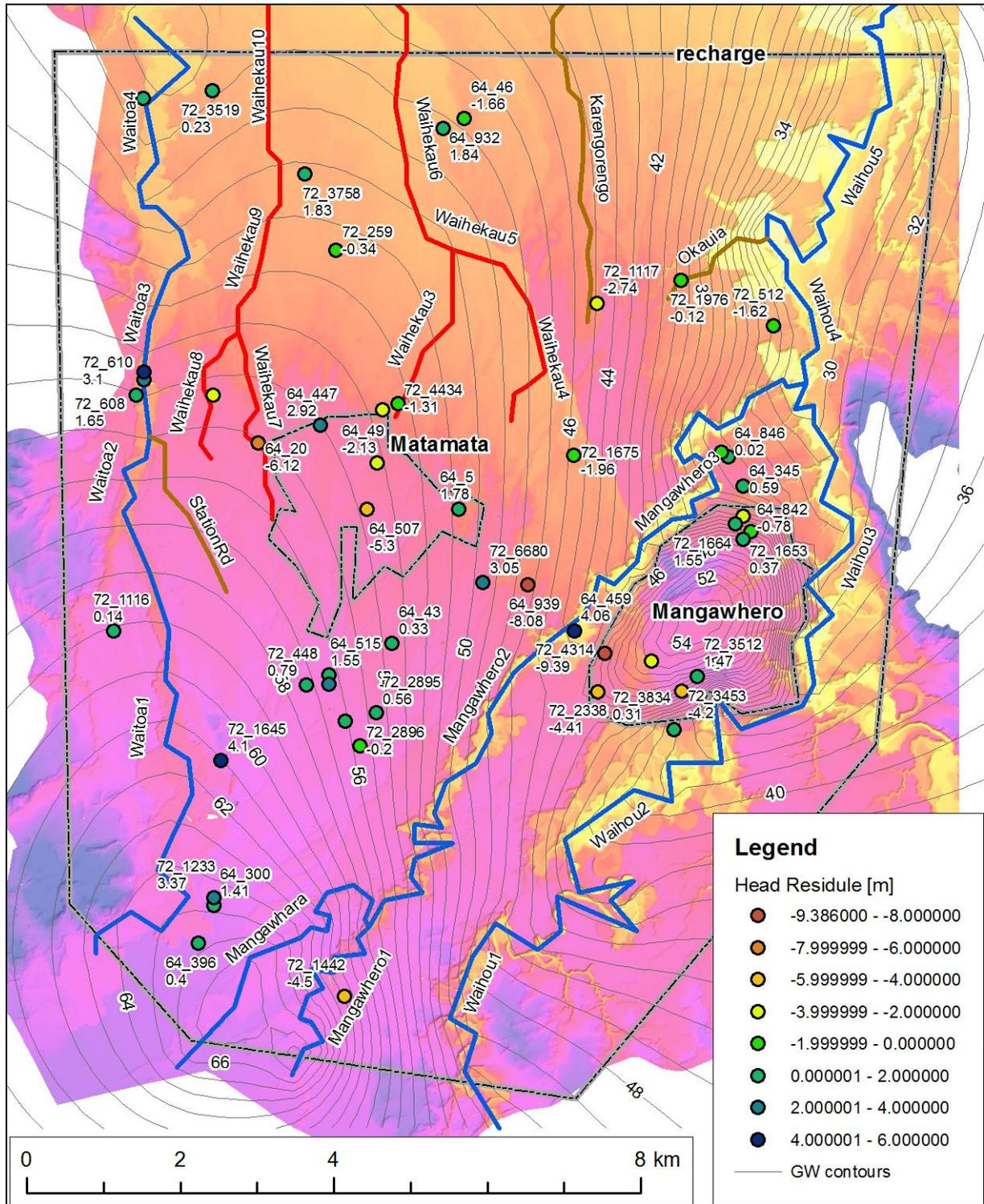
Figure 6 Base scenario calibration without pumping, showing groundwater head contours and head residuals between observed and simulated values.
