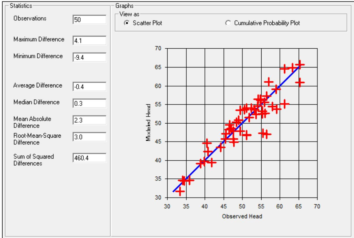
Figure 7 Base scenario calibration statistics and scatter plot of observed and simulated heads. Scatter of residues along the one-to-one line reveals that the calibration is unbiased, with a near constant variance.
