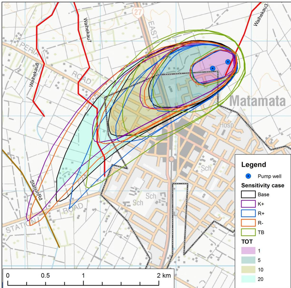
Figure 9 Capture zone delineations for all sensitivity analysis scenarios (Table 6), each showing 1-, 5-, 10-, and 20-year isochrones. The filled polygons show the median PZs.
