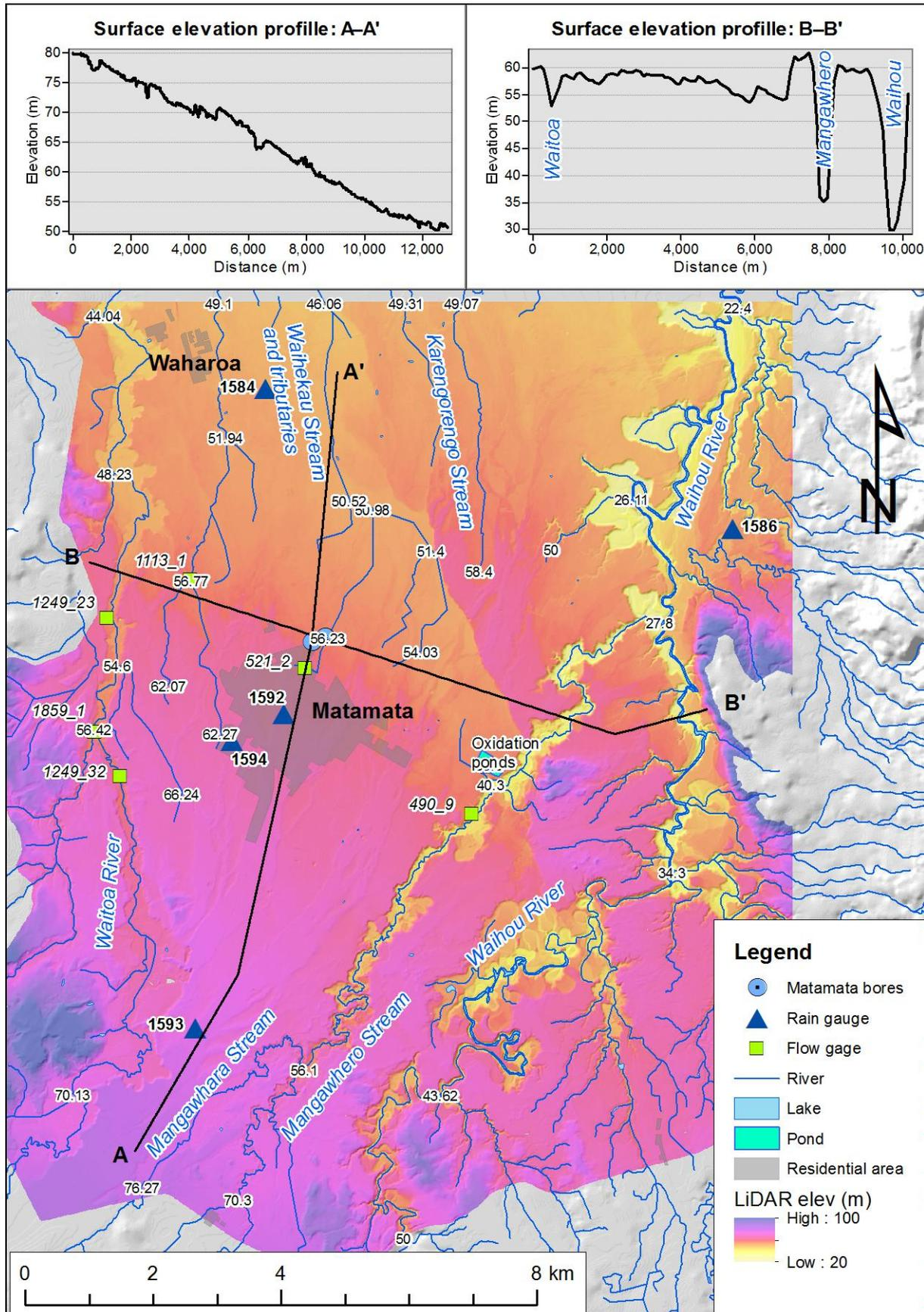
Figure 3 Map of hydrology and surface elevation from LiDAR and two elevation profiles which intersect the Matamata supply wells. Elevations of surface water features from LiDAR data are labelled. Bold labels are climate station agent numbers (Table 1), and italics labels are flow gauge identifiers (Table 2).
