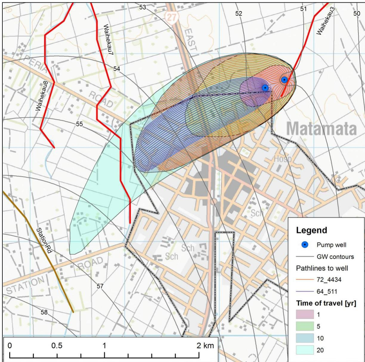
Figure 8 Flow pathlines with 10-year travel time to Tawari Street groundwater wells, based on a pumping rate of 60 m<sup>3</sup>/hr (total 120 m<sup>3</sup>/hr). PZ delineations are shown for 1-, 5-, 10-, and 20-year isochrones. This model is the calibrated Base scenario.
