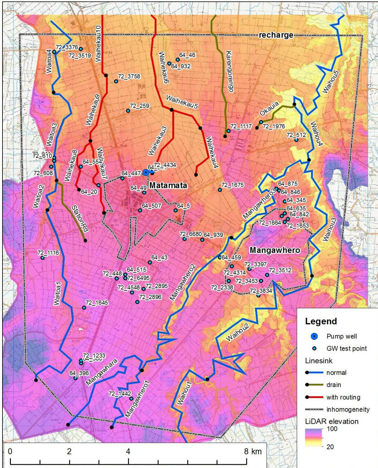
Figure 5 GFLOW model for the Matamata region, showing different labelled analytic elements. The starting locations for each line-sink are shown with a black dot, and have properties listed in Table 4. Three inhomogeneity zones for recharge, Matamata residential area, and Mangawhero, are shown. Labelled GW test points show boreholes that have groundwater elevations, and were used for the calibration process.
