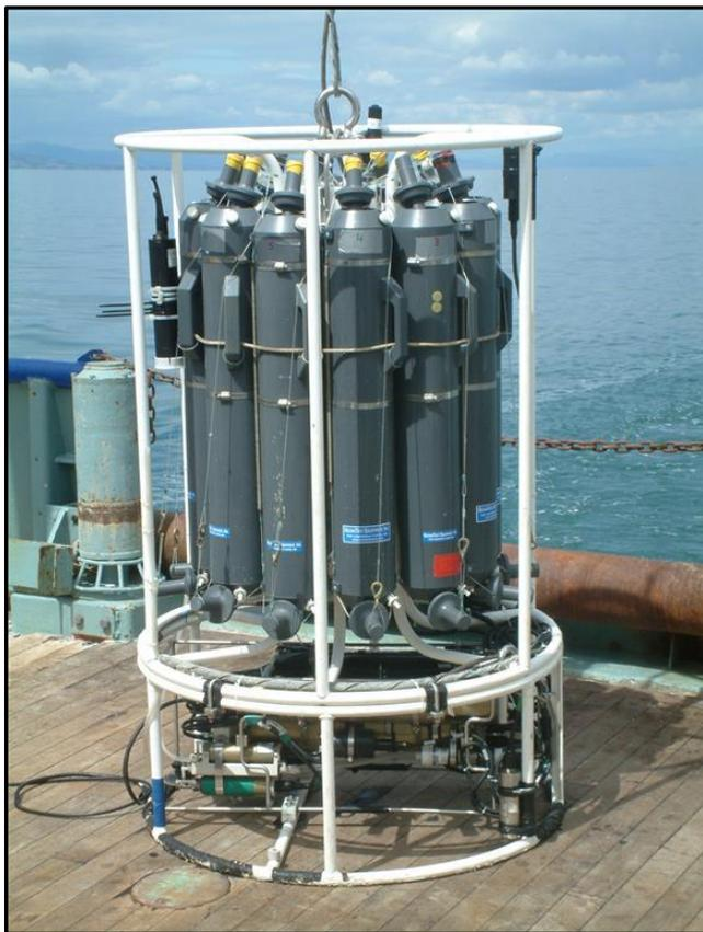
**Figure 10-3: The conductivity–temperature–depth (CTD) instrument about to be deployed from the stern of NIWA RV *Kaharoa*.** It is lowered through the water and used to sample parameters including temperature, salinity, oxygen and light, at various depths in the water column, using the electronic sensors at the base of the package. The bottles can be shut at specified depths to capture water for later laboratory analysis for nutrients.
