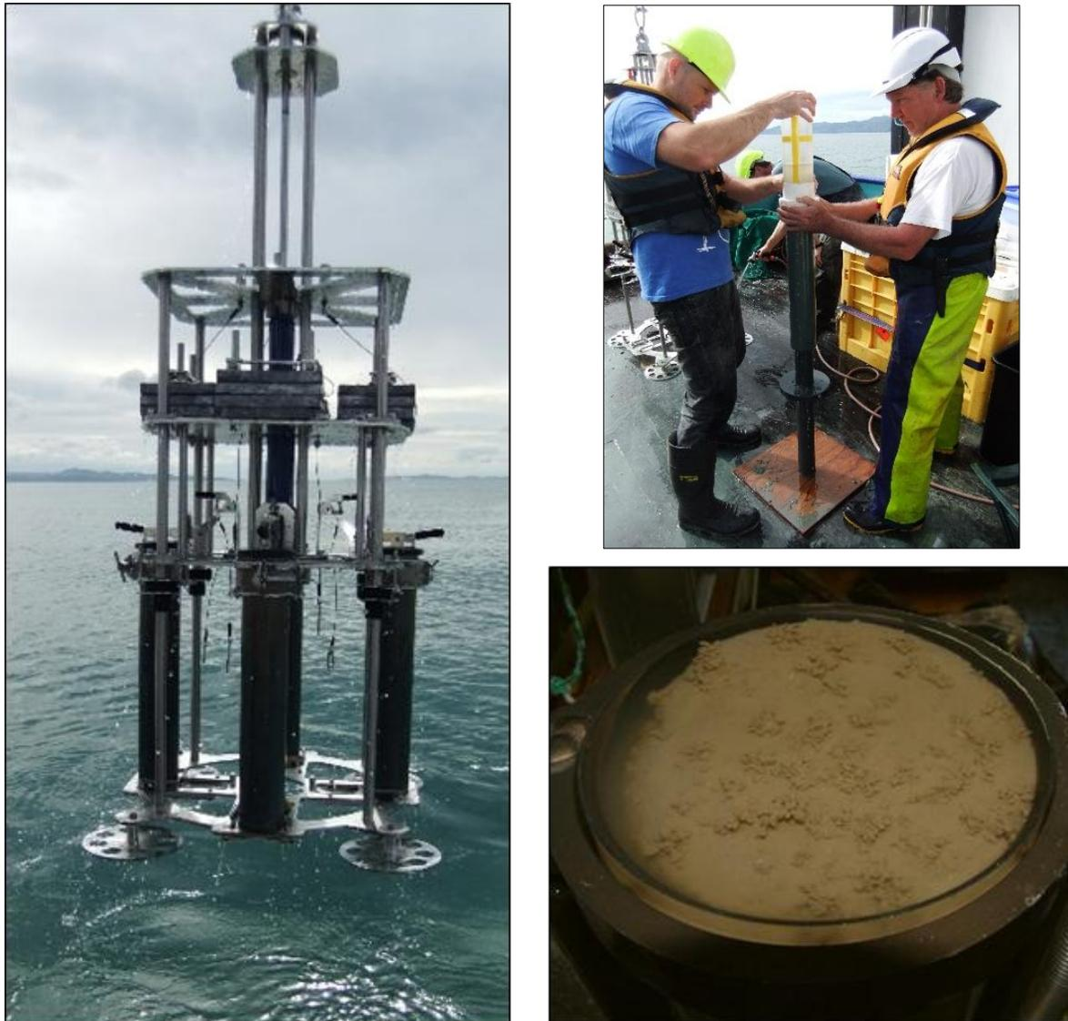
**Figure 9-2: Sediment sampling in the Firth.** Multi-coring device retrieved onto the ship with sediment cores. Upper right: sediments being extruded to incubation cores. Lower right: core surface showing intact surface faunal structure.
