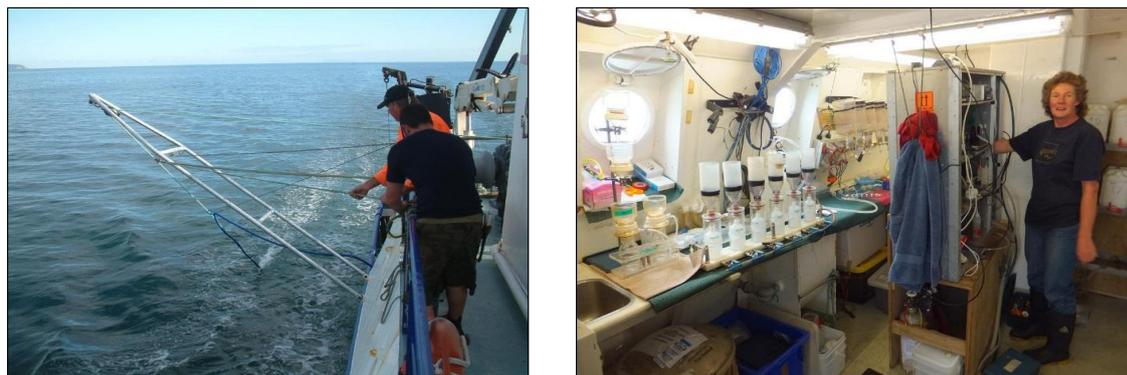
**Figure 8-1: Underway sampling and shipboard laboratory.** (Left) Water was pumped aboard via a towfish and hose assembly, and (right) sent to the shipboard LiCor  $\text{CO}_2$  analyser and filtration laboratory.
