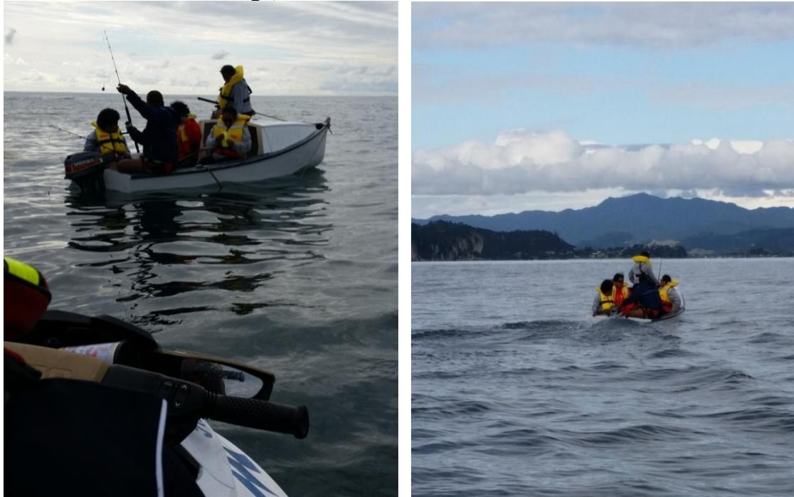
Photo 1 & 2: This vessel was over two nautical miles from shore, overloaded, with insufficient PFDs for the number of people aboard. Of the PFDs put on, two were a good fit and two were a poor fit, with straps unable to be fastened. The picture on the right shows the lack of freeboard when this vessel was underway.
