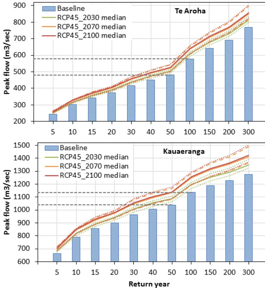
Figure 14 Peak flows (m<sup>3</sup>/sec) and corresponding ARI values for baseline and future climate change scenarios for the Waihou River, (station at Te Aroha) (top figure) and the Kauaeranga River (station at Kauaeranga station) (bottom figure) for 2030, 2070 and 2100 using RCP4.5.
