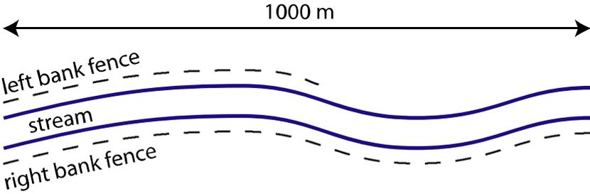
**Figure 2:** A stylised example of a stream reach that illustrates the concepts of stream length, bank length, and fencing configuration (source: Storey, 2010, p.8).
