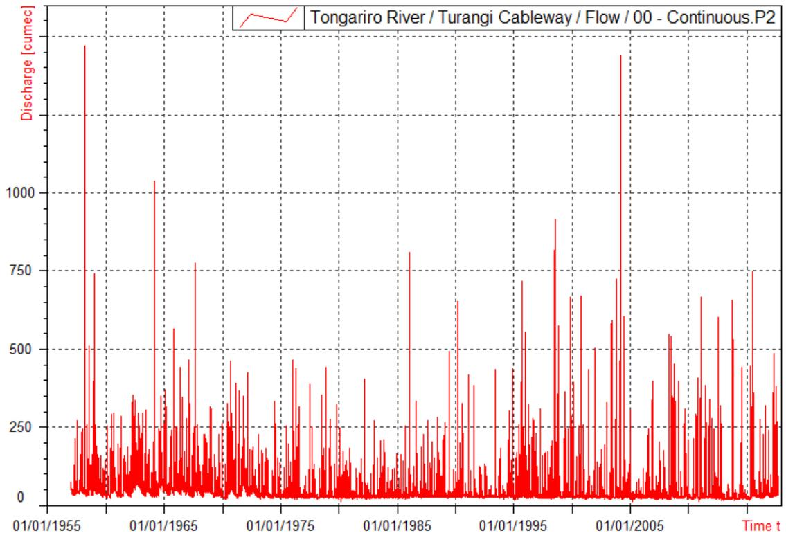
**Figure 4 Flow record for the Tongariro River at Turangi Cableway.**
