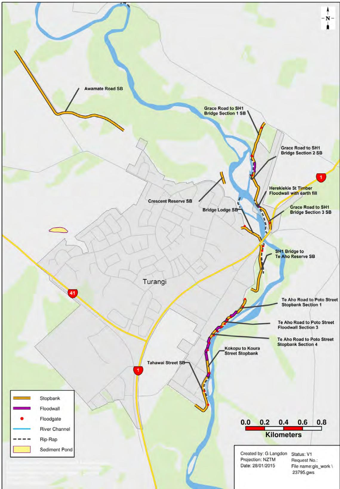
Figure 1 Flood protection scheme assets along the Tongariro River at Turangi.
