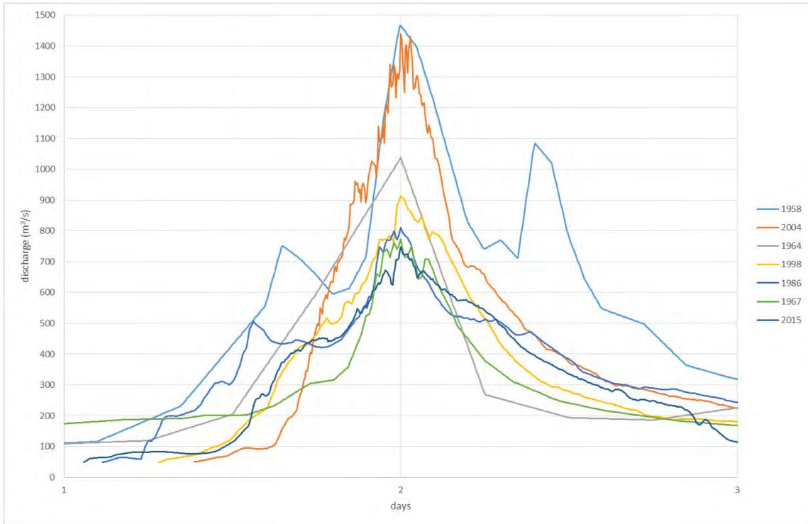
**Figure 5** Peak centered flood hydrographs for the 7 largest events on record for the Turangi Cableway (NIWA gauge).
