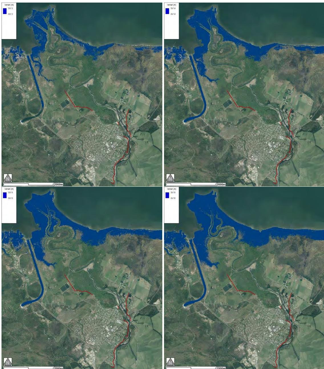
**Figure 7** Lake water level inundation on 2016 LIDAR surface at RL 357.2m, 357.4m, 357.6m and 357.8m.
