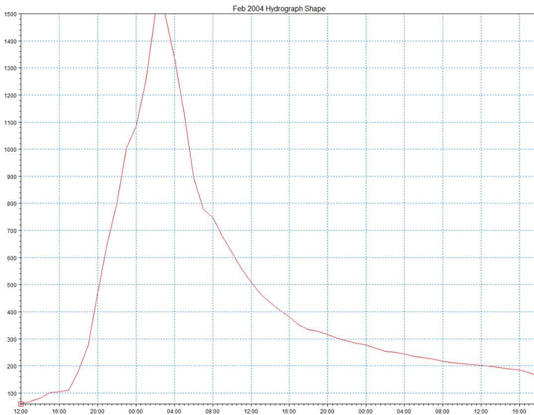
**Figure 6** Design hydrograph shape used in hydraulic modelling - derived from smoothed 2004 event data and adjusted in the vertical to required design discharge.
