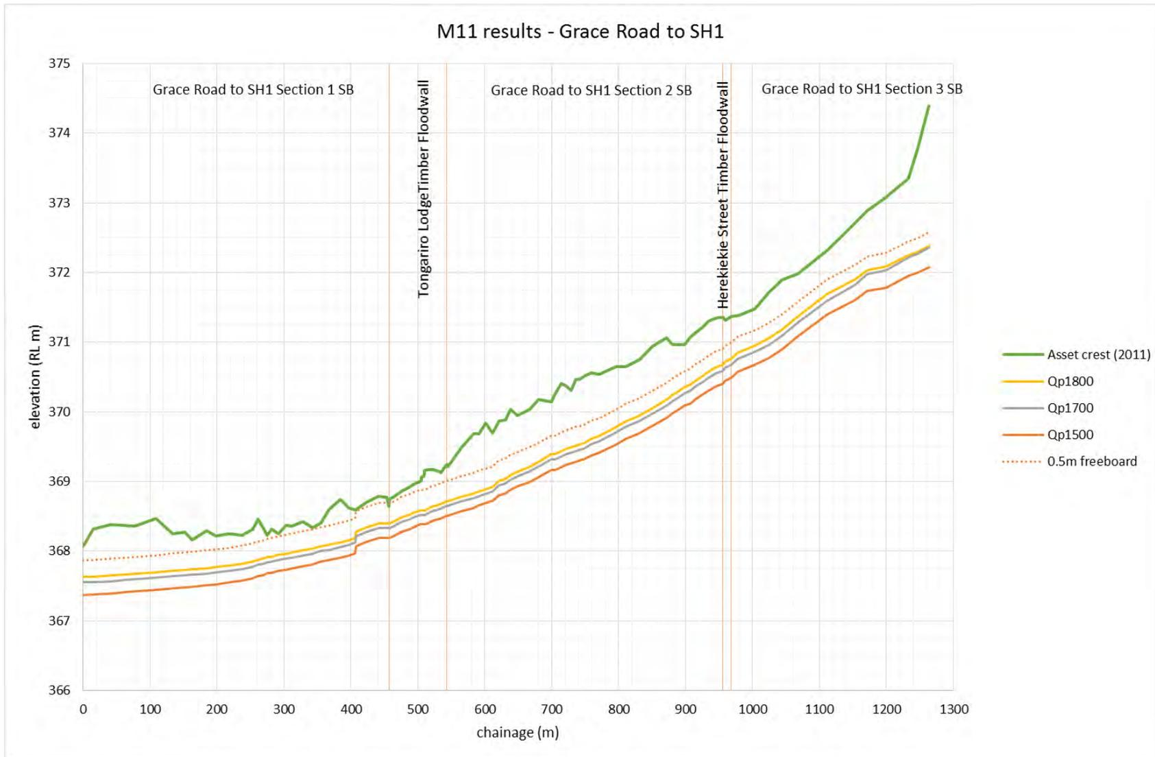
**Figure 10** MIKE11 modelled water levels for various discharges compared against right bank flood protection scheme assets between Grace Road and SH1.
