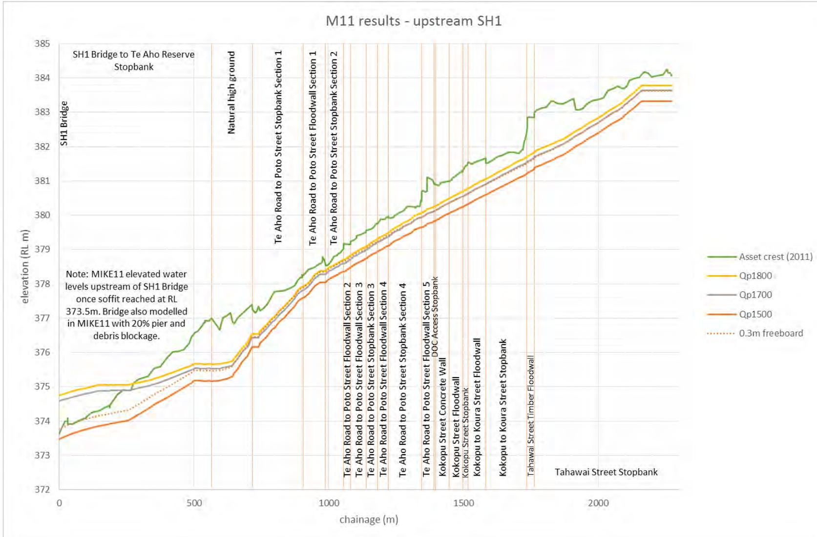
**Figure 9 MIKE11 modelled water levels for various discharges compared against left bank flood protection scheme assets upstream of SH1.**
