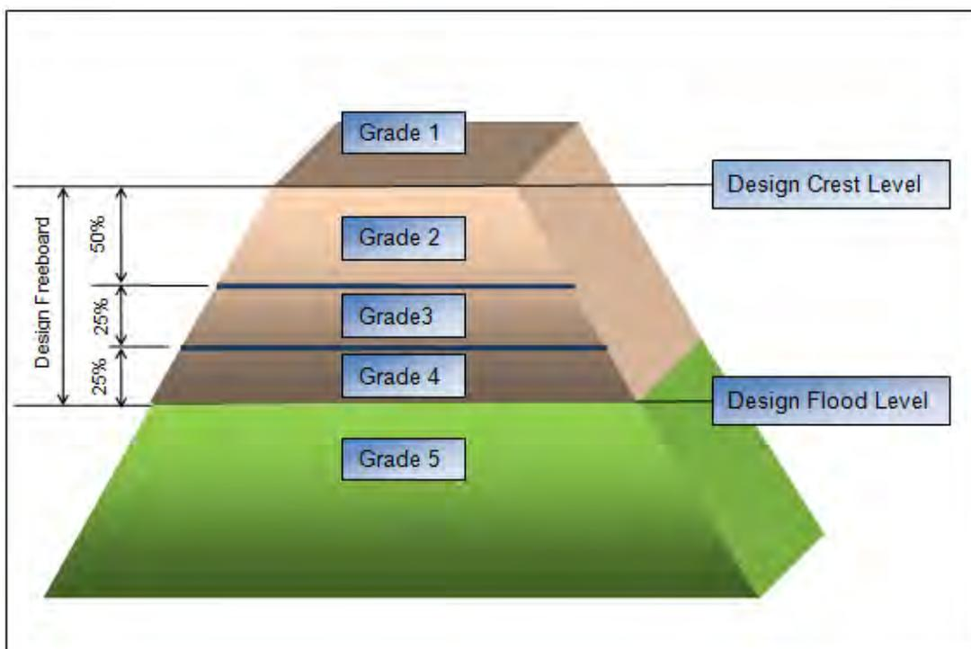
Figure 14 Diagrammatic representation of stopbank performance grades.
