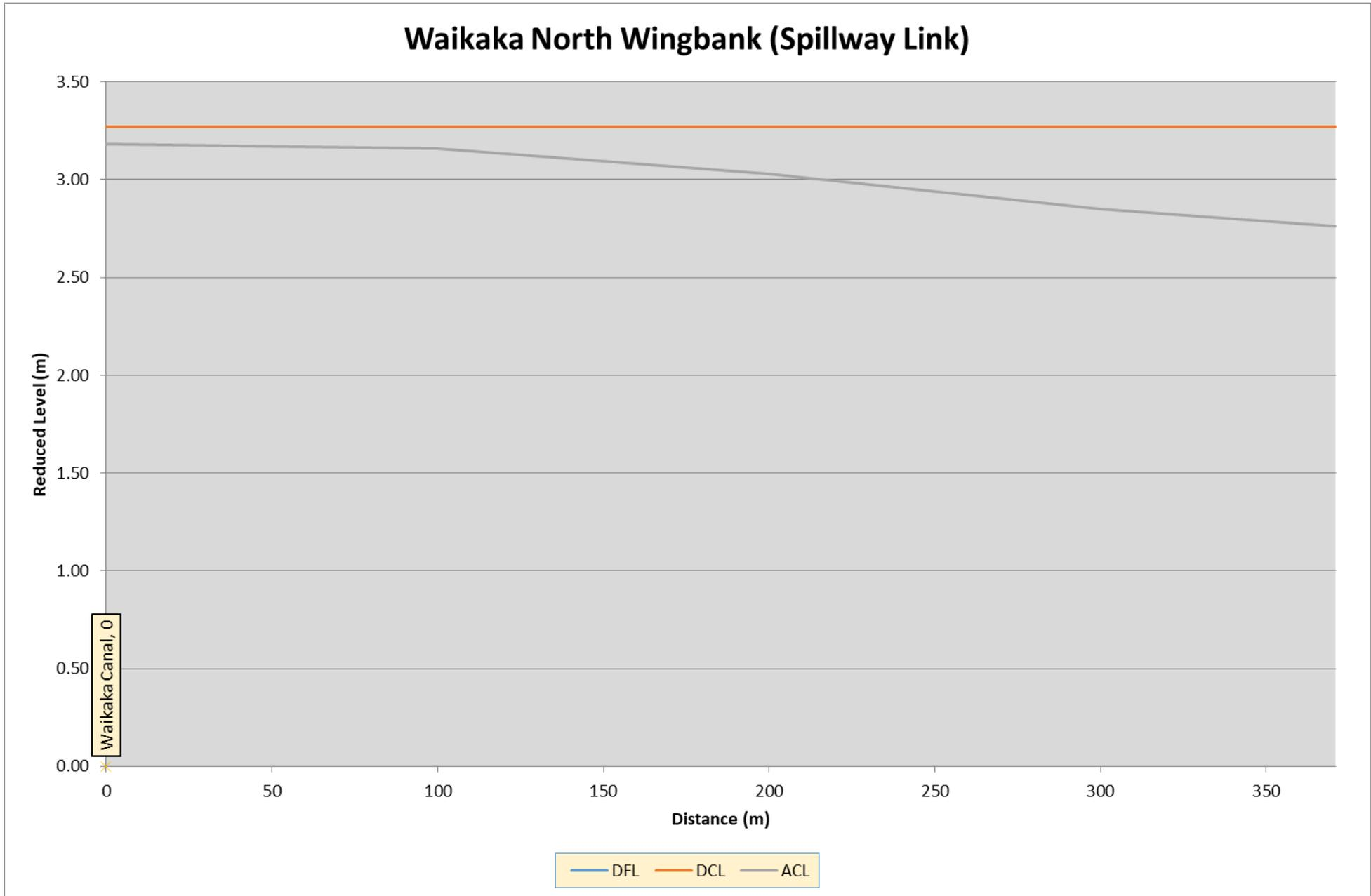
Figure 24: Waikaka North Wing Bank stopbank profile
