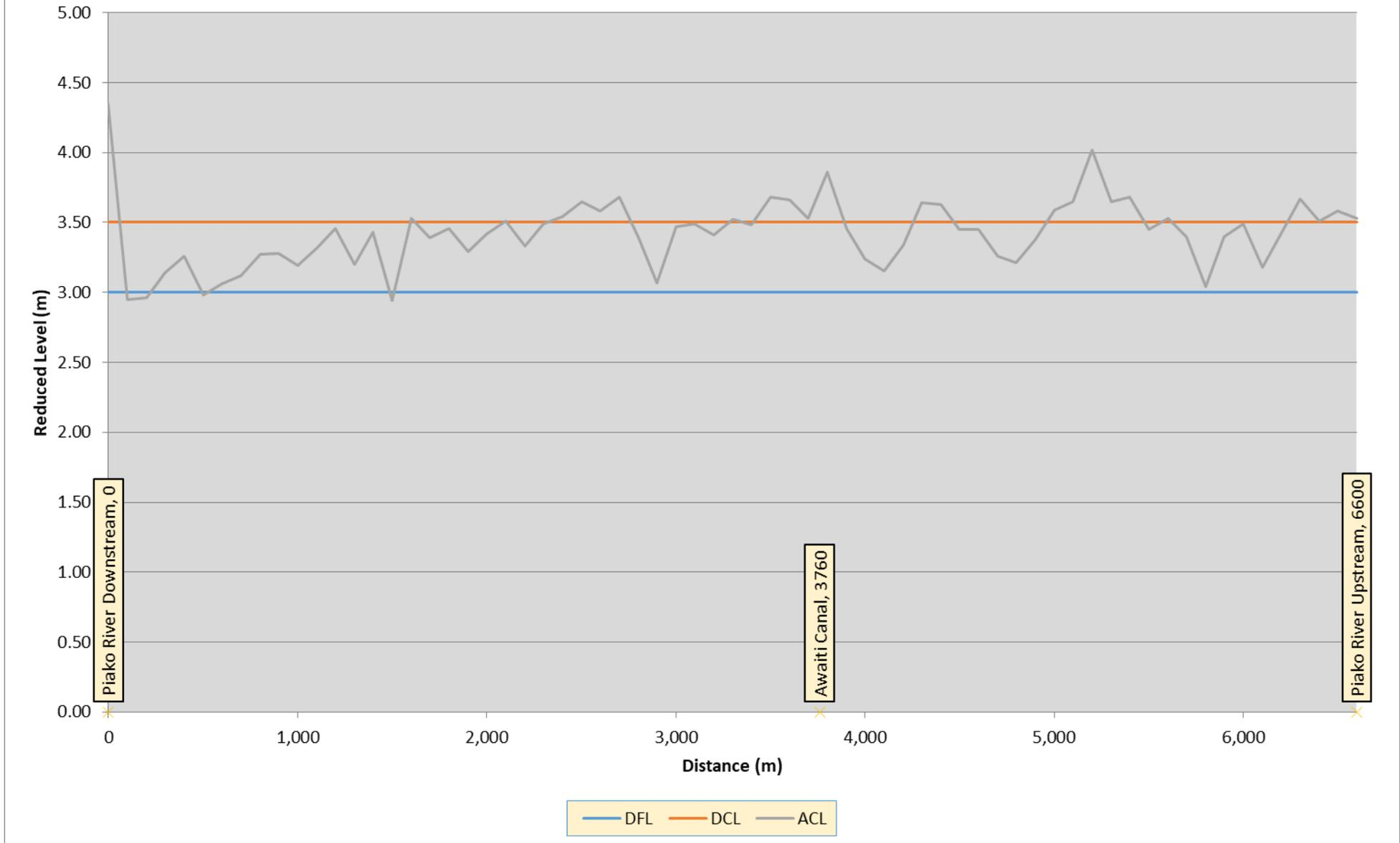
Figure 32: Kerepehi Loop left bank stopbank profile
