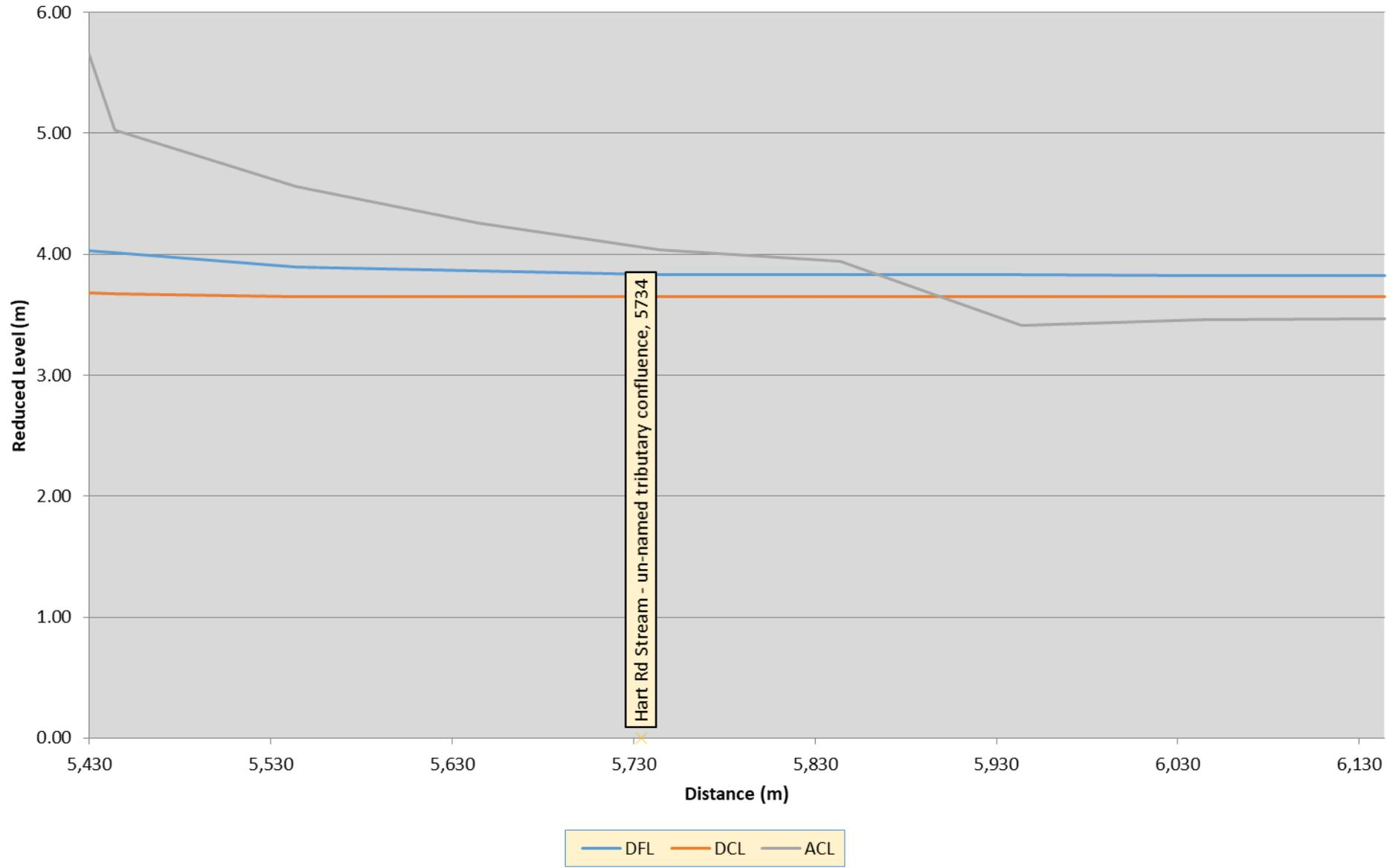
Figure 20: 2nd Emergency Ponding Zone - Hart Rd Stream right bank stopbank profile
