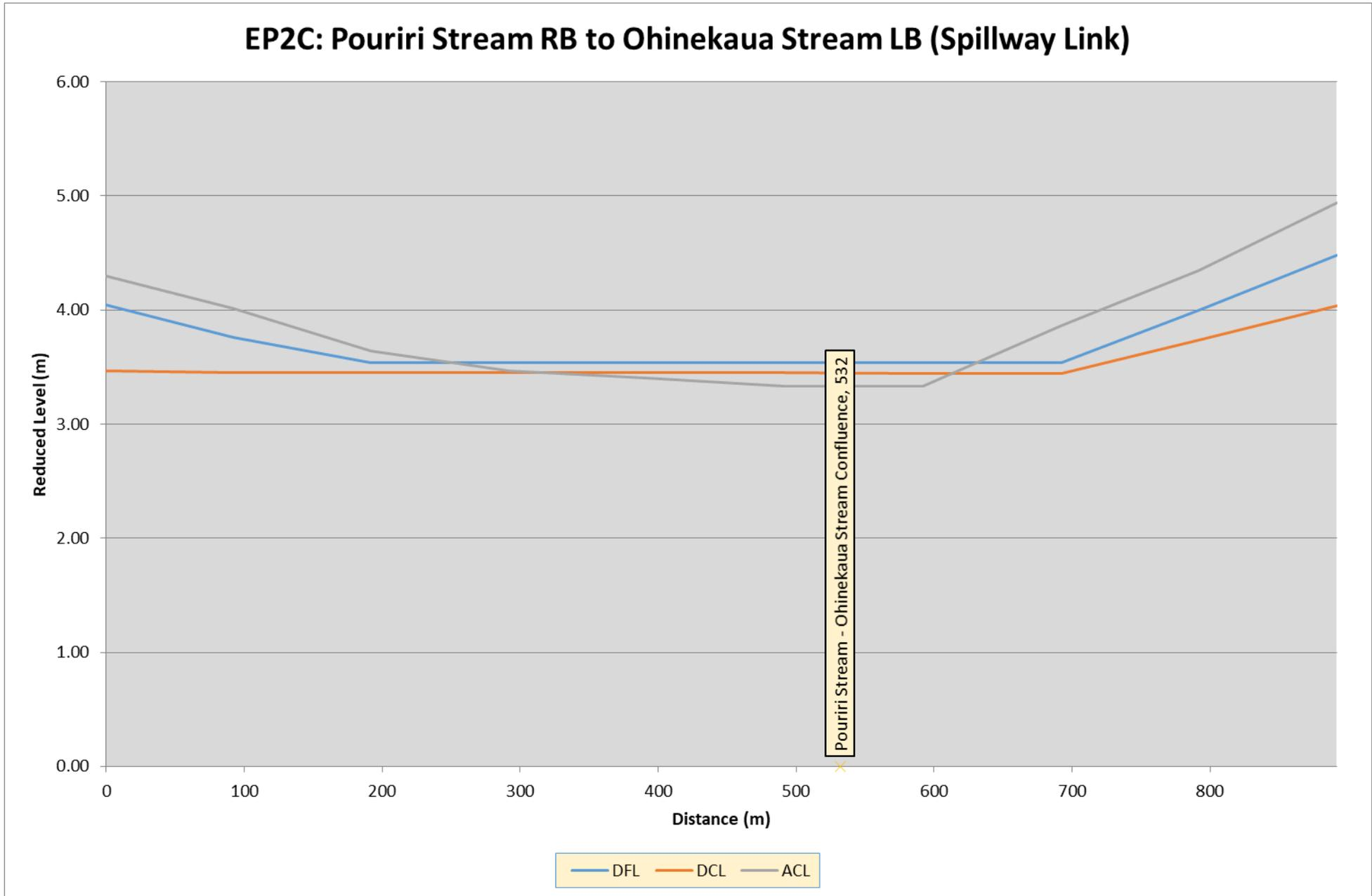
Figure 22: 2nd Emergency Ponding Zone - Pouriri Stream right bank to Ohinekaia Stream left bank stopbank profile
