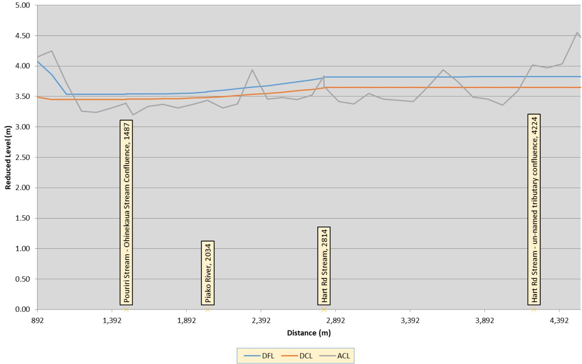
Figure 21: 2nd Emergency Ponding Zone - Ohinekaia Stream right bank to Hart Rd Stream left bank stopbank profile
