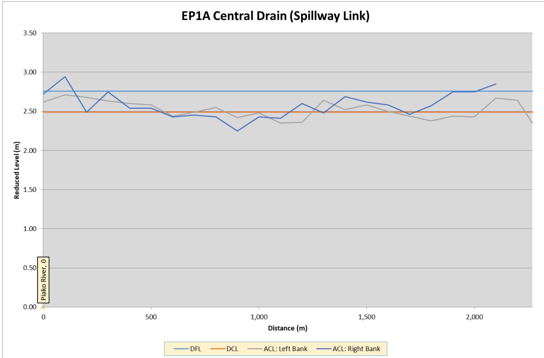
Figure 15: Central Drain stopbank profiles
