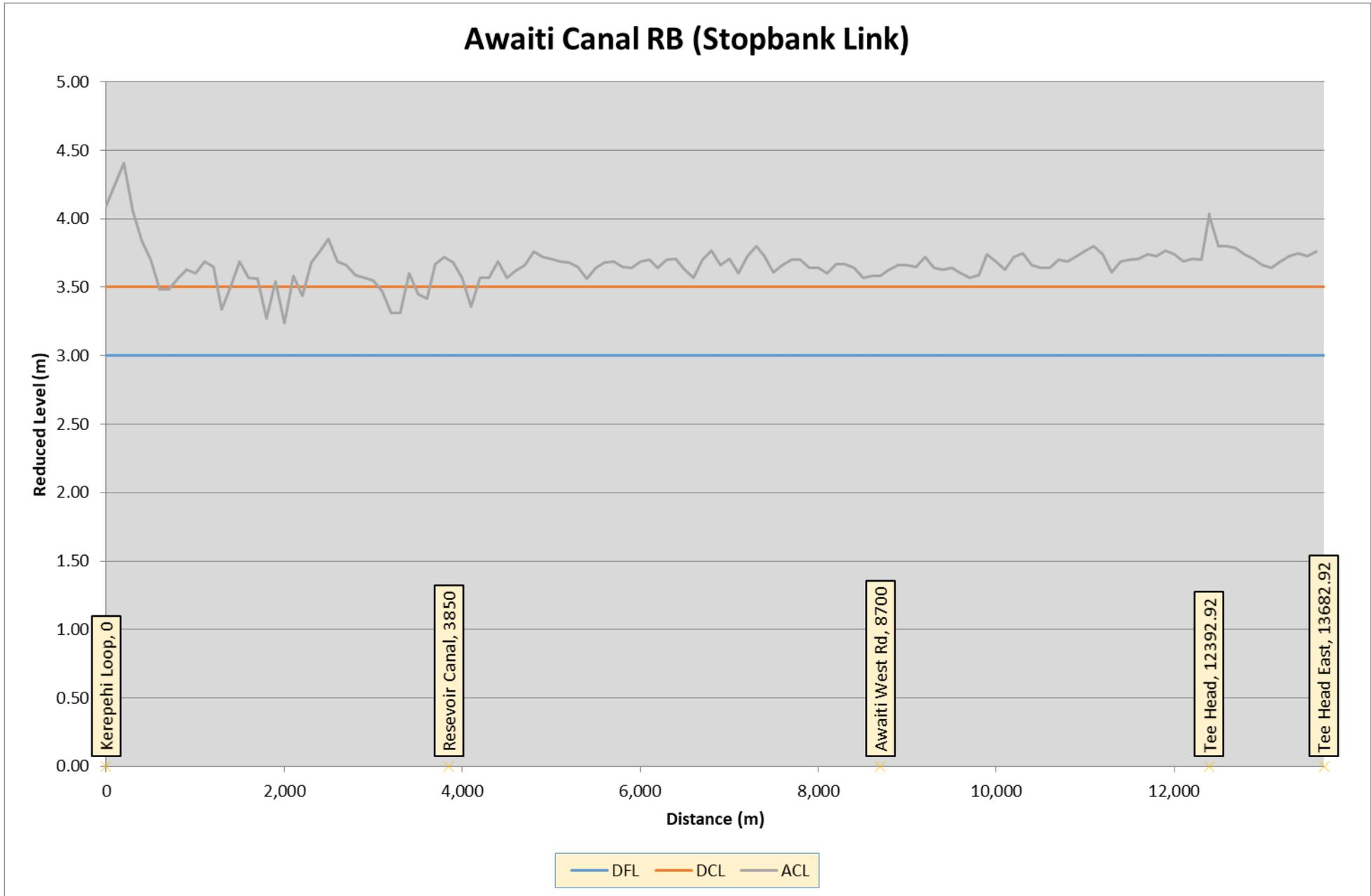
Figure 26: Awaiti Canal right bank stopbank profile
