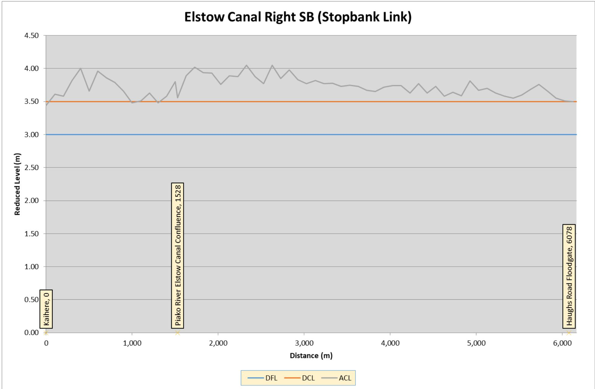
Figure 30: Elstow Canal right bank stopbank profile
