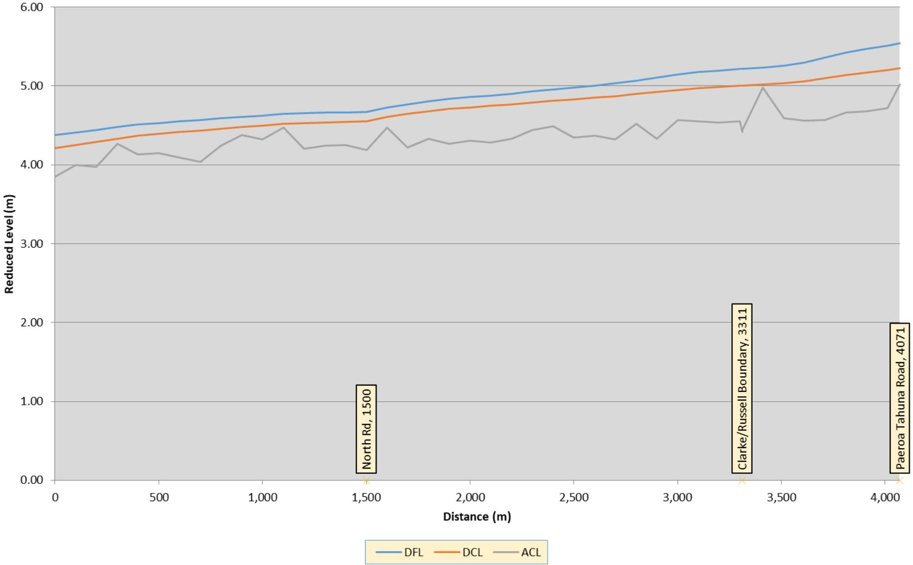
Figure 23: 2nd Emergency Ponding Zone – Waitoa River right bank Clarke to Paeroa Tahuna Rd stopbank profile
