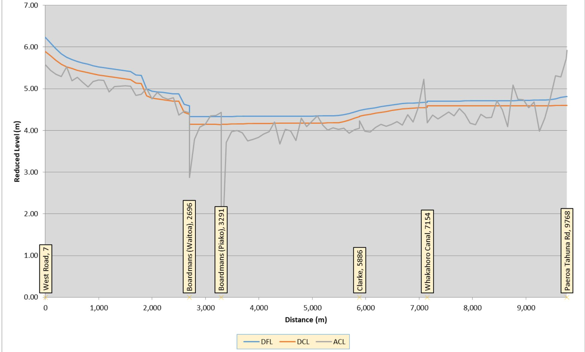
Figure 19: 2nd Emergency Ponding Zone - West Rd to Paeroa Tahuna Rd stopbank profile
