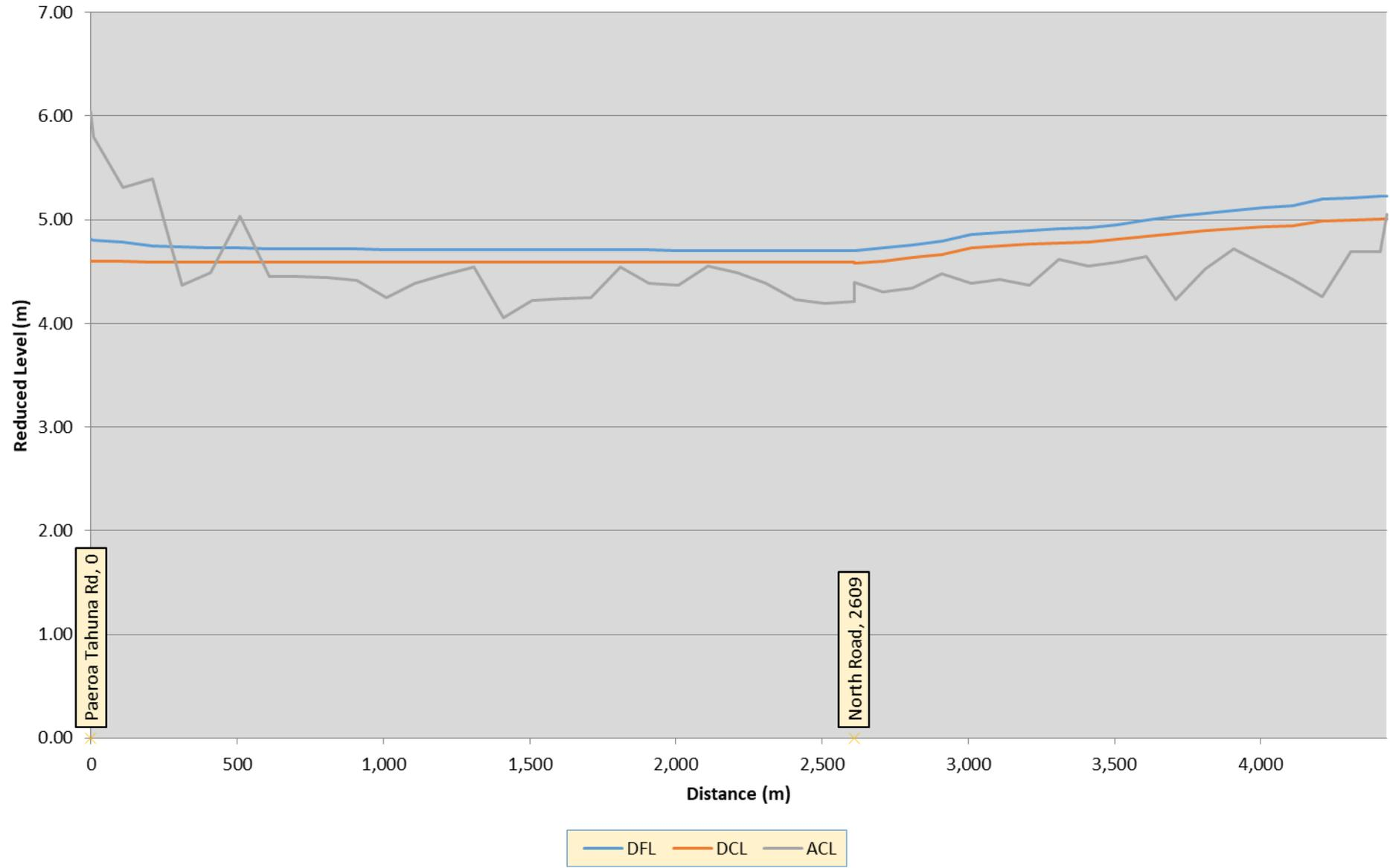
Figure 18: 2nd Emergency Ponding Zone - Paeroa Tahuna Rd to Chatfield Cooksons stopbank profile
