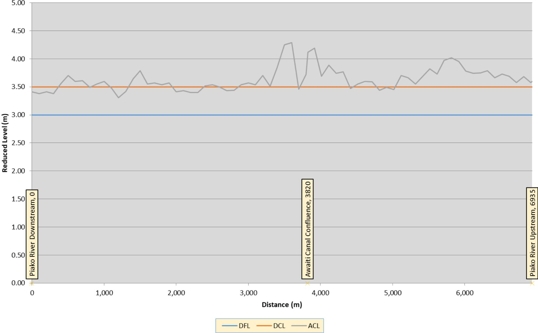
Figure 33: Kerepehi Loop right bank stopbank profile
