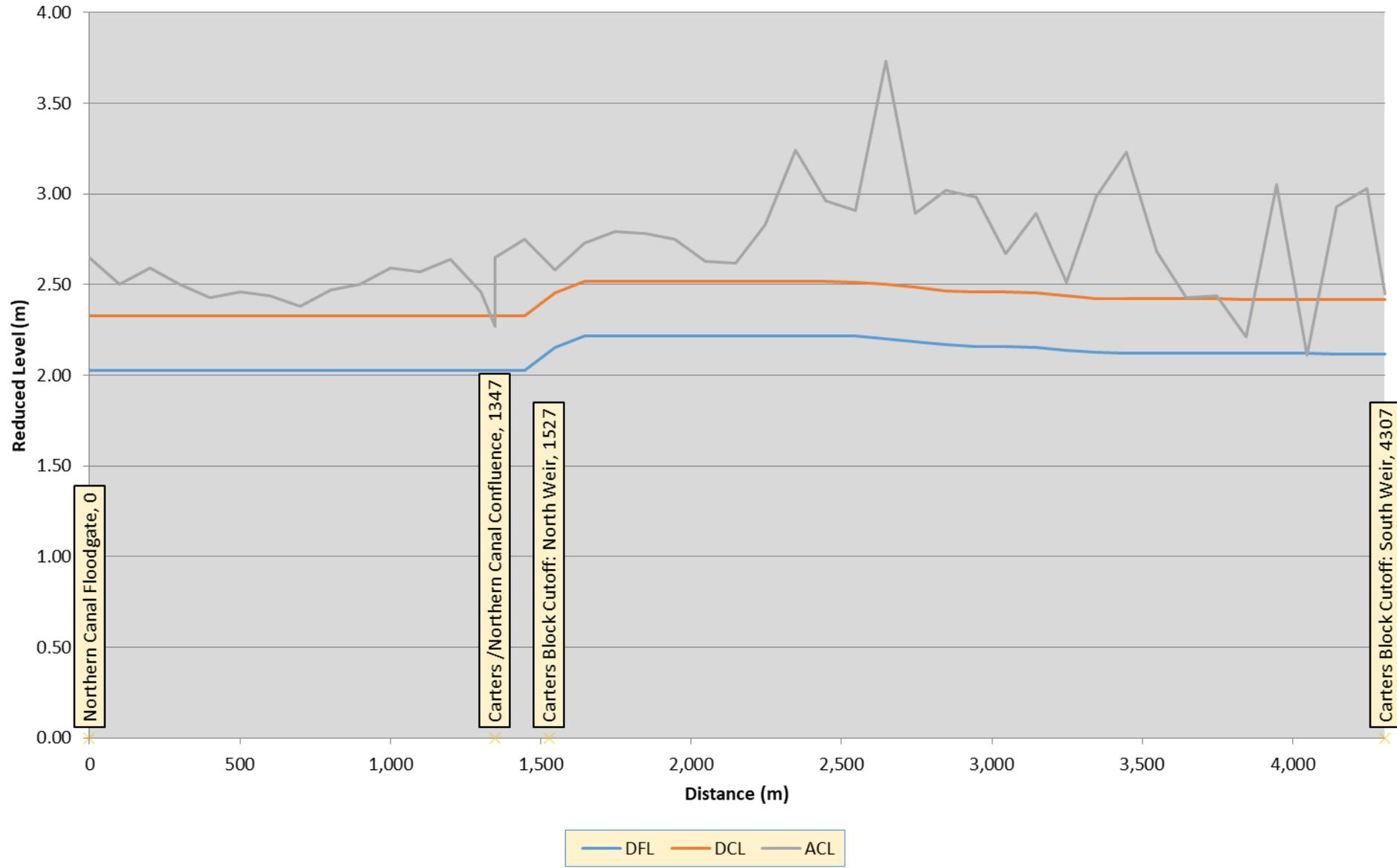
Figure 28: Carters Block Cut-off/Northern Canal right bank stopbank profile
