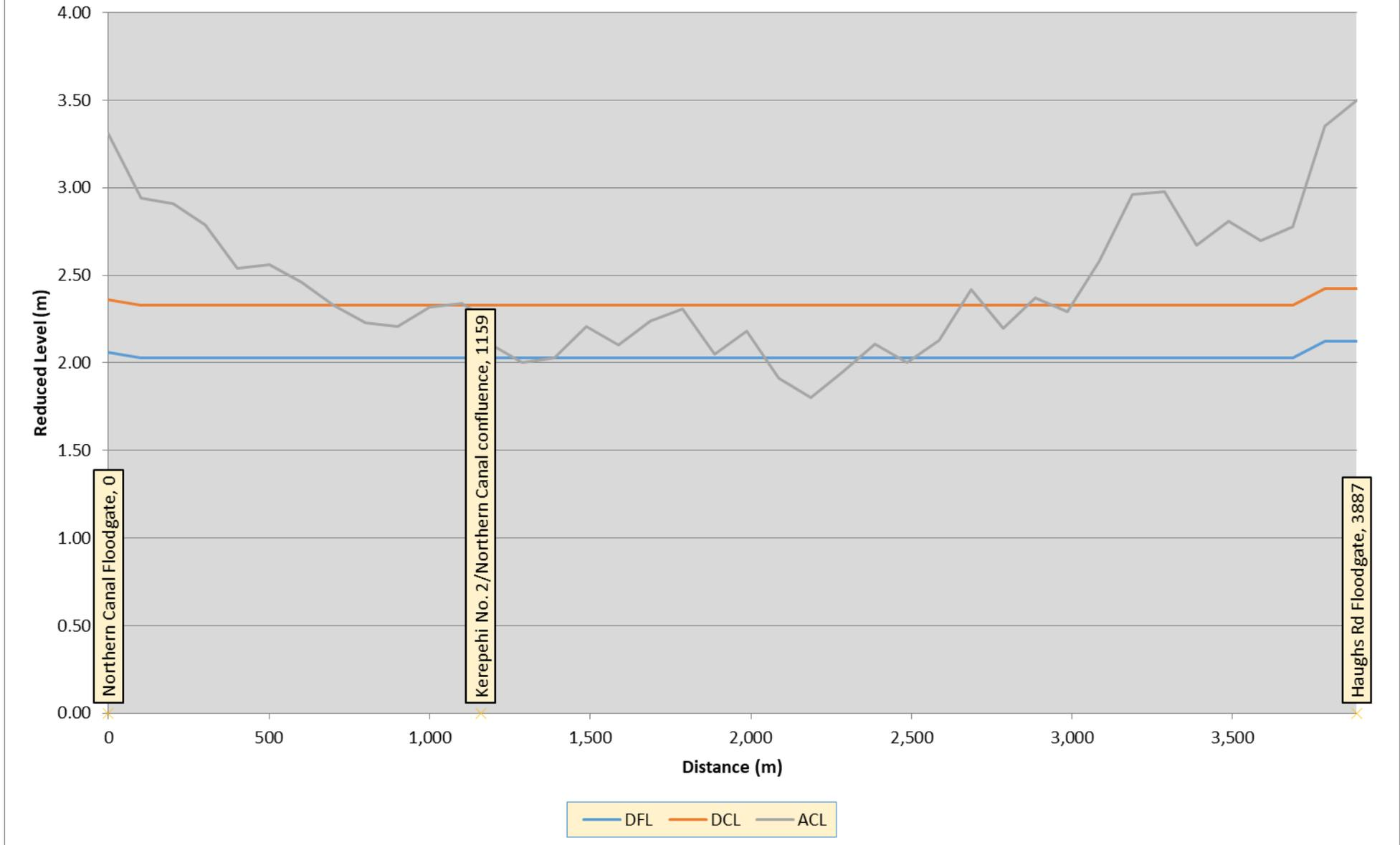
Figure 29: Kerepehi No 2 Cutoff and Northern Canal left bank stopbank profile
