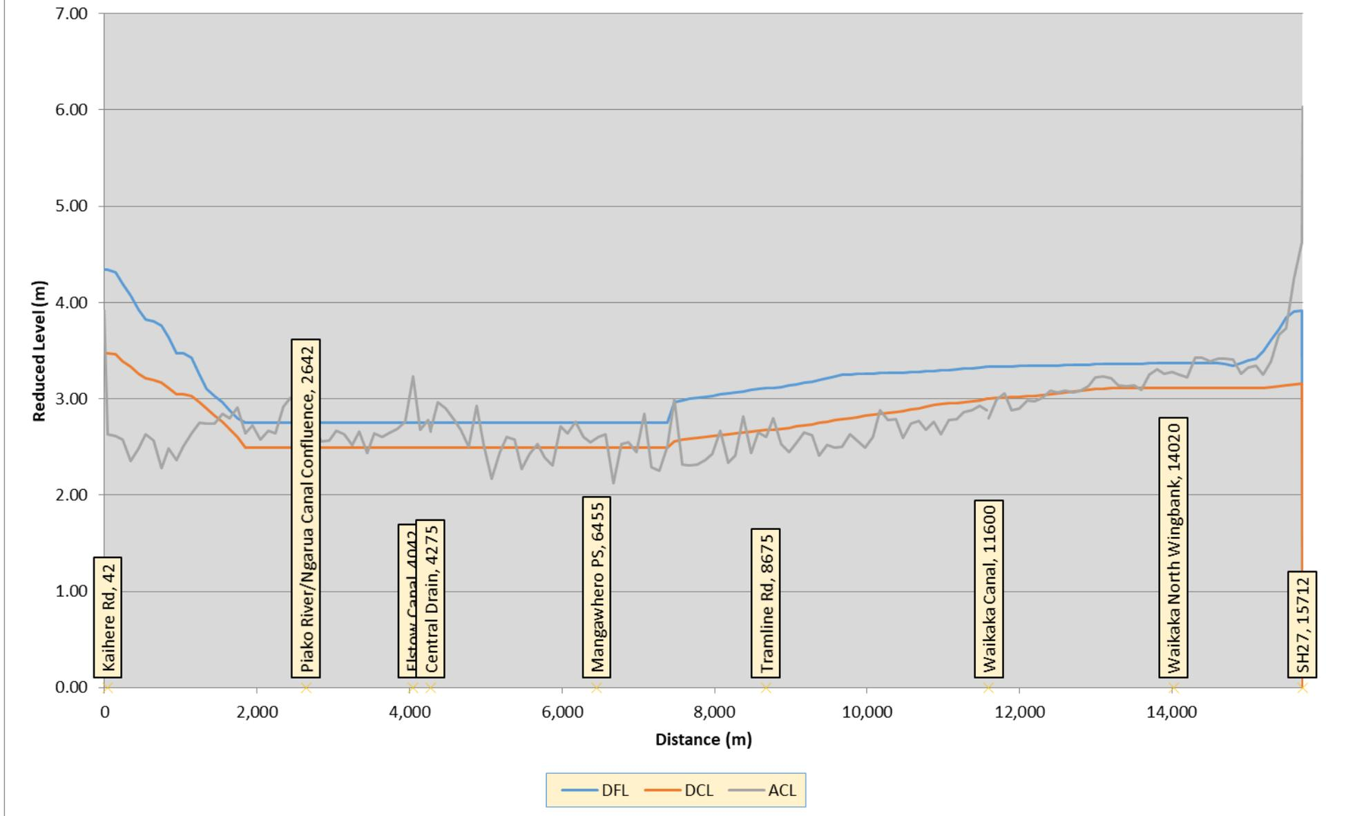
Figure 16: 1st Emergency Ponding Zone - Kaihere Rd to State Highway 27 stopbank profile
