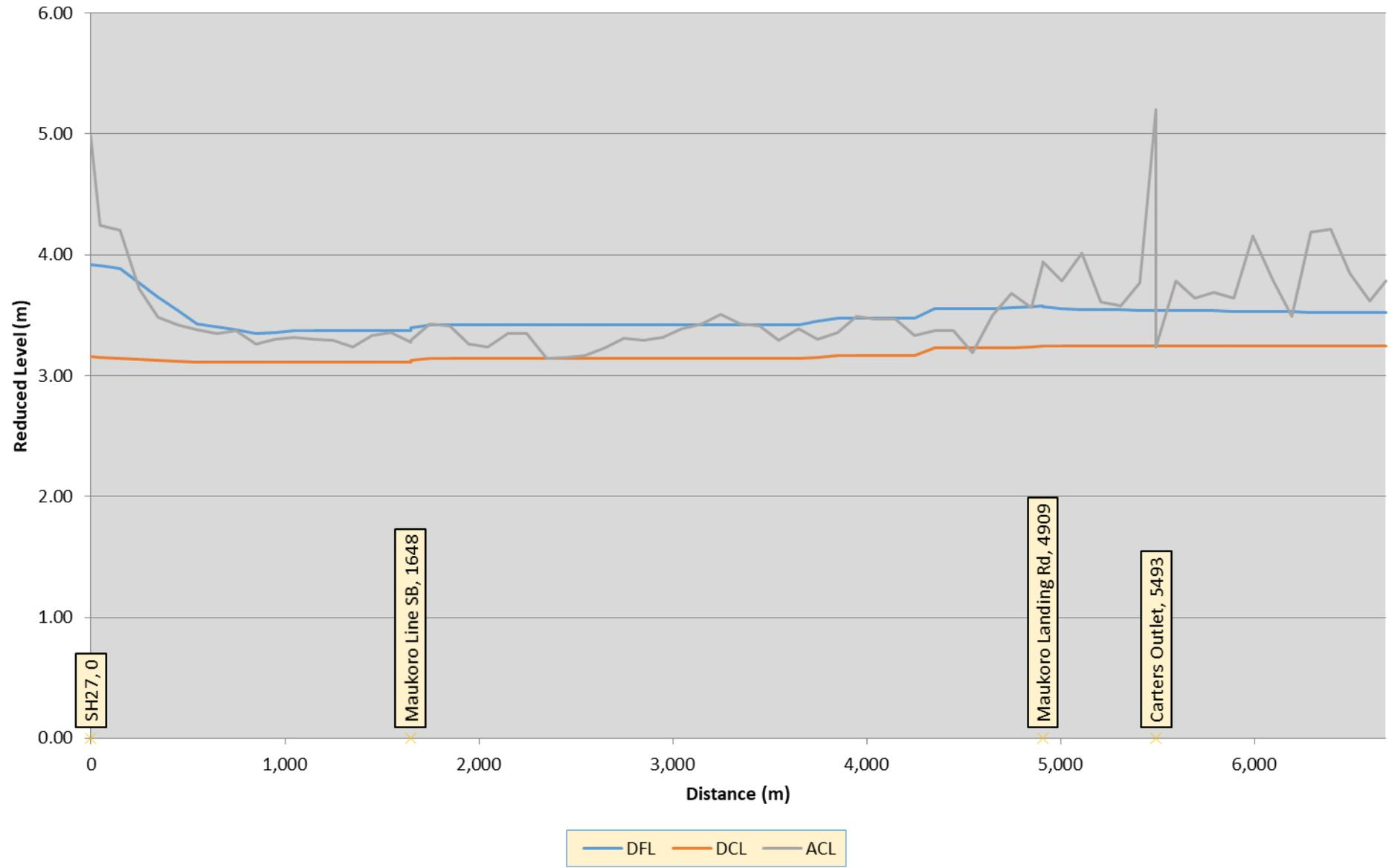
Figure 17: 1st Emergency Ponding Zone - State Highway 27 to Carters Outlet stopbank profile
