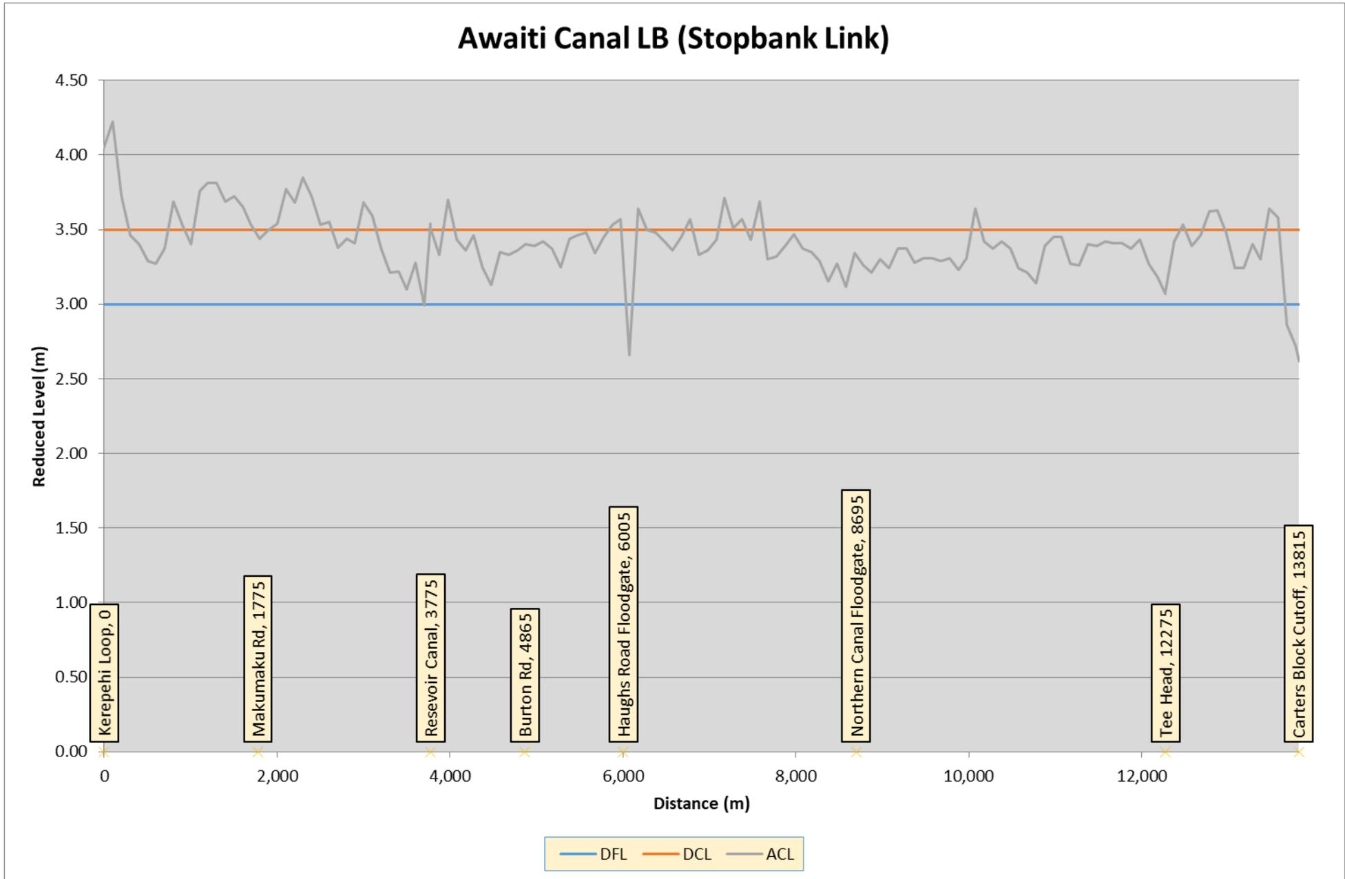
Figure 25: Awaiti Canal left bank stopbank profile
