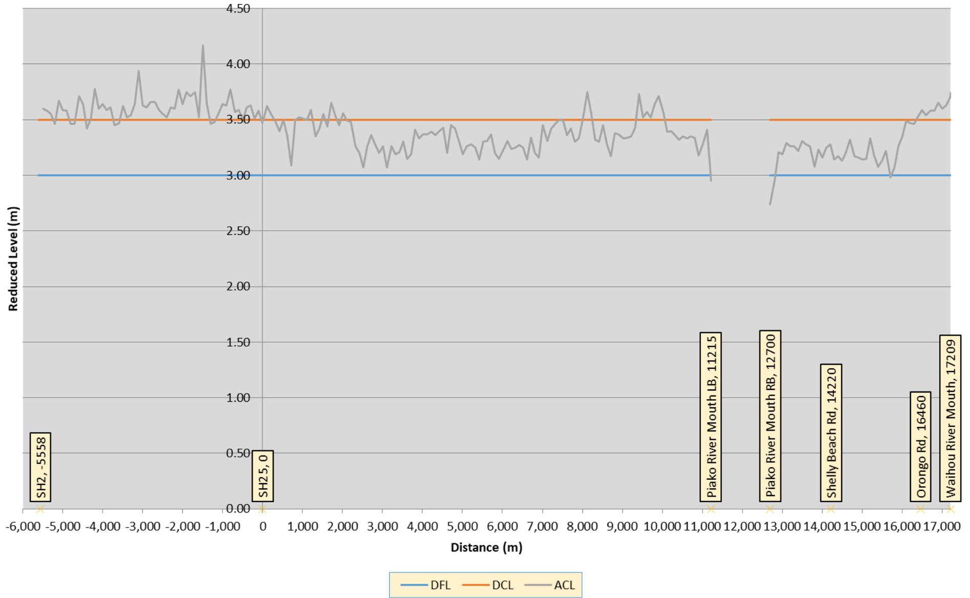
Figure 31: Maukoro Canal right bank and Piako Foreshore Stopbank Profile
