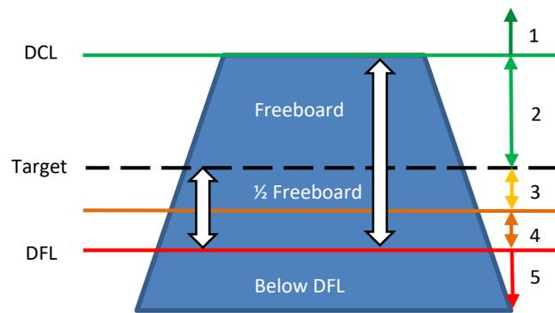
**Figure 3 Condition Assessments for Stopbanks**
