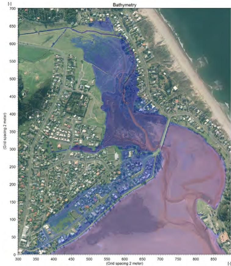
Figure 10 Tidal inundation during design + 0.8m sea level rise
