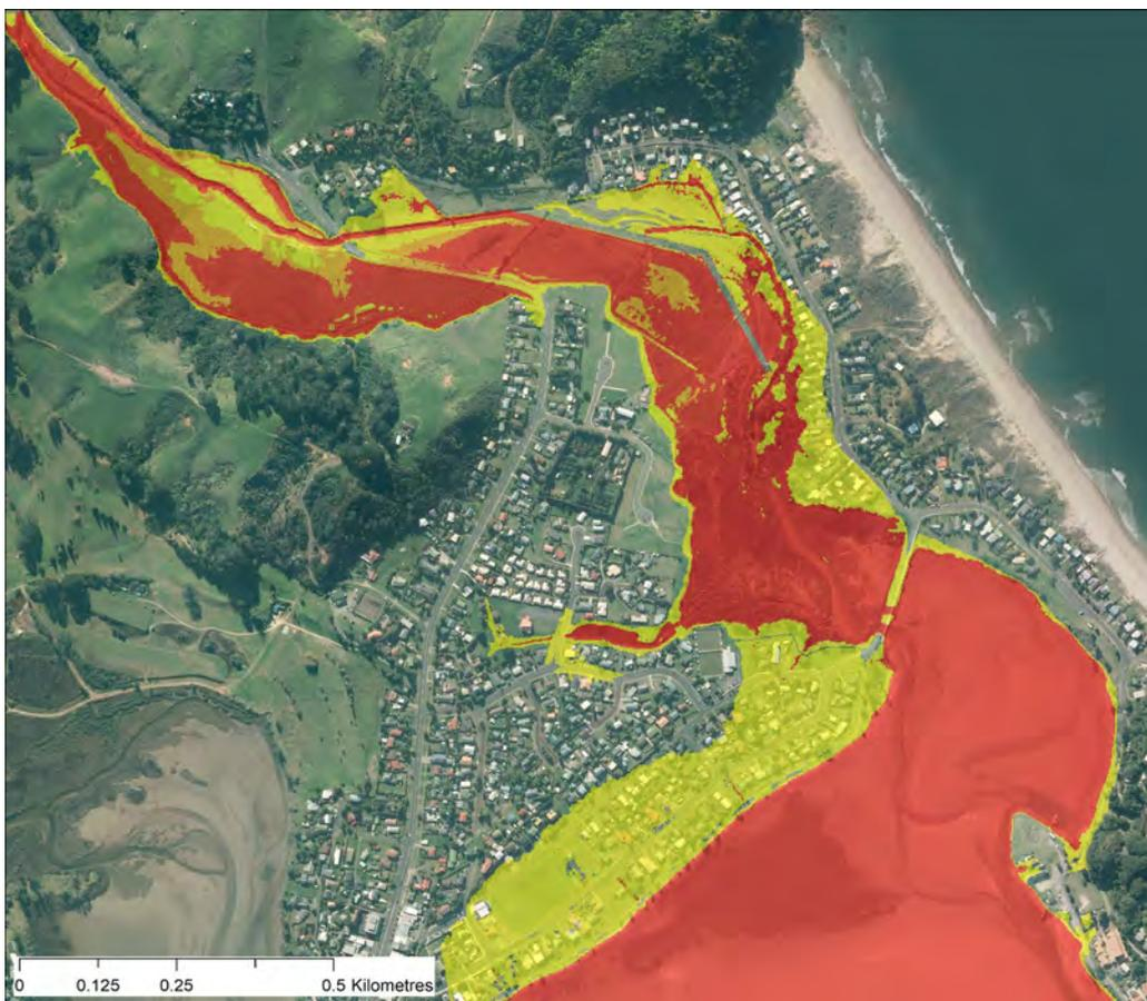
**Figure 20** Post-Scheme 1%AEP (100 year ARI) river flood hazard classification map for Grahams Creek with a projected 1.0 m sea level rise
