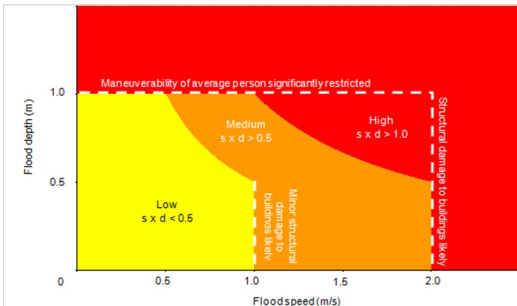
**Figure 15 River flood hazard classification matrix.**
