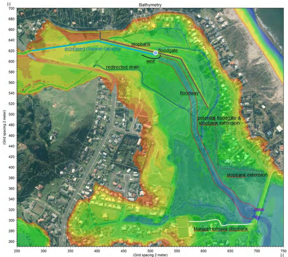
**Figure 13** Schematic showing bathymetry and location of flood alleviation components including stopbanks, increased channel capacity, floodway, floodgate, and redirected drain.
