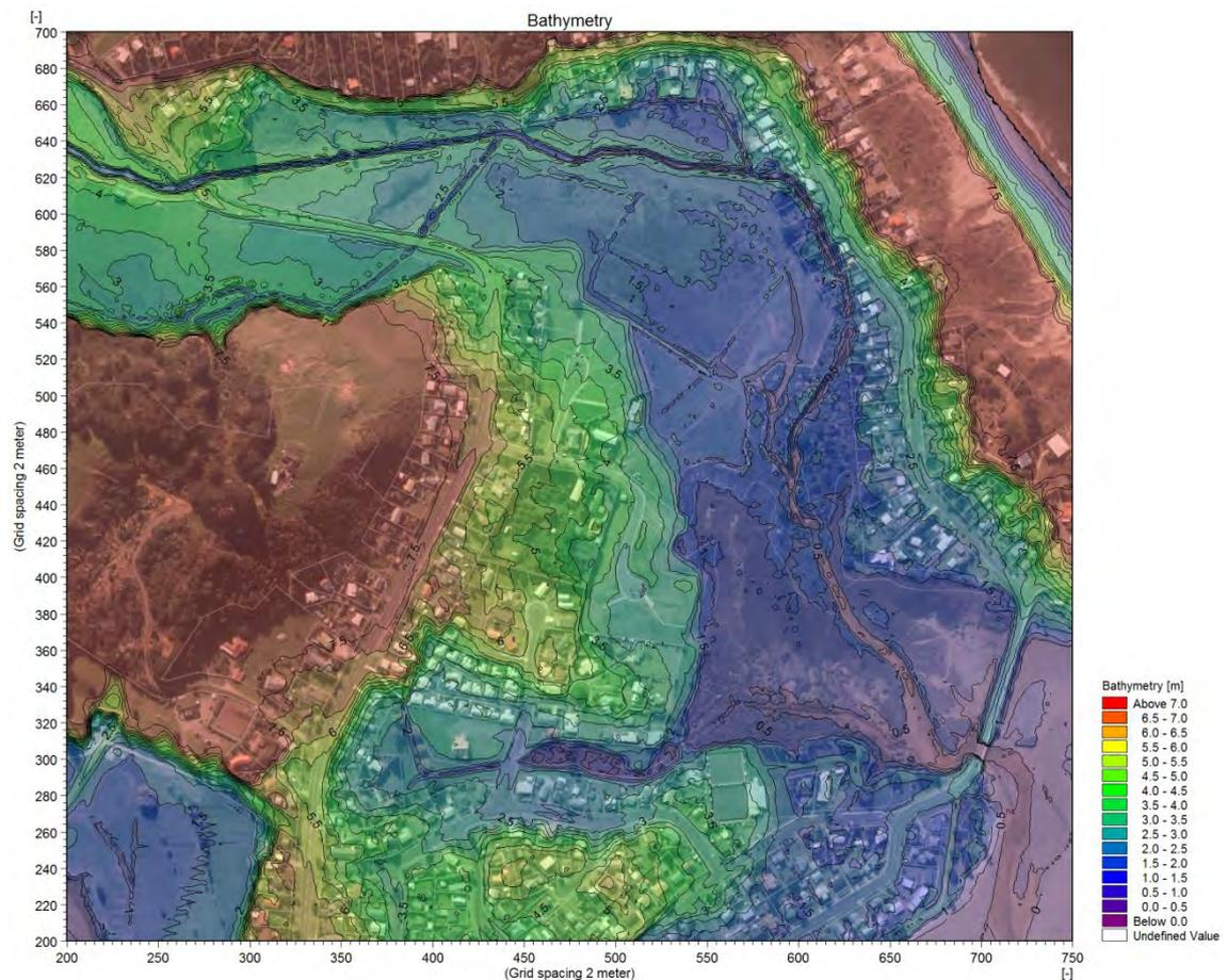
**Figure 8 Existing 2012 LIDAR bathymetry used in modelling the existing case with aerial/land parcel background (relative to Moturiki vertical datum)**
