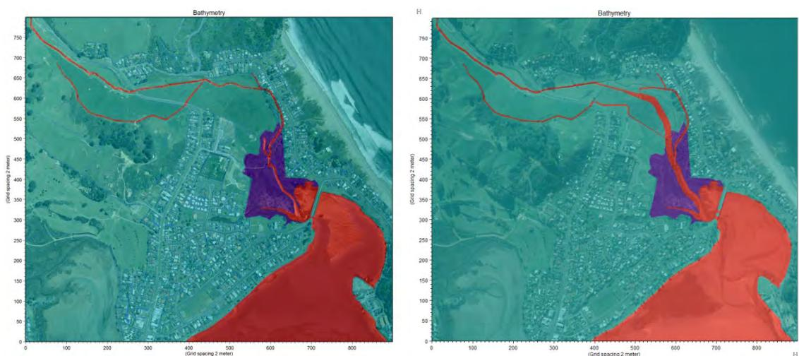
Figure 11 Roughness maps used in existing and proposed case
