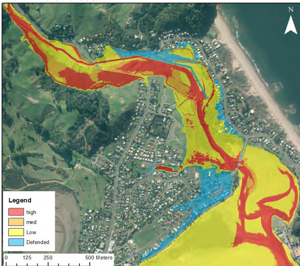
**Figure 17** Post-Scheme (current climate 1%AEP (100 year ARI) river flood hazard classification map for Grahams Creek.
