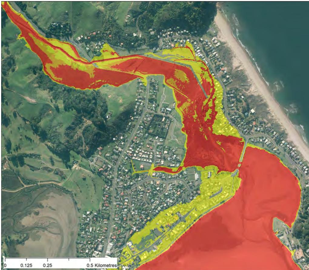
**Figure 19** Post-Scheme 1%AEP (100 year ARI) river flood hazard classification map for Grahams Creek with a projected 0.8 m sea level rise
