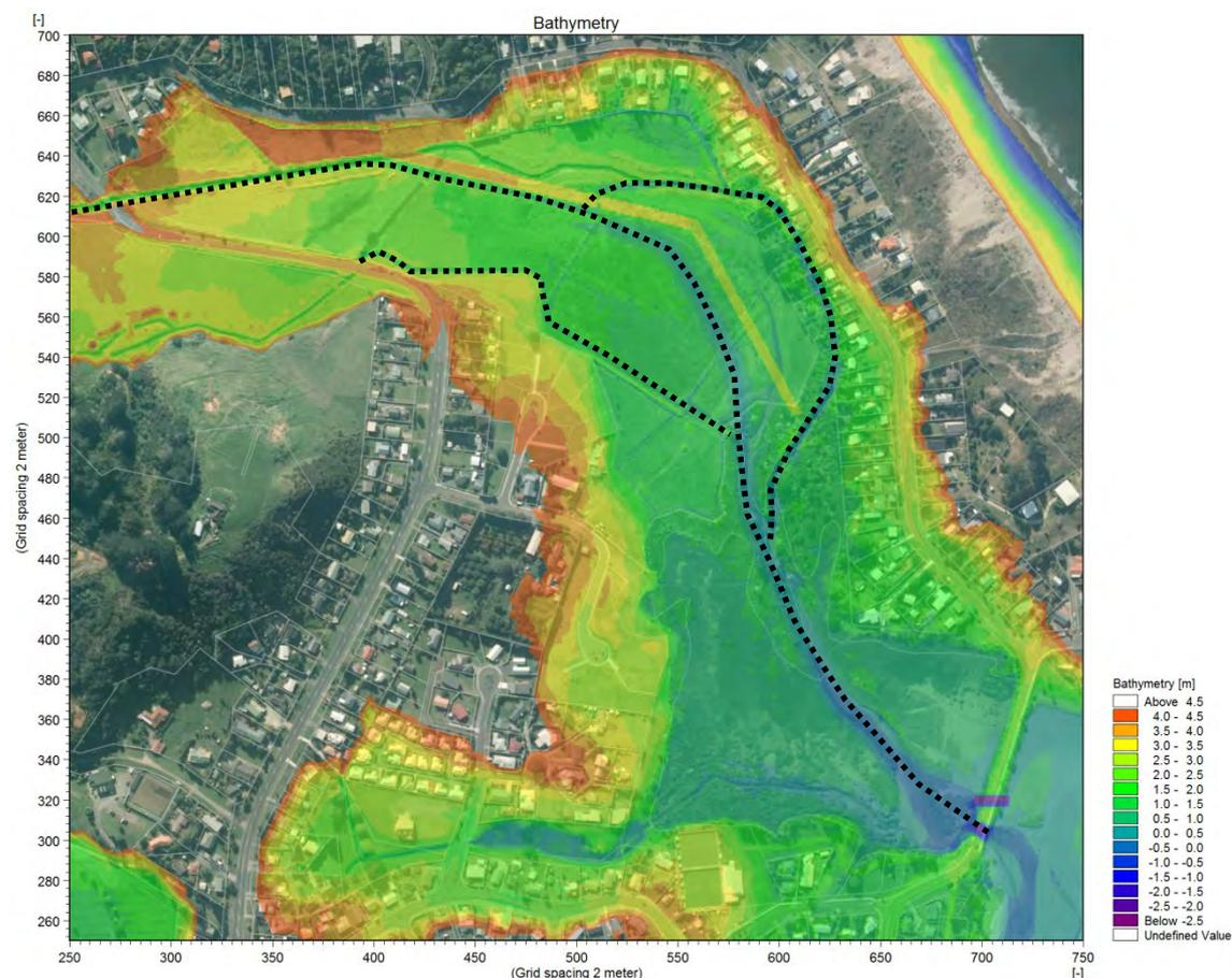
**Figure 14** Extent of channel maintenance in Grahams Stream, floodway and right bank drain (black dotted line).
