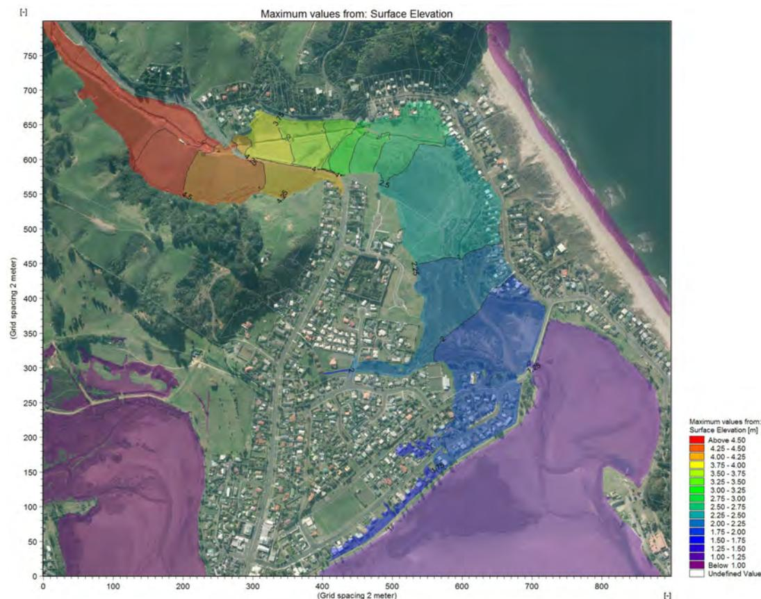
**Figure 6 Predicted inundation for the pre scheme 100y flood levels (relative to Moturiki vertical Datum)**
