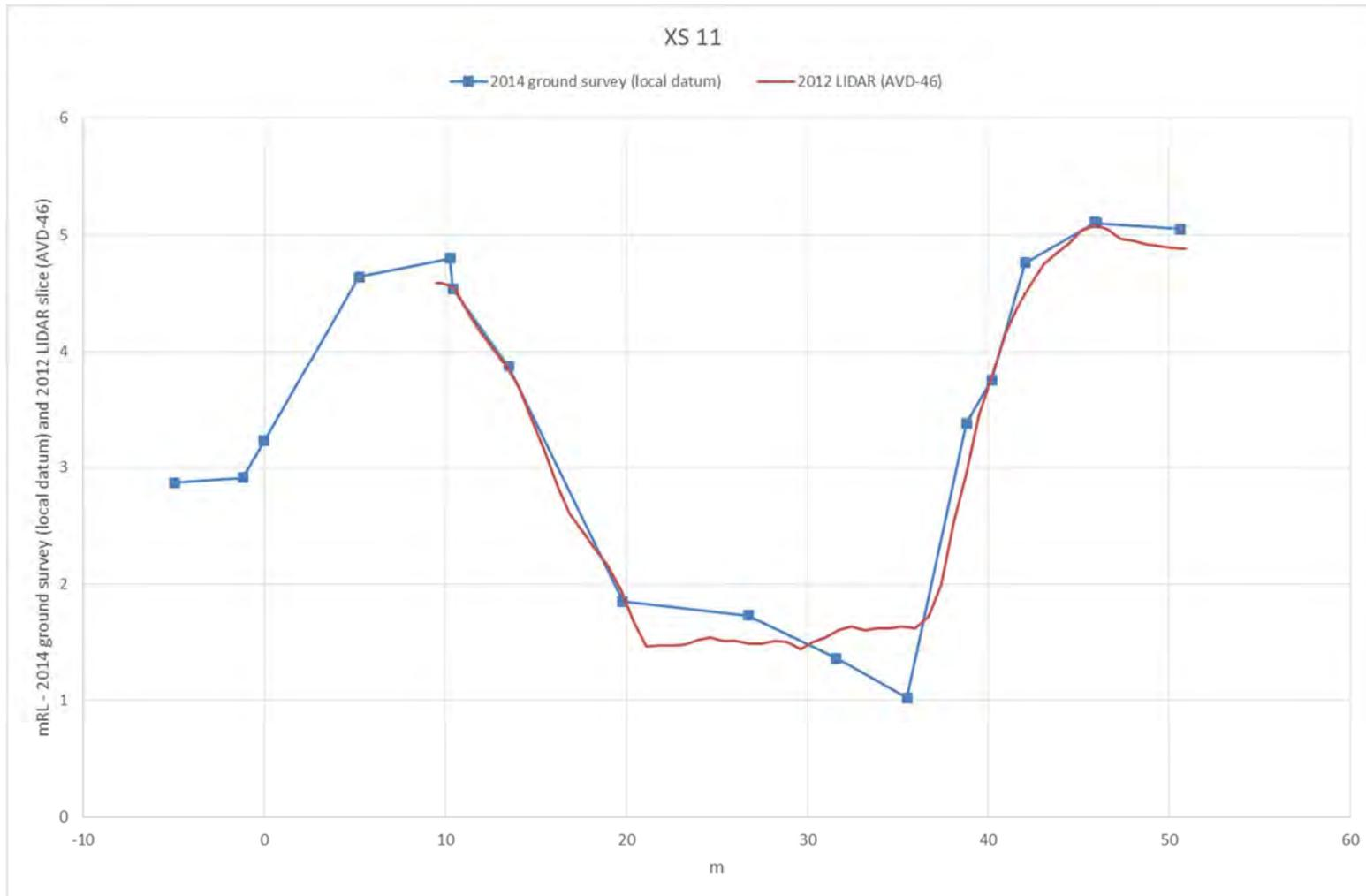
Figure A11 XS 11 (MIKE11 model chainage 501m – location shown in Figure A16)
