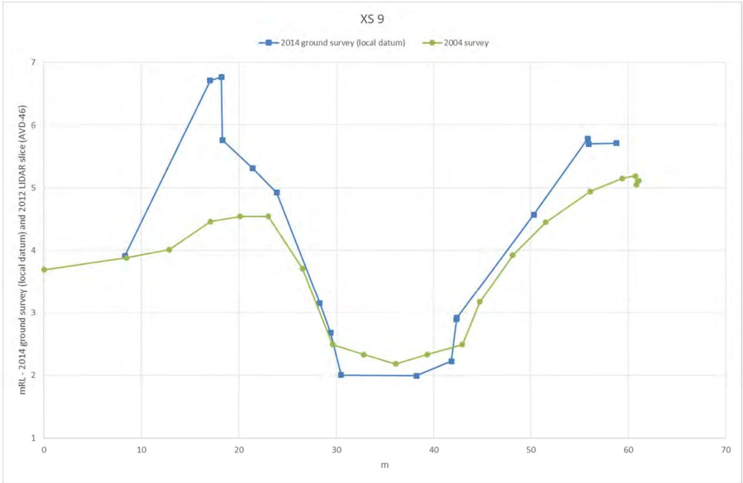
**Figure B9 Comparison of 2004 and 2014 survey at XS 9 (MIKE11 model chainage 402m – location shown in Figure A16)**
