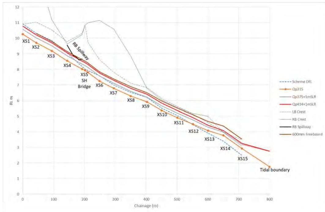
**Figure 18 Modelled flood profiles compared with original design flood levels and left and right bank assets.**
