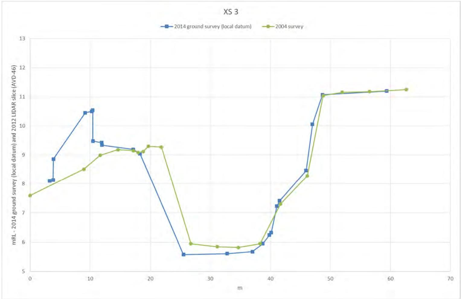
Figure B3 Comparison of 2004 and 2014 survey at XS 3 (MIKE11 model chainage 94m – location shown in Figure A16)
