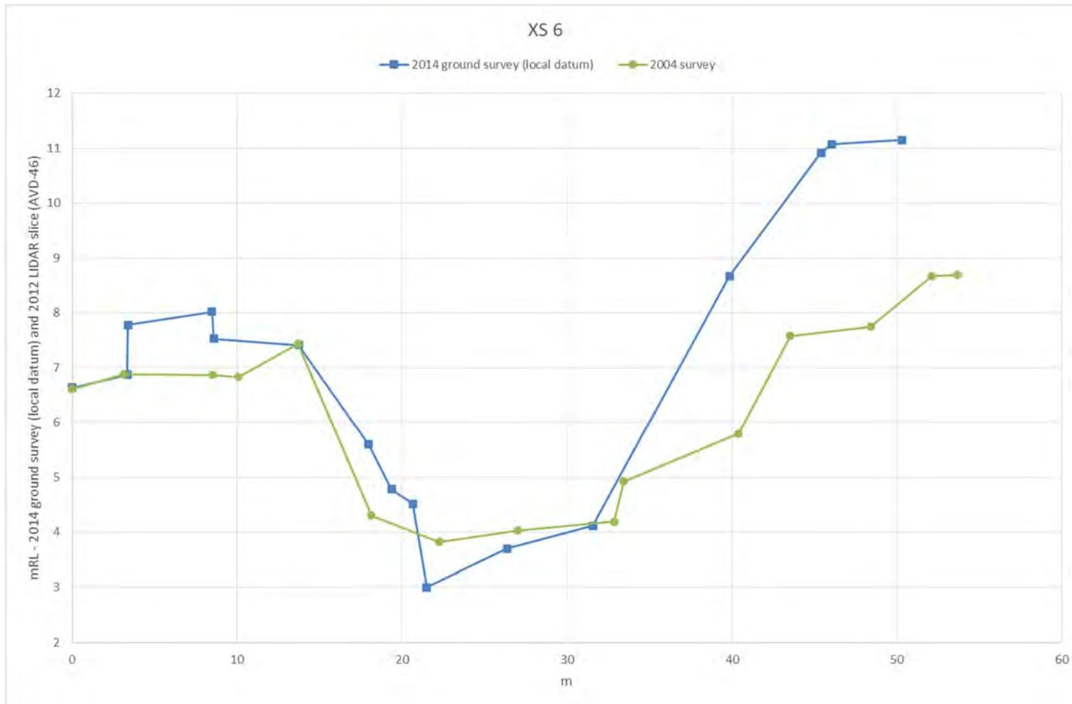
Figure B6 Comparison of 2004 and 2014 survey at XS 6 (MIKE11 model chainage 249m – location shown in Figure A16)
