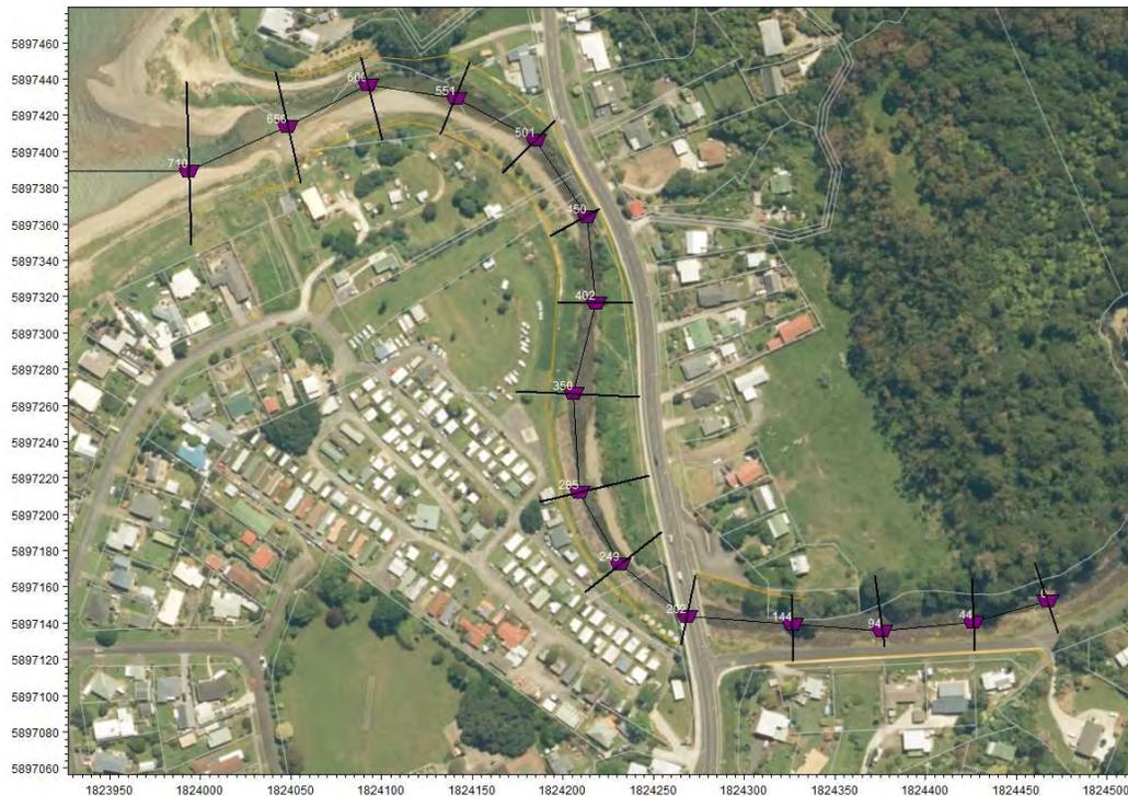
**Figure 15** Location and extent of 2014 ground survey cross-sections as shown in MIKE11 model. Note model chainage is shown in image but cross-sections are XS 1 (upstream - right) to XS 15 (downstream - left).
