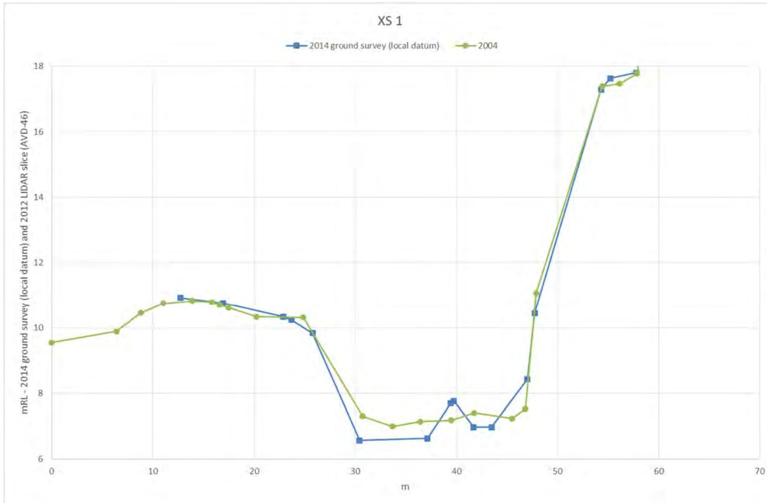
Figure B1 Comparison of 2004 and 2014 survey at XS 1 (MIKE11 model chainage 0m – location shown in Figure A16)
