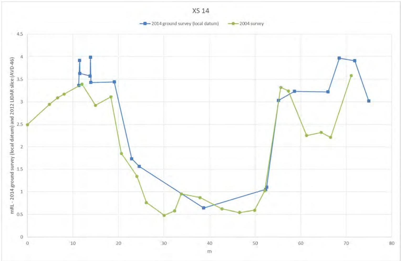
Figure B14 Comparison of 2004 and 2014 survey at XS 14 (MIKE11 model chainage 650m – location shown in Figure A16)
