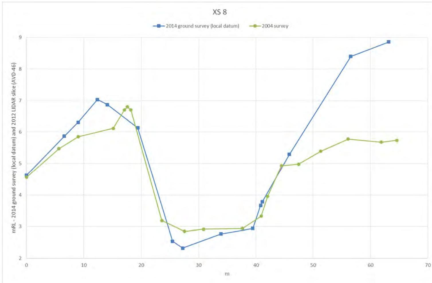
**Figure B8 Comparison of 2004 and 2014 survey at XS 8 (MIKE11 model chainage 350m – location shown in Figure A16)**
