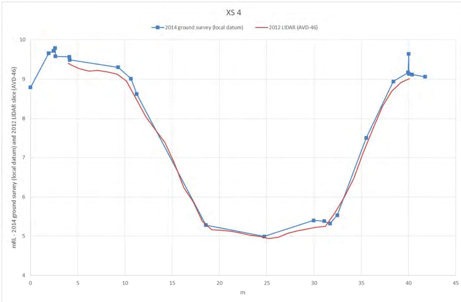
Figure A4 XS 4 (MIKE11 model chainage 144m – location shown in Figure A16)
