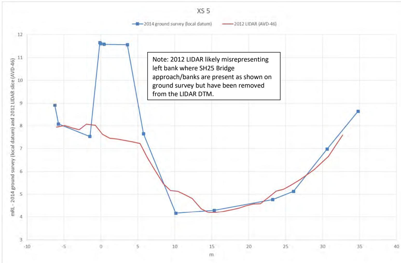
Figure A5 XS 5 (MIKE11 model chainage 202m – location shown in Figure A16)
