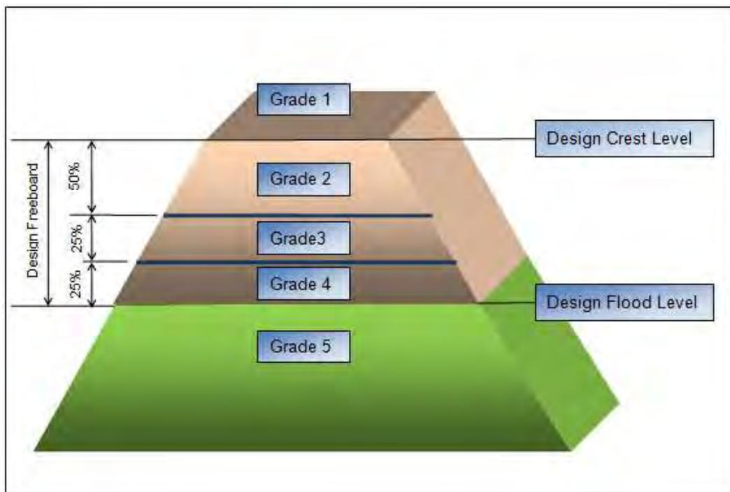
**Figure 33** Diagrammatic representation of stopbank performance grades.
