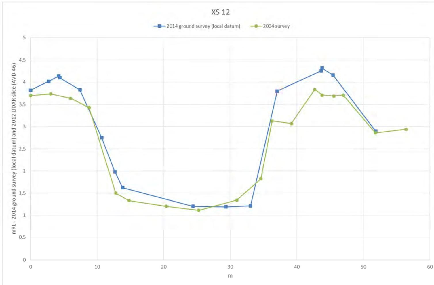
Figure B12 Comparison of 2004 and 2014 survey at XS 12 (MIKE11 model chainage 551m – location shown in Figure A16)
