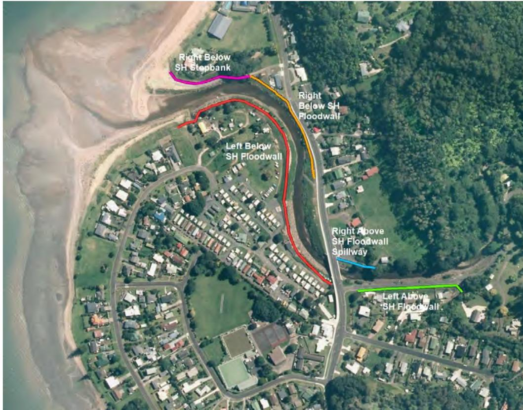
**Figure 11** Location of Te Puru flood protection scheme assets.
