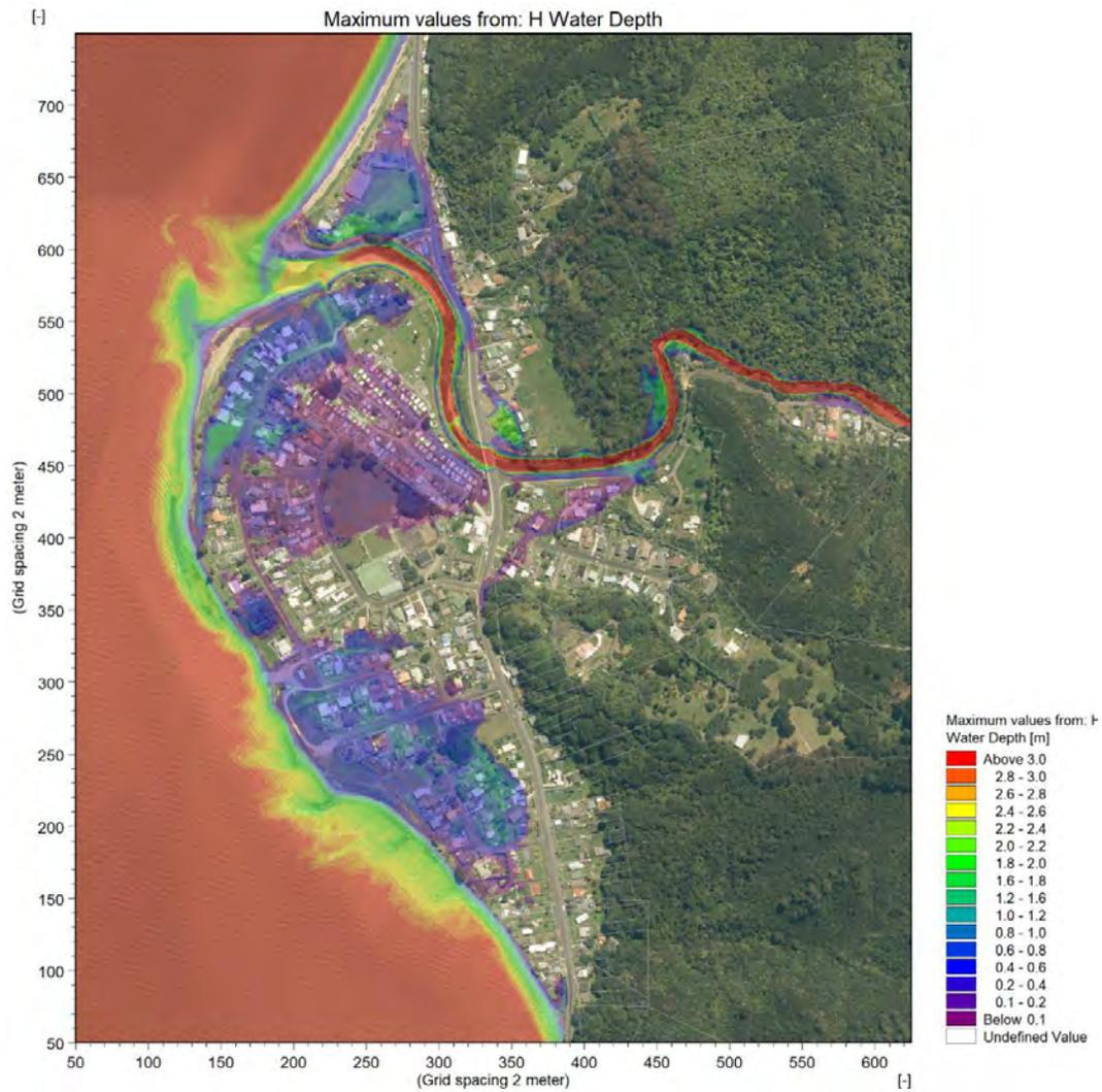
**Figure 23** MIKE21 model estimated maximum depth for future climate (RCP 6.0) 1%AEP design discharge ( $Q_p375$ ) and MWHS tide (RL 2.76m).
