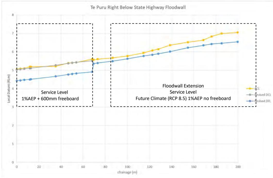
**Figure 31** Te Puru Right Below State Highway Floodwall - profiles for actual crest level (ACL) compared to the revised design crest level (DCL) and design flood level (DFL).
