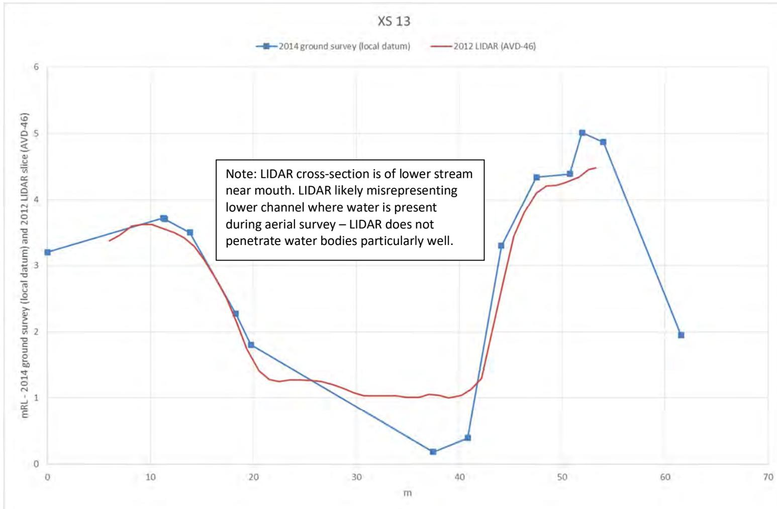
Figure A13 XS 13 (MIKE11 model chainage 600m – location shown in Figure A16)
