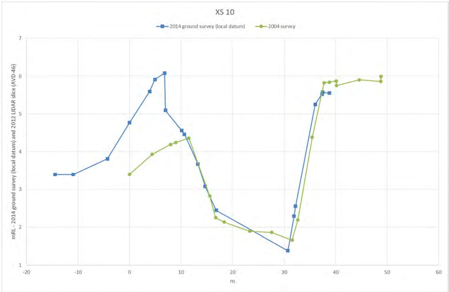
Figure B10 Comparison of 2004 and 2014 survey at XS 10 (MIKE11 model chainage 450m – location shown in Figure A16)
