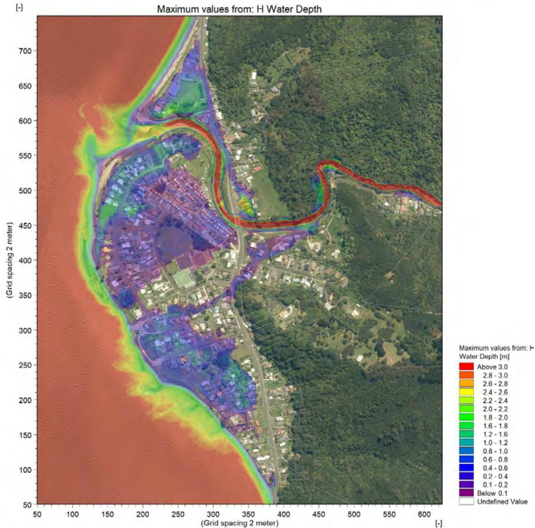
Figure 24 MIKE21 model estimated maximum depth for future climate (RCP 8.5) 1%AEP design discharge ( $Q_{p414}$ ) and MWHS tide (RL 2.76m).
