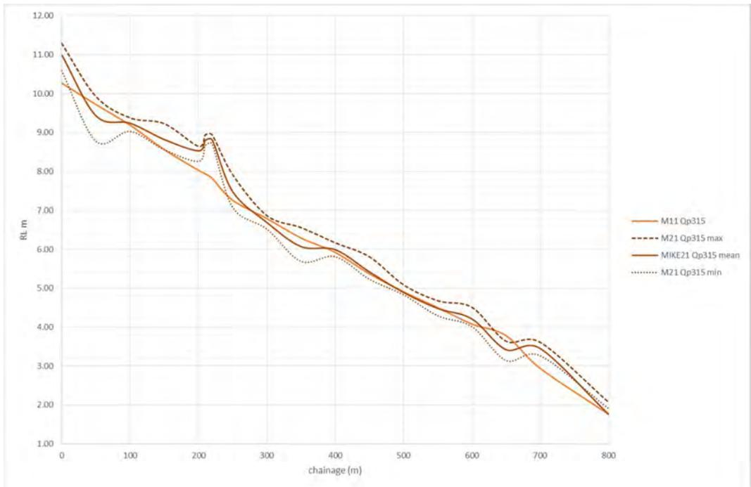
**Figure 26** Comparison of Q<sub>p315</sub> MIKE11 maximum water levels and MIKE21 minimum and maximum water levels at cross-sections alignments.
