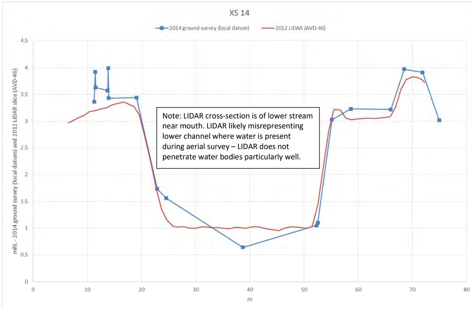
Figure A14 XS 14 (MIKE11 model chainage 650m – location shown in Figure A16)
