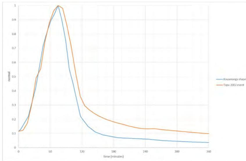
**Figure 9 Comparison of normalised Kauaeranga shape hydrograph and that from the Tapu catchment.**
