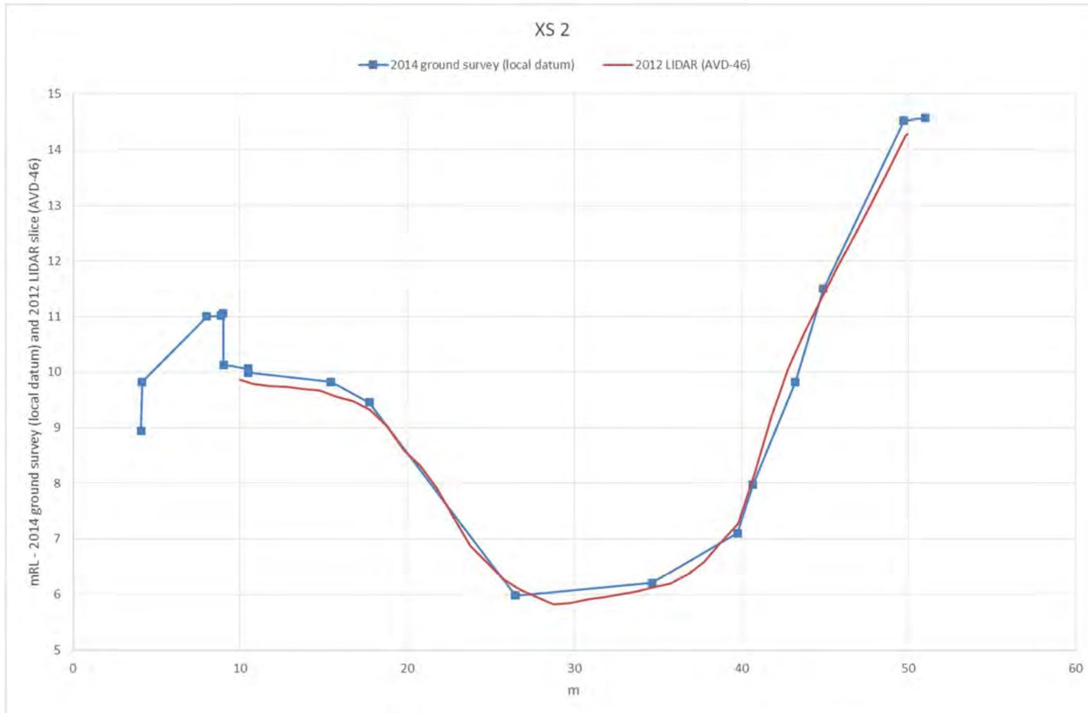
Figure A2 XS 2 (MIKE11 model chainage 44m – location shown in Figure A16)
