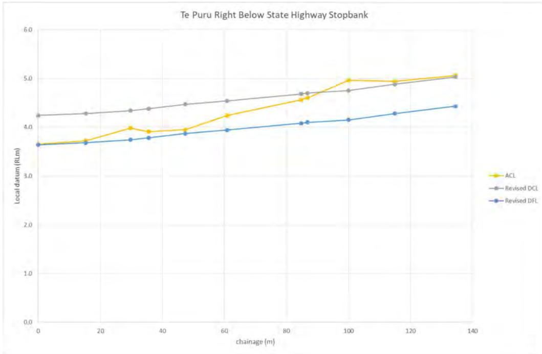
**Figure 30** Te Puru Right Below State Highway Stopbank - profiles for actual crest level (ACL) compared to the revised design crest level (DCL) and design flood level (DFL).
