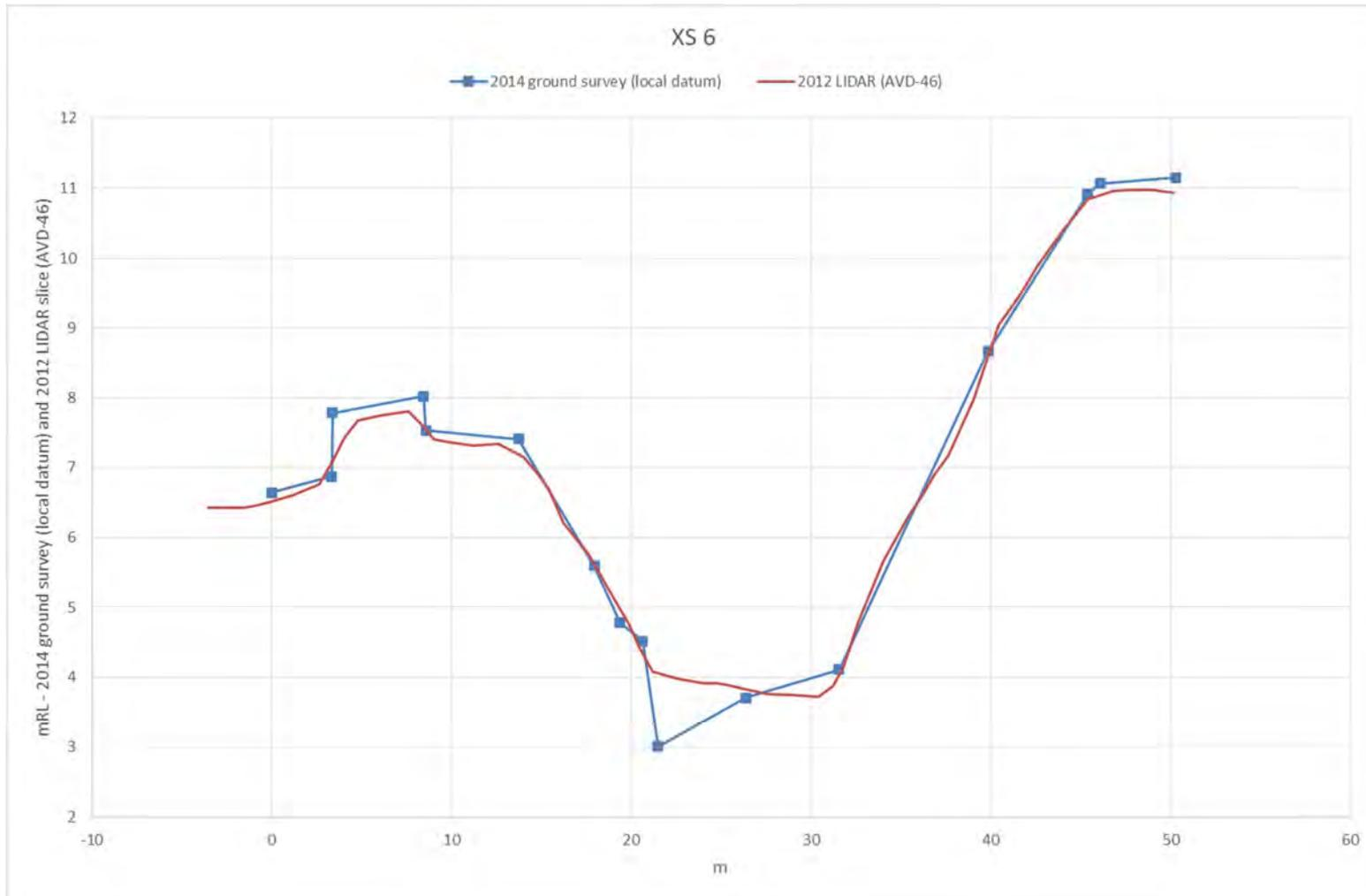
Figure A6 XS 6 (MIKE11 model chainage 249m – location shown in Figure A16)
