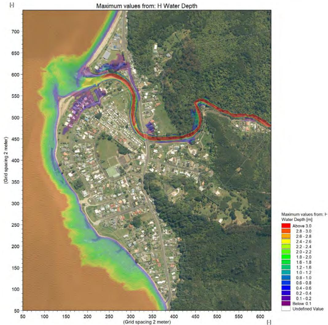
**Figure 22 MIKE21 model estimated maximum depth for present climate 1%AEP design discharge (Q<sub>p315</sub>) and MWHS tide (RL 1.76m) considering MIKE21 model.**
