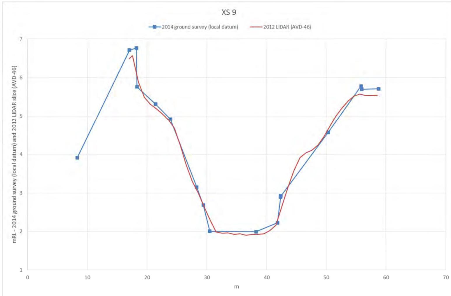
Figure A9 XS 9 (MIKE11 model chainage 402m – location shown in Figure A16)
