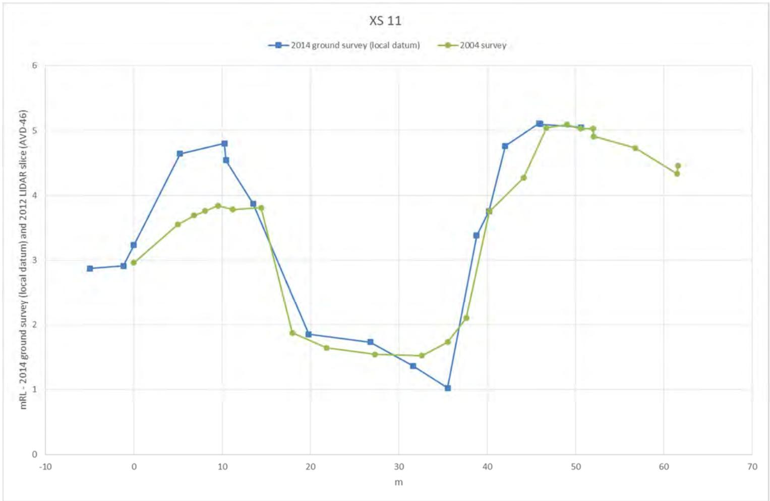
Figure B11 Comparison of 2004 and 2014 survey at XS 11 (MIKE11 model chainage 501m – location shown in Figure A16)
