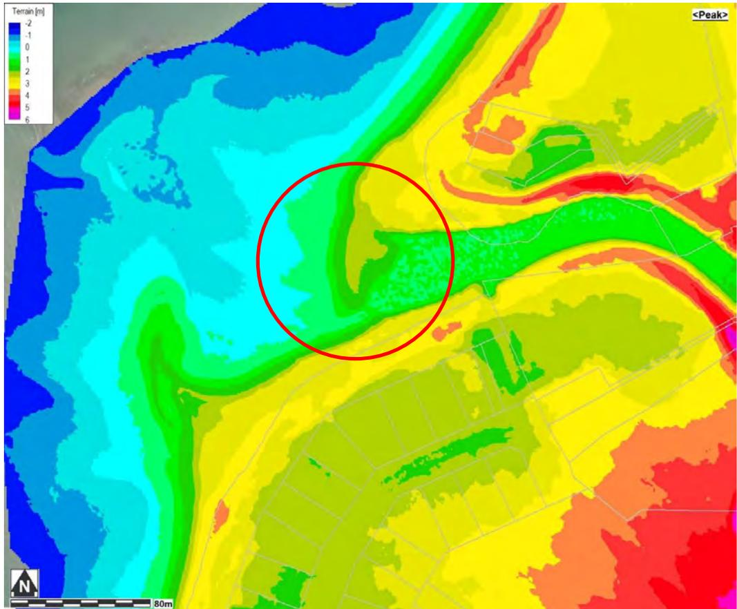
**Figure 27** 2013 LIDAR imagery showing narrow channel opening and spit extending from north bank at time of LIDAR capture.
