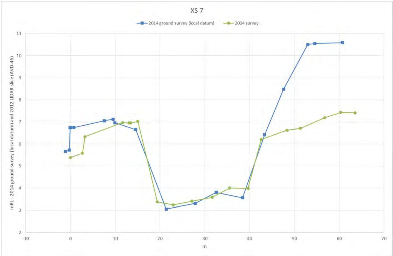
**Figure B7 Comparison of 2004 and 2014 survey at XS 7 (MIKE11 model chainage 295m – location shown in Figure A16)**
