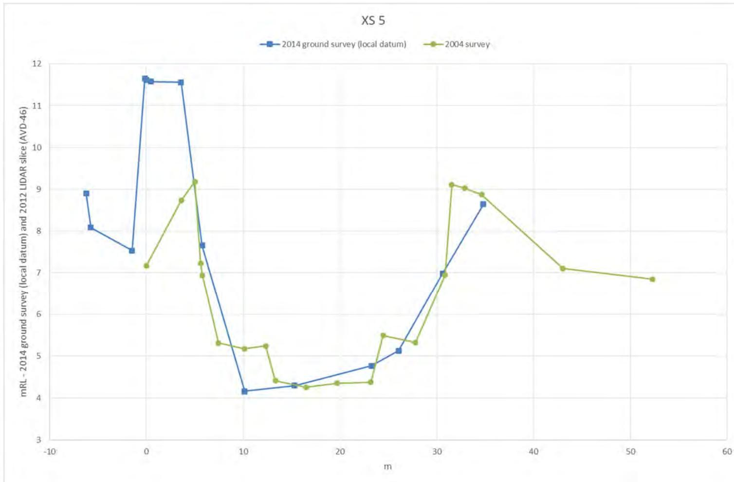
Figure B5 Comparison of 2004 and 2014 survey at XS 5 (MIKE11 model chainage 202m – location shown in Figure A16)
