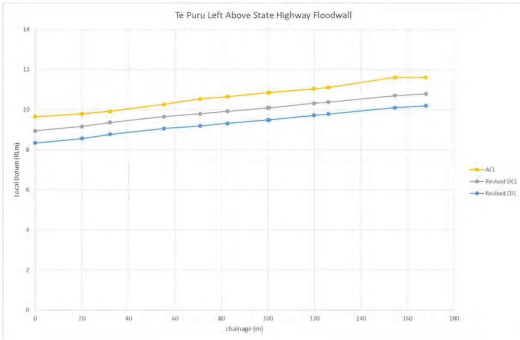
**Figure 29** Te Puru Left Above State Highway Floodwall - profiles for actual crest level (ACL) compared to the revised design crest level (DCL) and design flood level (DFL).
