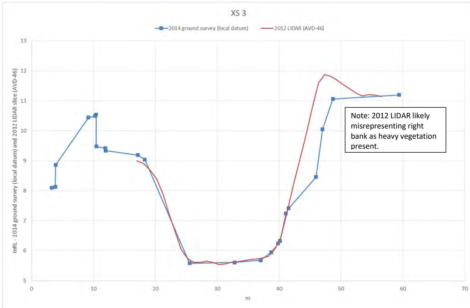
Figure A3 XS 3 (MIKE11 model chainage 94m – location shown in Figure A16)
