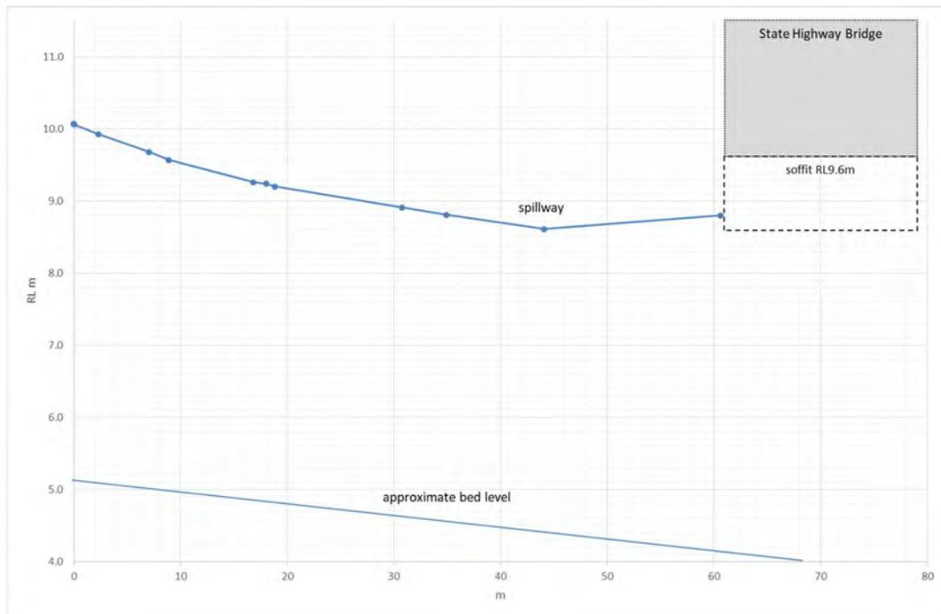
**Figure 17** Right bank spillway upstream of State Highway Bridge as surveyed in 2014 (as viewed from right bank). Note bed and bridge are approximated in image.
