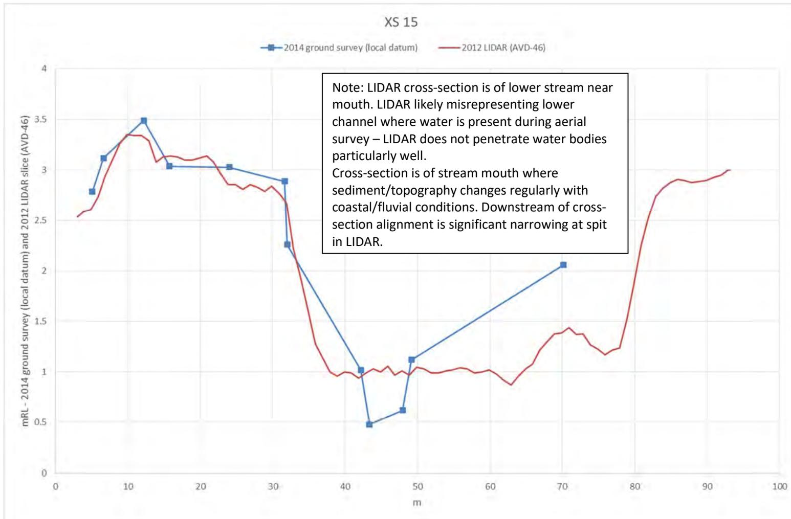
Figure A15 XS 15 (MIKE11 model chainage 710m – location shown in Figure A16)
