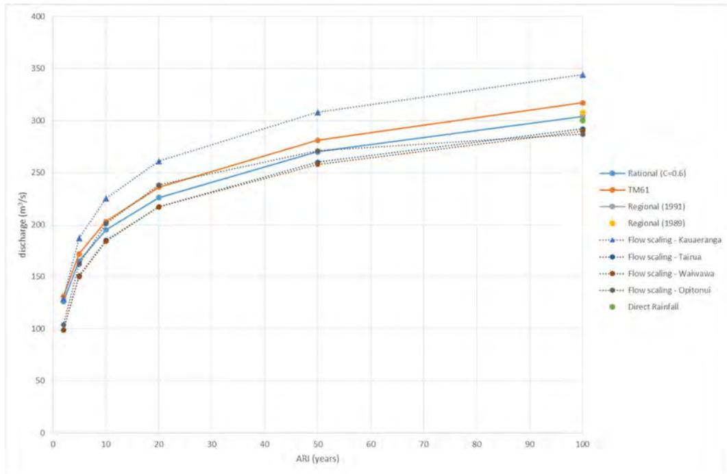
Figure 8 Comparison of various methods for current climate discharge estimates.
