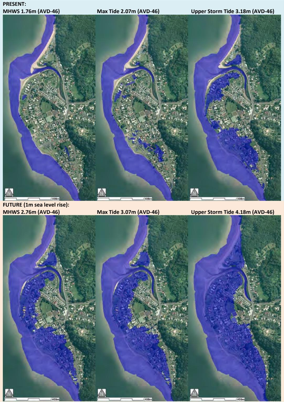
Figure 10 Various coastal water levels on 2013 LIDAR surface (AVD-46). Note: Future water levels include 1.0m of sea level rise.
