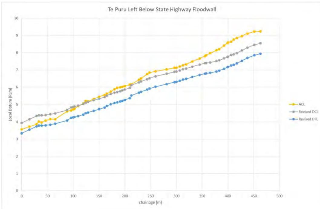
**Figure 28** Te Puru Left Below State Highway Floodwall - profiles for actual crest level (ACL) compared to the revised design crest level (DCL) and design flood level (DFL).
