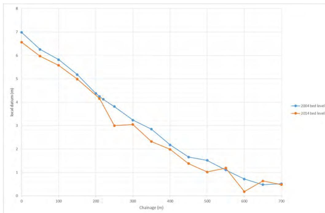
**Figure 19** Minimum bed level profiles from 2004 and 2014 channel surveys between XS 1 (upstream) and XS 15 (downstream).
