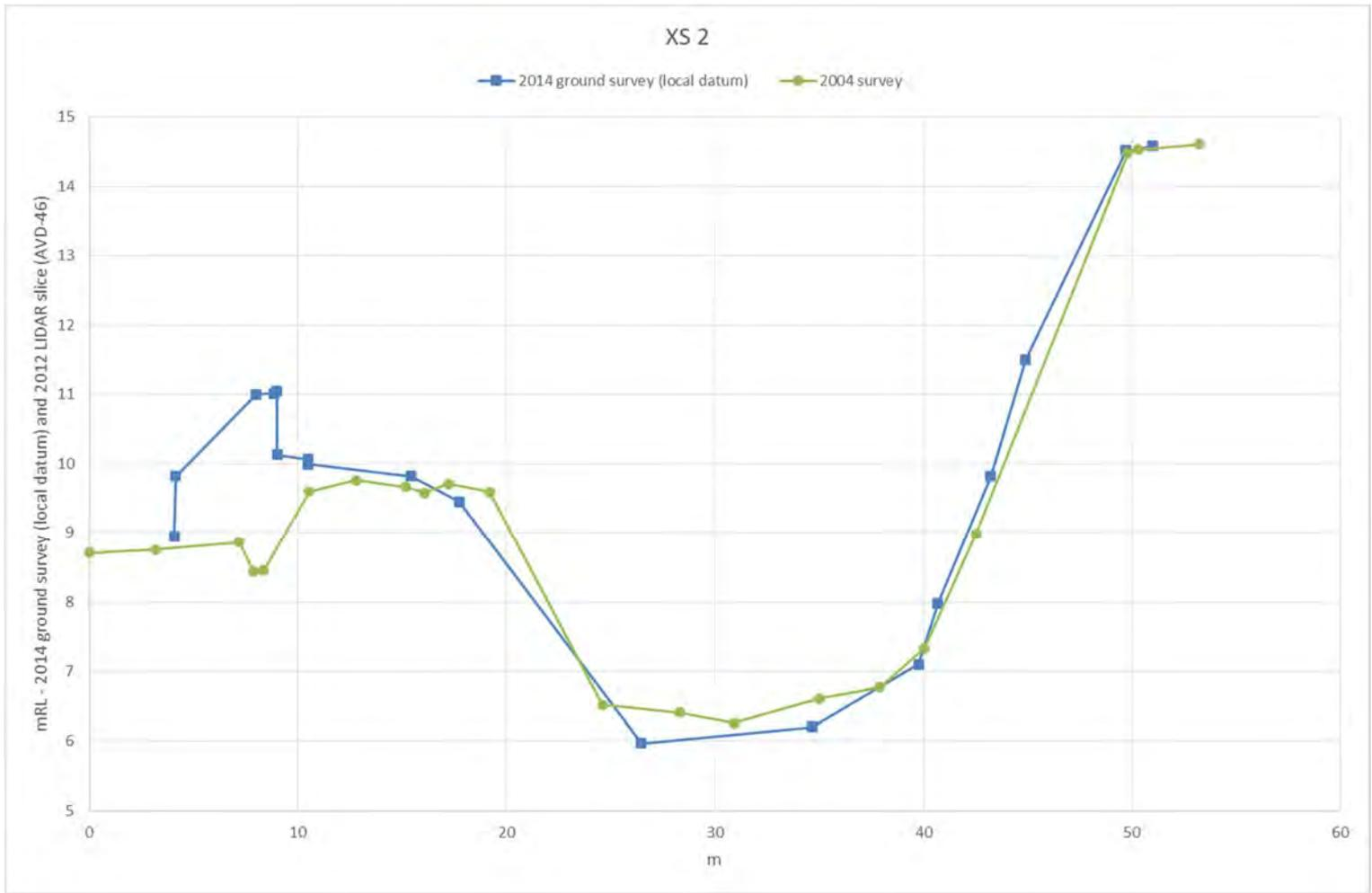
Figure B2 Comparison of 2004 and 2014 survey at XS 2 (MIKE11 model chainage 44m – location shown in Figure A16)
