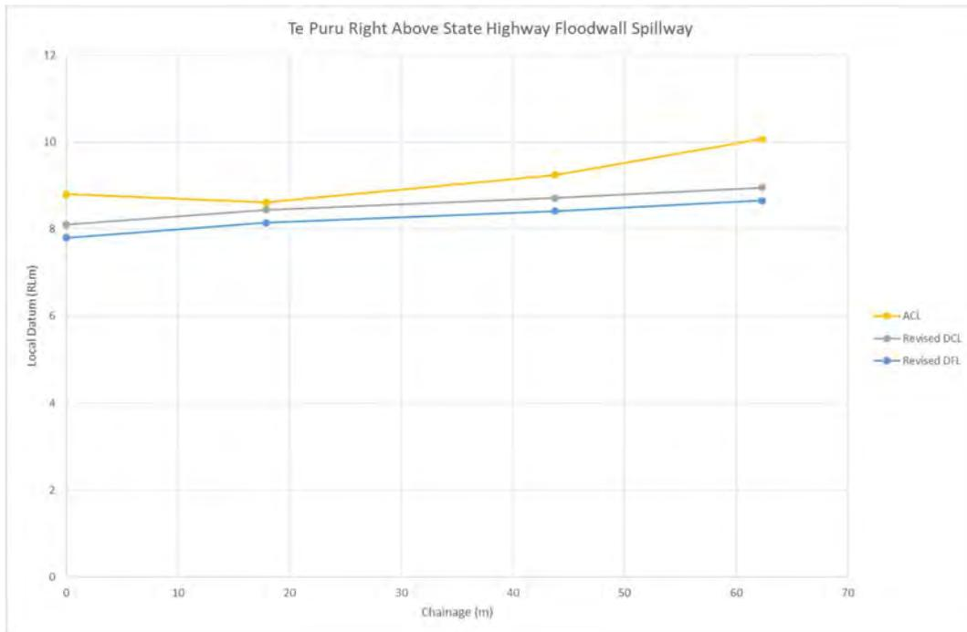
**Figure 32** Te Puru Right Above State Highway Floodwall Spillway - profiles for actual crest level (ACL) compared to the revised design crest level (DCL) and design flood level (DFL).
