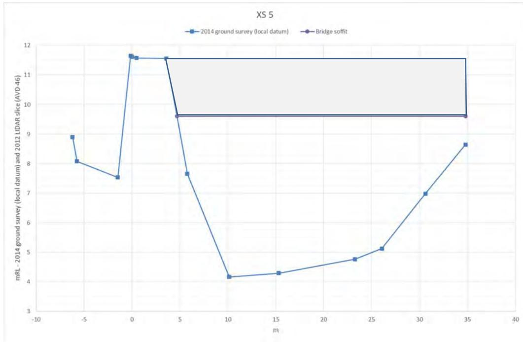
**Figure 16** State Highway Bridge cross-section (XS 5) as surveyed in 2014, minimum bridge soffit shown at RL 9.6m, with left bank bridge approach / stopbank adjacent.
