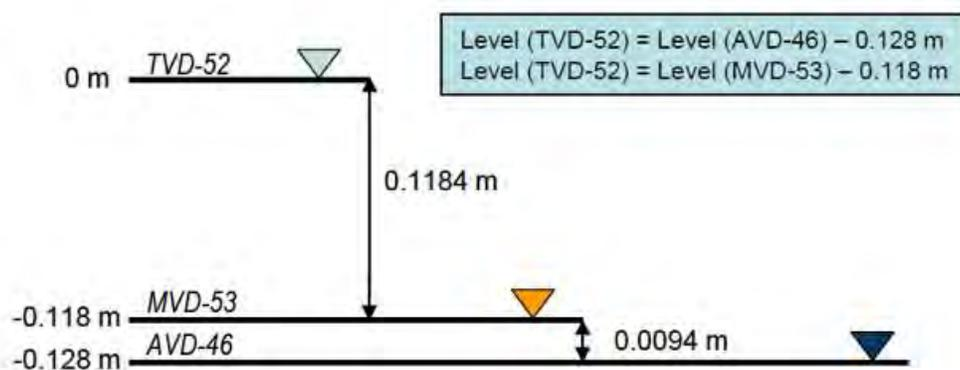
Figure 12 Relationship and conversions between the three local vertical datum of Tararu (TVD-52), Moturiki (MVD-53) and Auckland (AVD-46).
