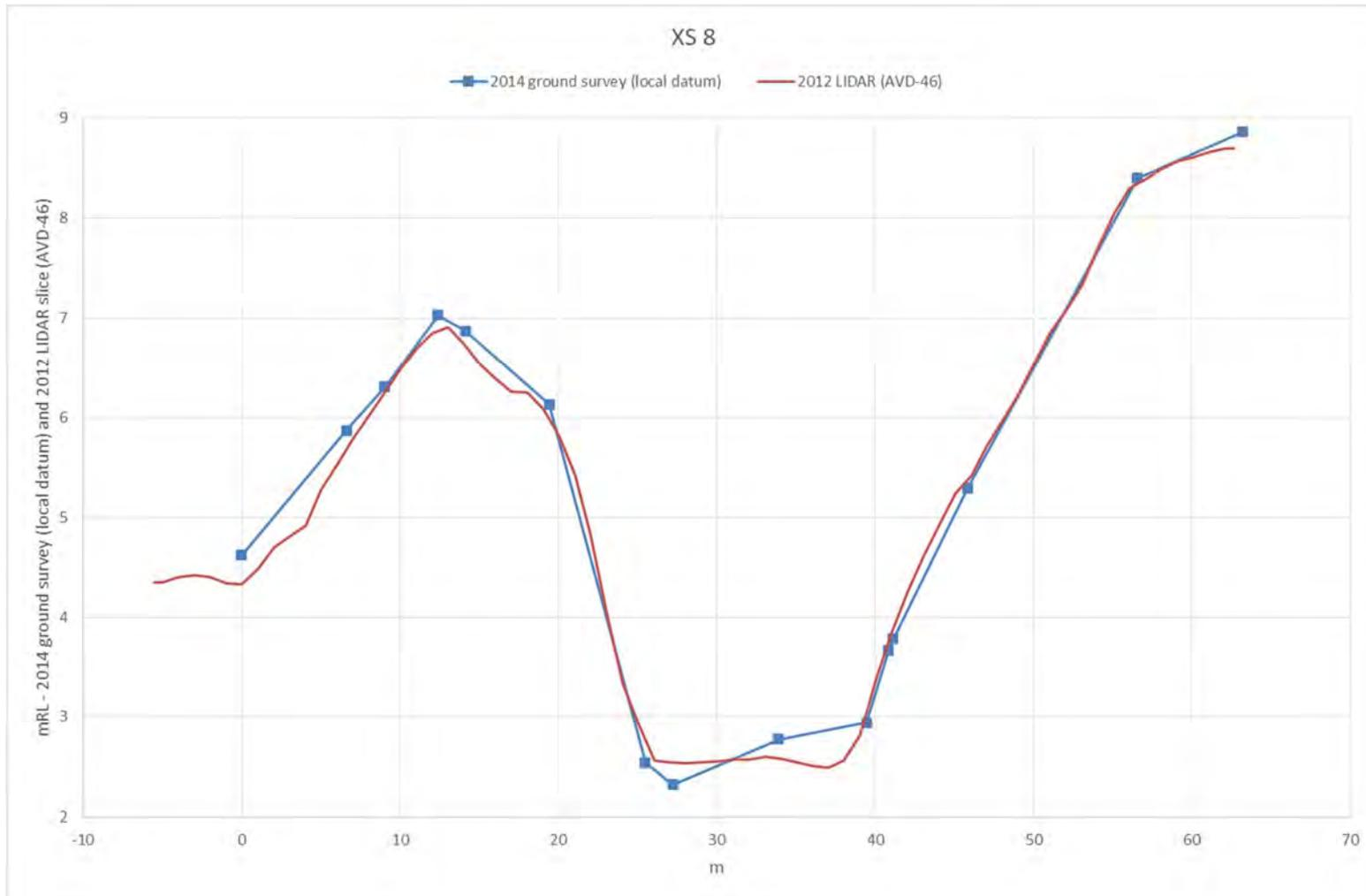
Figure A8 XS 8 (MIKE11 model chainage 350m – location shown in Figure A16)
