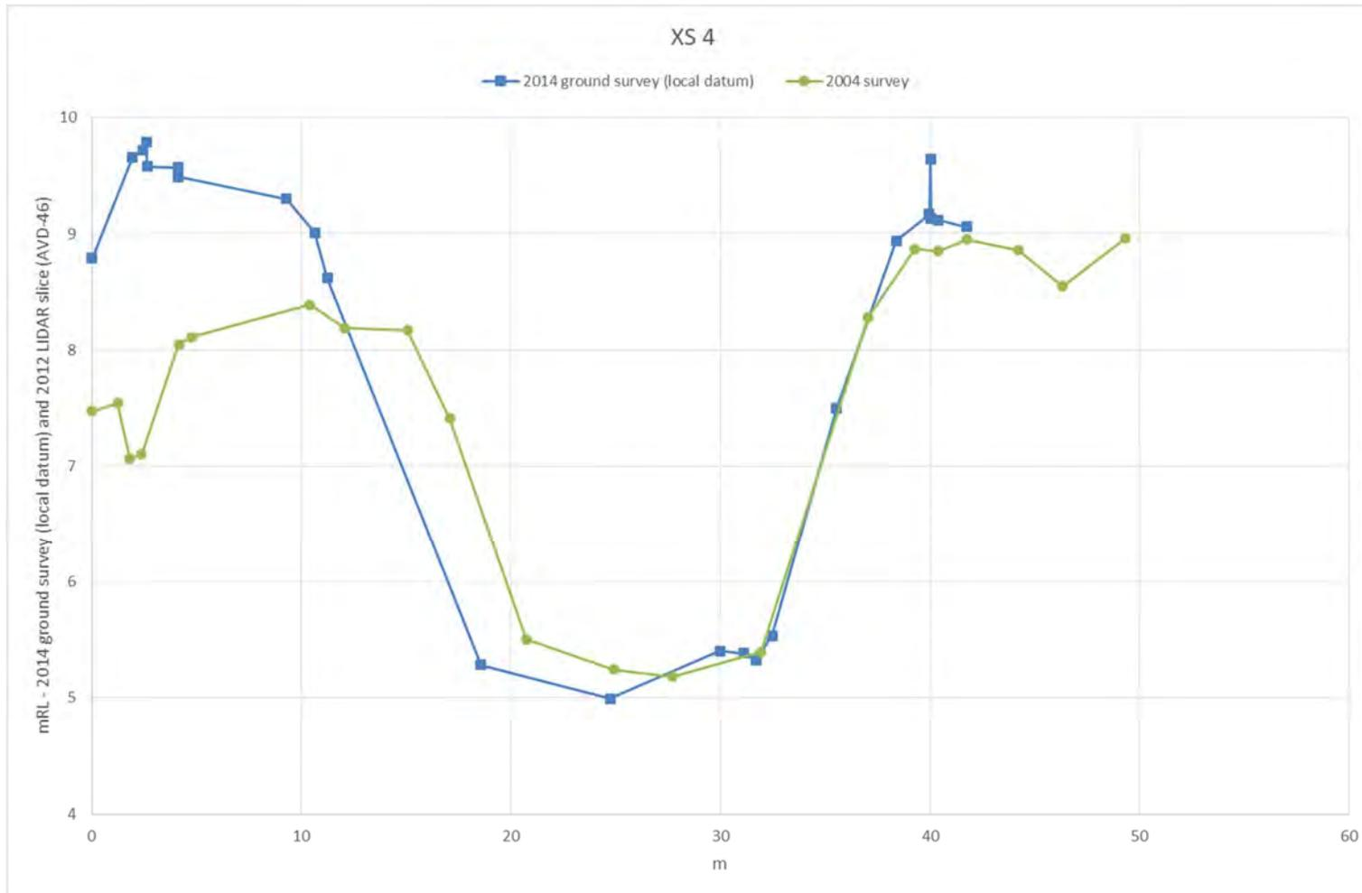
**Figure B4** Comparison of 2004 and 2014 survey at XS 4 (MIKE11 model chainage 144m – location shown in Figure A16)
