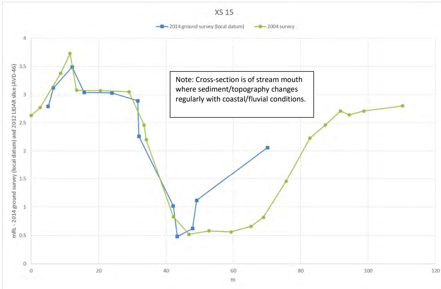
Figure B15 Comparison of 2004 and 2014 survey at XS 15 (MIKE11 model chainage 710m – location shown in Figure A16)
