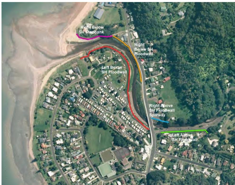
**Figure 1** Location of Te Puru flood protection scheme assets.
