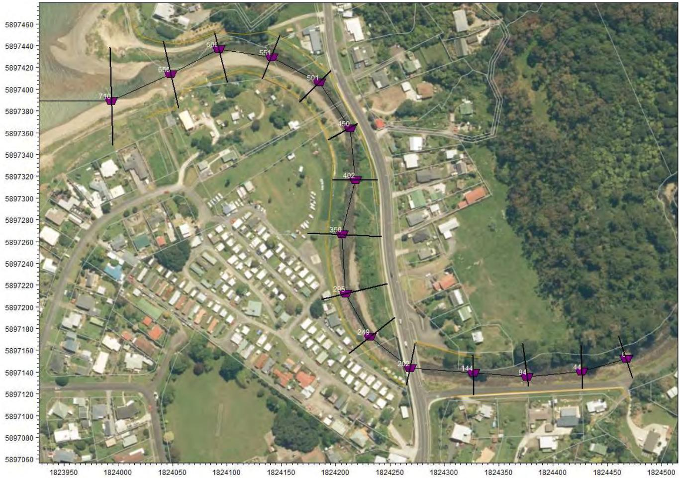
Figure A16 Location of ground survey cross-sections as shown in the MIKE11 model. Note model chainages are shown in image but cross-sections are XS 1 (upstream) to XS 15 (downstream).
