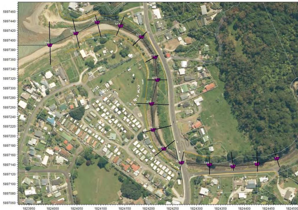
**Figure 4** Location and extent of 2020 ground survey cross-sections as shown in MIKE11 model. Note model chainage is shown in image but cross-sections are XS 1 (upstream - right) to XS 15 (downstream - left).
