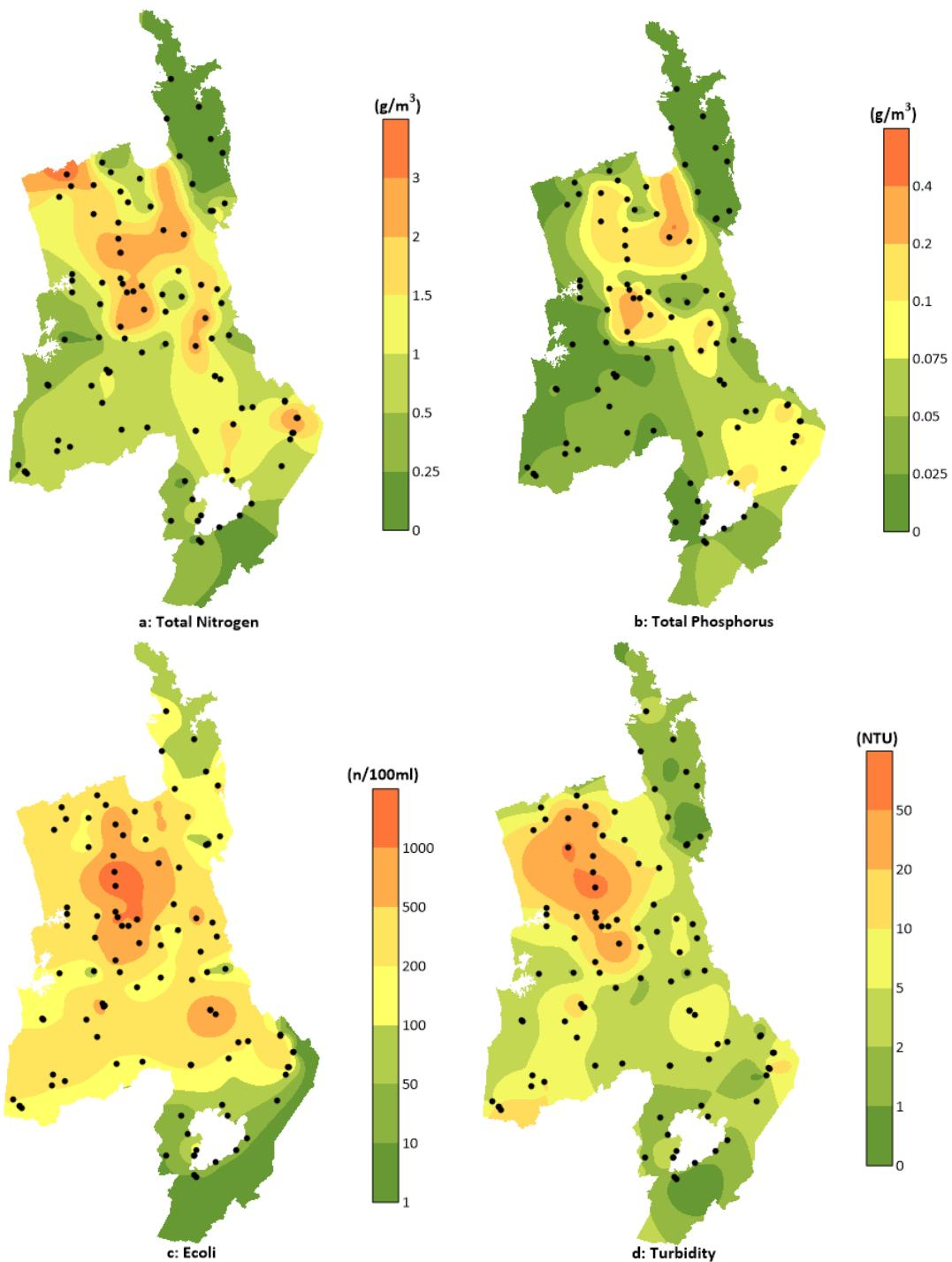
**Figure 2:** Spatial contour plots of four water quality parameters (based on 5 year median values, 2015-2019); a: Total Nitrogen, b: Total Phosphorus, c: Escherichia coli, d: Turbidity
