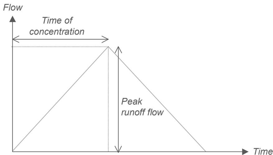
*Figure: Generalised flood hydrograph produced for each catchment*
