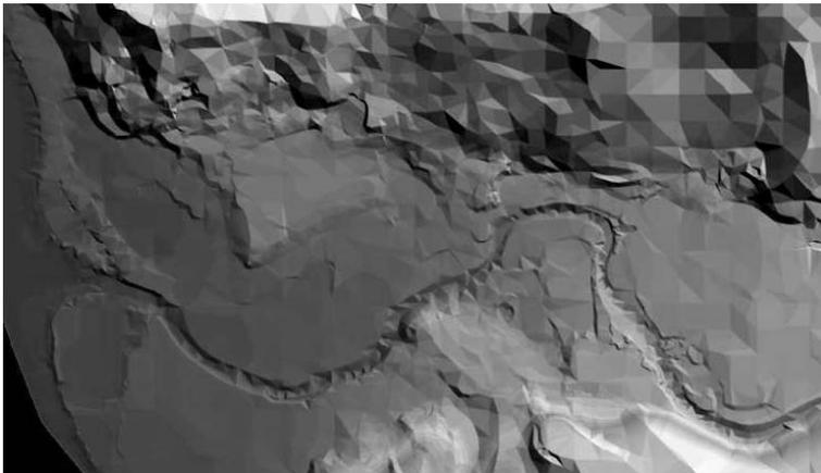
*Figure: A digital elevation model of the Tararu Stream and floodplain*
