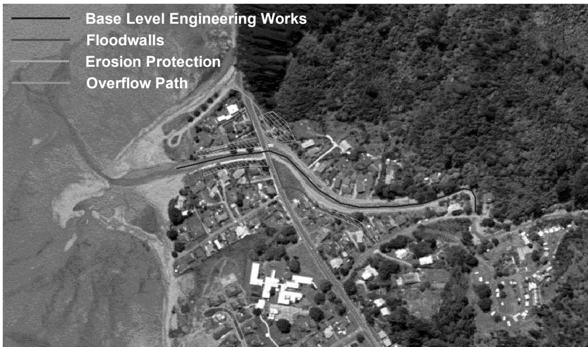
*Figure: Intermediate engineering works on the Tararu Stream*
