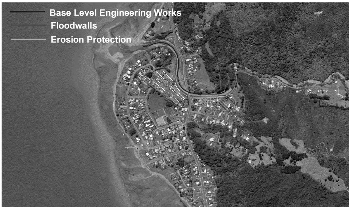
*Figure: Full engineering works on the Te Puru Stream*
