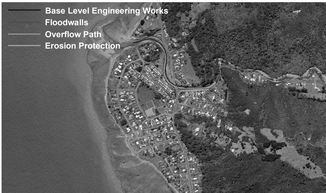
*Figure: Intermediate engineering works on the Te Puru Stream*
