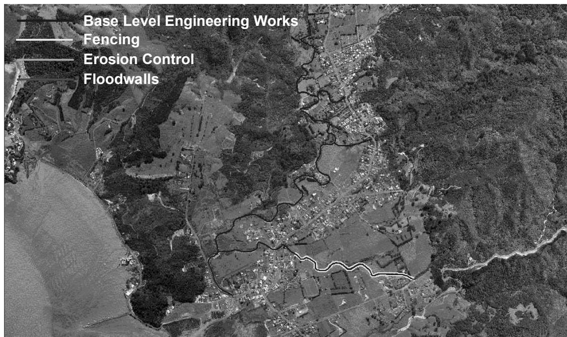
*Figure: Full engineering works on the Whangarahi Stream*
