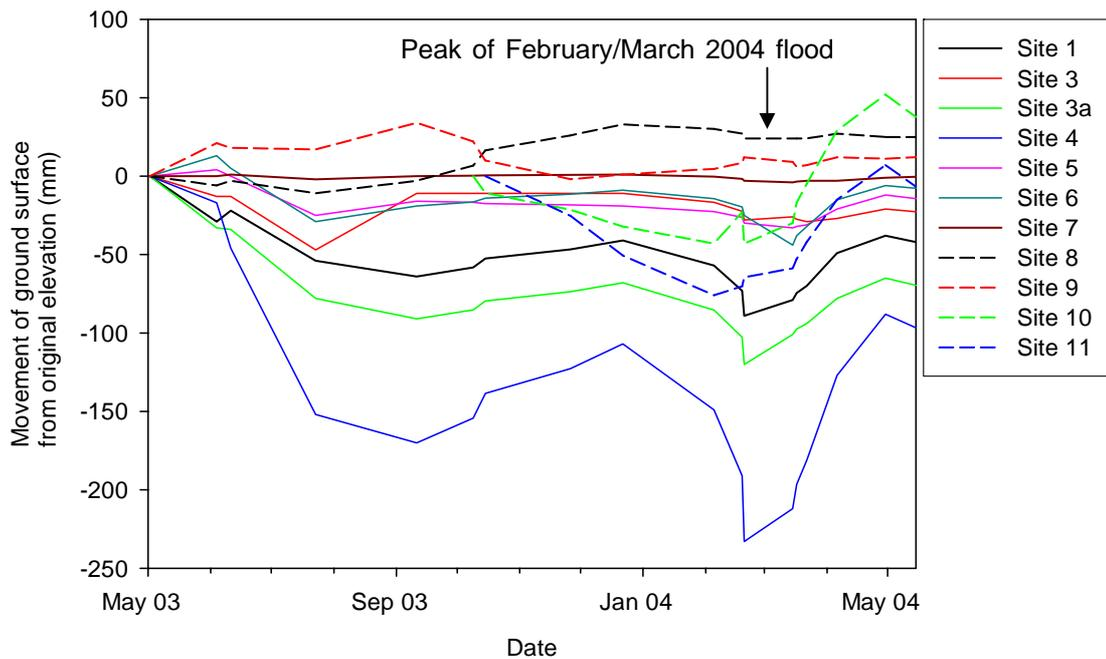
**Figure 20: Movement of the ground surface relative to a reference pole anchored in the mineral substrate below peat deposits.**
