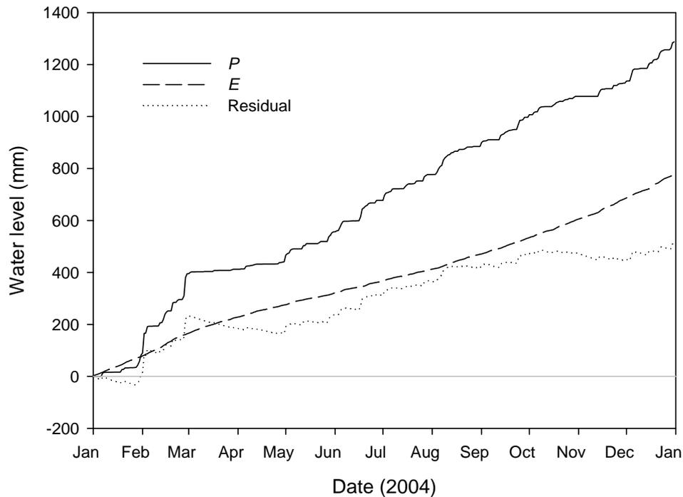
**Figure 24: Annual (2004) cumulative water balance for Opuatia Wetland. Measurements from the EC site. *P* = precipitation and *E* = evaporation.**
