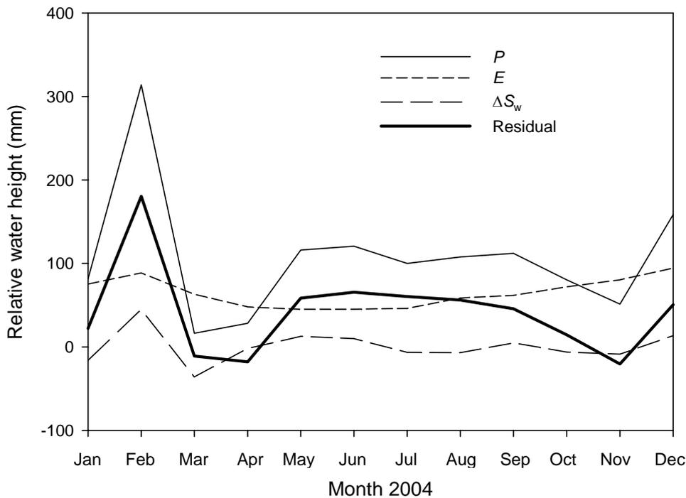
**Figure 25: Monthly water balance for the fen and bog area of Opuatia Wetland.  $P$  = precipitation,  $E$  = evaporation and  $\Delta S_w$  = change in water table storage.**
