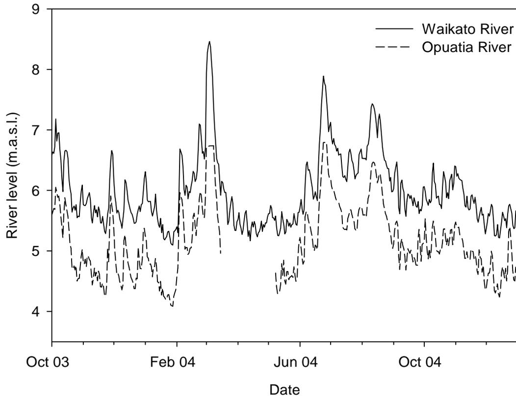
**Figure 26: Waikato River and Opuatia River stage single midnight values from October 2003 to January 2004. The flat tops on the Opuatia River level data occur due to overtopping the instrumentation during flood events.**
