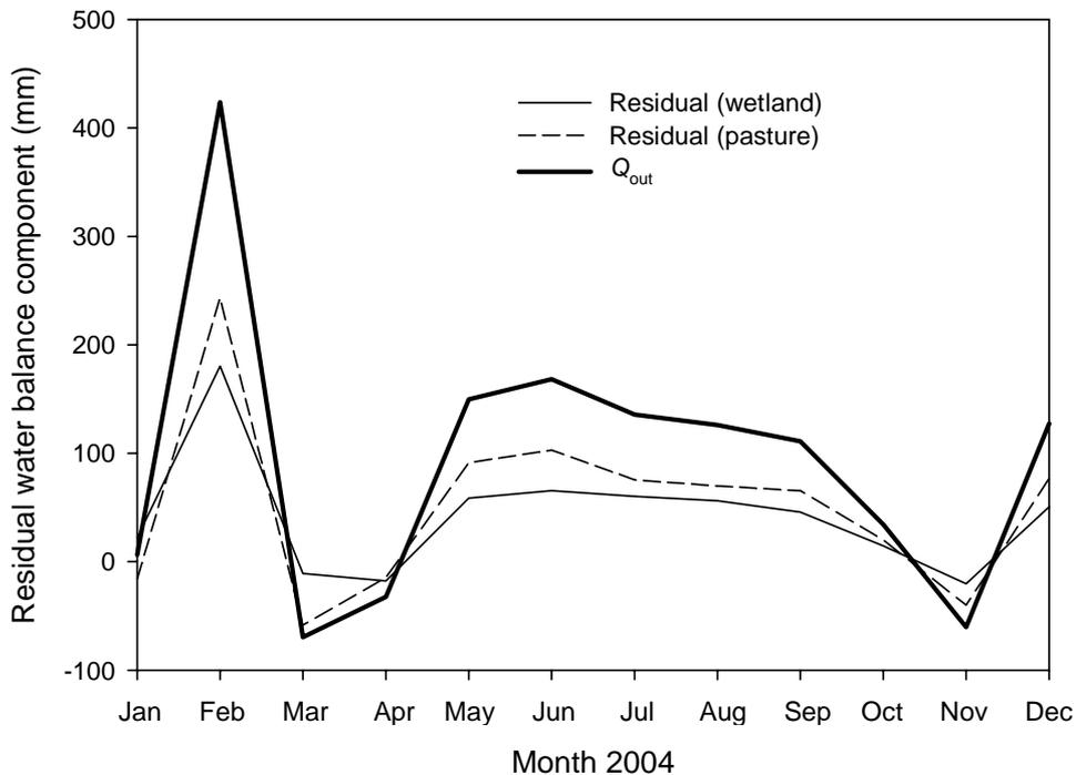
**Figure 23: Monthly residuals taken from the pasture, swamp, fen and bog water balances. The residuals were summed to calculate total discharge ( $Q_{out}$ ) from the wetland. Pasture residual is scaled to represent a depth over the wetland.**
