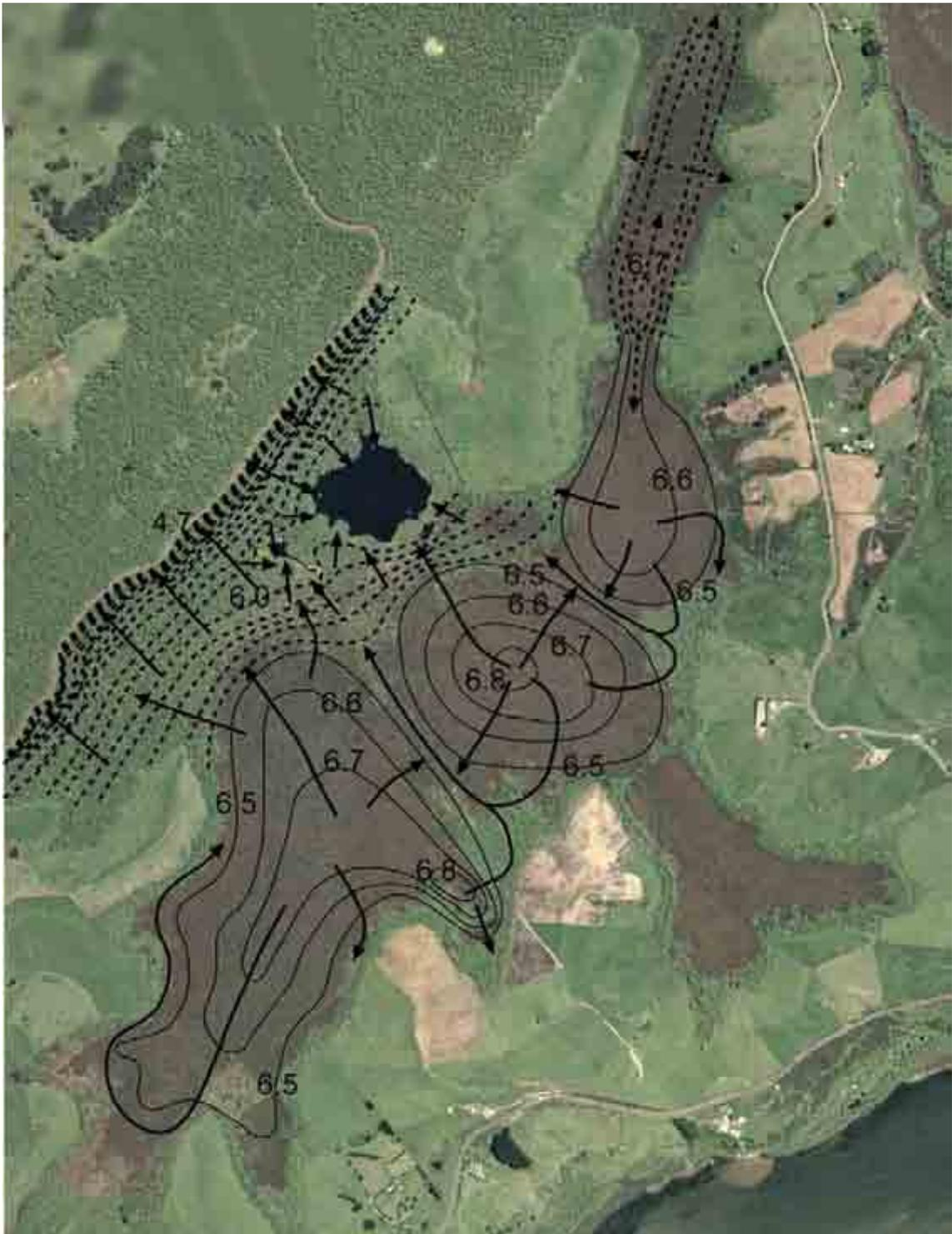
**Figure 18:** Average water level surface contours at intervals of 0.1 metres above sea level and flow directions for 1 December to 1 March 2005. Dashed contours are inferred.
