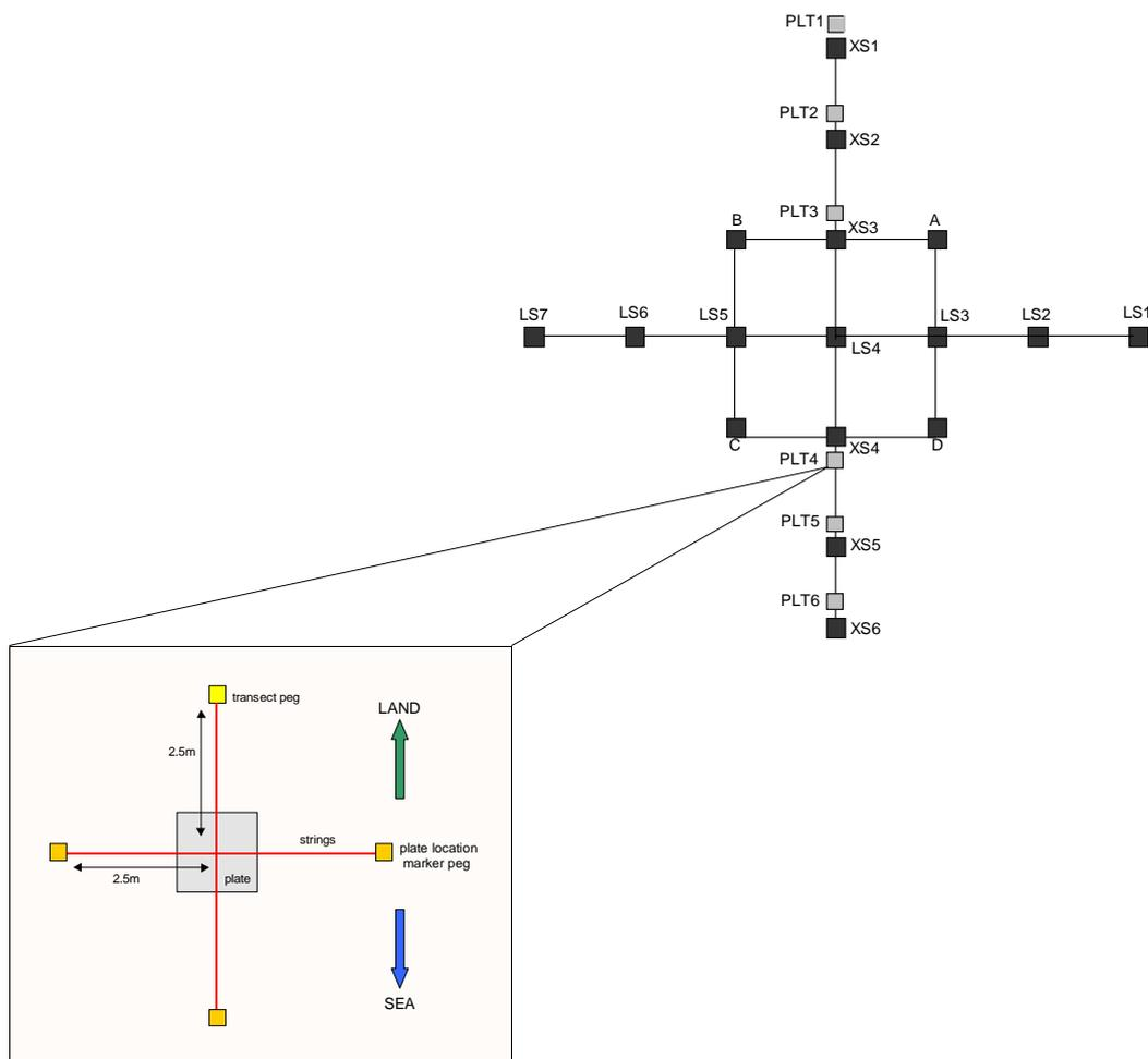
**Figure 4: Diagram illustrating buried plate and locator peg positions.**
