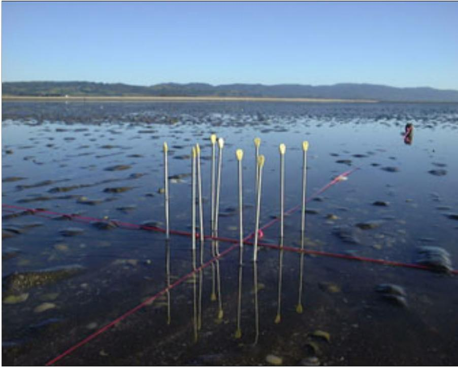
**Figure 5:** Knitting needles were used to measure the depth of sediment over each of the plates at each sampling run. One of the four locator pegs can be seen in the background, and the strings (pink) can be seen in the foreground, crossing over the plate.
