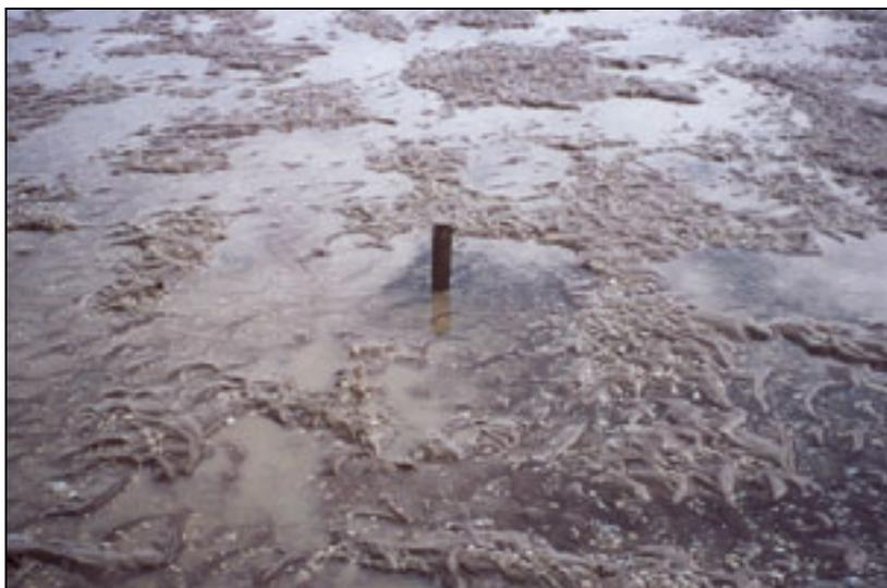
**Figure 3: Wooden post placed to mark the monitoring plot and to measure sediment levels. Localised scour around the posts has created problems with sediment level measurements.**
