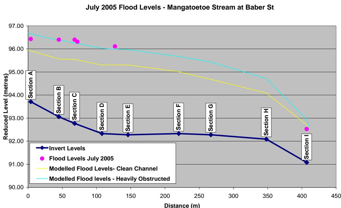
**Figure 2 Observed and modelled water levels for the Mangatoetoe Stream**
