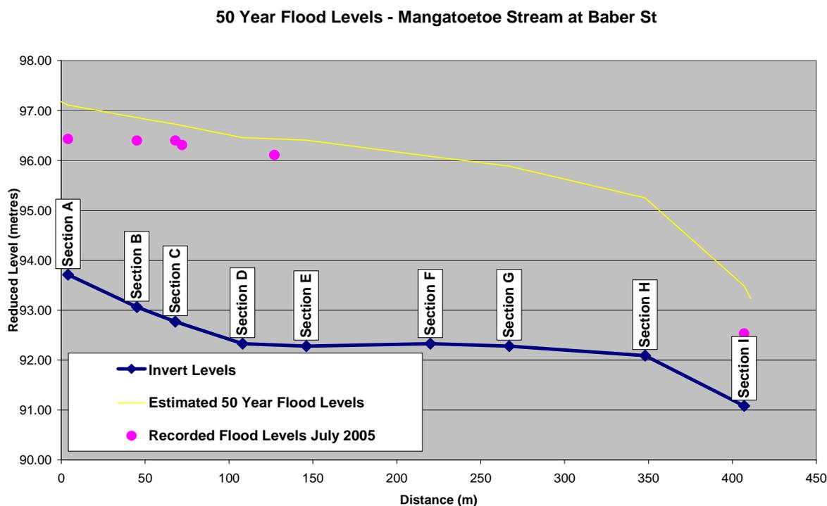
**Figure 4 Modelled 50 year flood levels**
