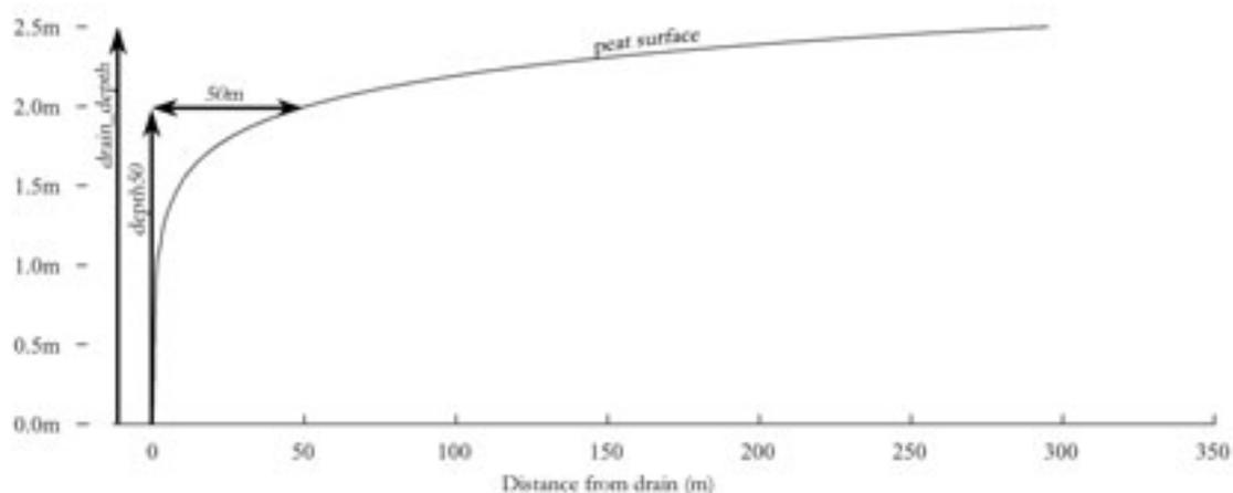
**Figure 19: Illustration of drain depth estimation from a depth measurement made relatively close to the drain.**
