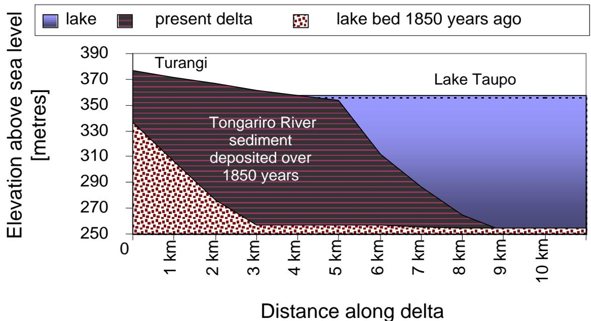
**Figure 3:** Cross-section cut through the Tongariro delta showing alluvial deposition that may have occurred during the last 1850 years.
