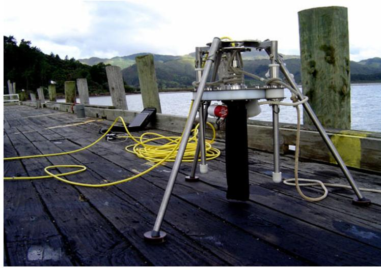
**Fig. 1.** The photograph shows the frame, the imaging cylinder (covered with black neoprene), and the yellow tether of the SPITwo. The imaging cylinder was covered for the purpose of test scans.
