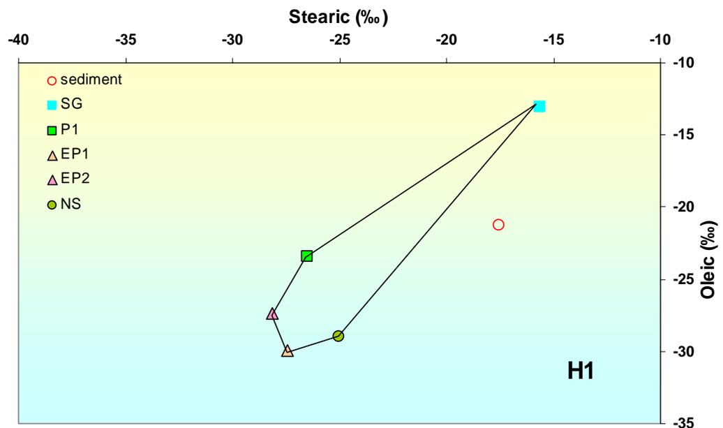
**Figure 4:** Selected sources plotted and connected as a straight line polygon relative to the harbour sediment sample, H1, being tested. While the sample H1 is outside the polygon, it is within the tolerance range of the IsoSource model.
