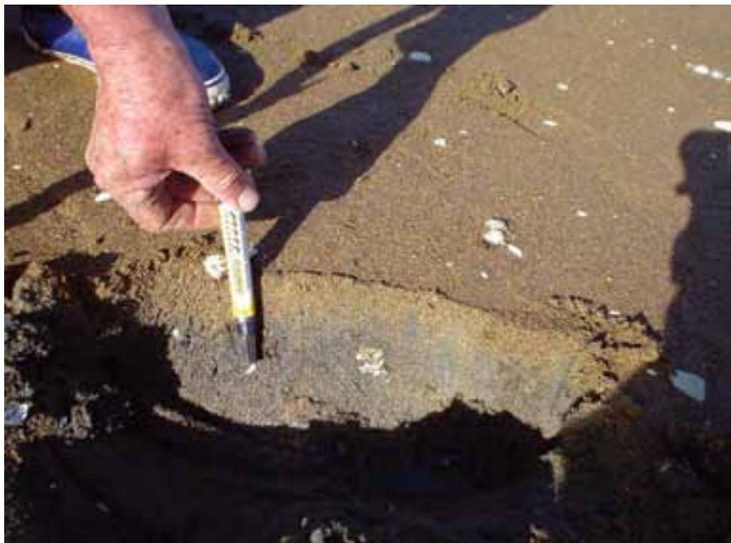
**Photo 7:** A section cut down through the intertidal sandflats at site H3 showing the layer of red-brown bed-load material covering the grey-white sands of the natural sandflats. Shell fragments have been entrained into the bed-load material.
